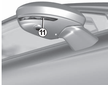
LED side repeaters 11 (depending on vehicle)
