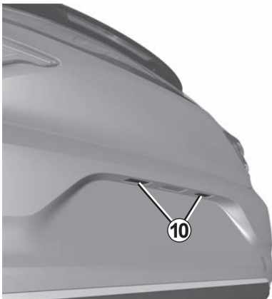
LED number plate lights 10 (depending on vehicle)
