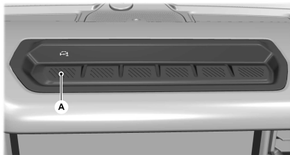
A Stabilizer bar disconnect switch.
