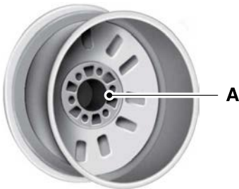
A Hub pilot bore.
