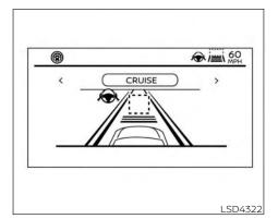
System set display with no vehicle detected ahead (7 inch (18 cm) display) No vehicle detected ahead
