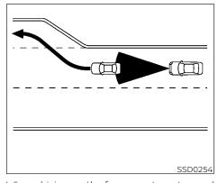
When driving on the freeway at a set speed and approaching a slower traveling vehicle ahead, the ICC system adjusts the speed to maintain the distance, selected by the driver, from the vehicle ahead. If the vehicle ahead changes lanes or exits the freeway. the ICC system accelerates and maintains the speed up to the set speed. Pay attention to the driving operation to maintain control of the vehicle as it accelerates to the set speed.
