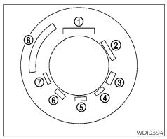
Tire Identification Number (TIN) for safety standard certification. The TIN can be used to identify the tire in case of a recall
