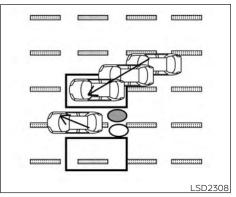
Illustration 6 - Entering from the side **Illustration 6:** If the driver activates the turn signal while another vehicle is in the detection zone, then the system chimes (twice) and the side BSW/RCTA indicator light and the BSW indicator flash.
