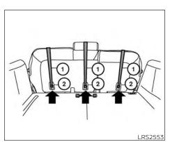
2nd row bench seat (if so equipped) Installing top tether strap
