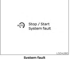
This message is displayed when the Idling Stop System is malfunctioning.
