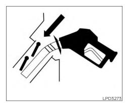
The fuel tank is not equipped with a fuel filler cap. After opening the fuel-filler door, insert the fuel pump nozzle directly into the fuel-filler opening. When the fuel pump nozzle is pulled out, the fuel filler opening will be sealed
