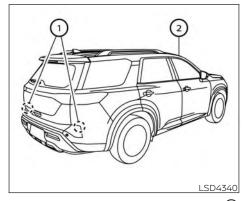
The I-BSI system uses radar sensors (1) installed near the rear bumper to detect other vehicles in an adjacent lane. In addition to the radar sensors, the I-BSI system uses a camera (2) installed behind the windshield to monitor the lane markers of your traveling lane.
