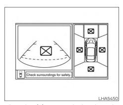
When the "[X]" icon is displayed on the screen, the camera image may be receiving temporary electronic disturbances from surrounding devices. This will not hinder normal driving operation but the system should be inspected if it occurs frequently. It is recommended that you visit a NISSAN dealer for this service
