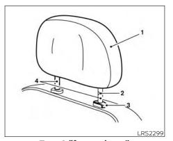
Type A (if so equipped) NON-ADJUSTABLE HEAD
