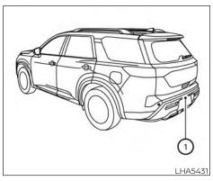
If dirt, rain or snow accumulates on the camera ①, the RearView Monitor may not display objects clearly. Clean the camera by wiping it with a cloth dampened with a diluted mild cleaning agent and then wiping it with a dry cloth.
