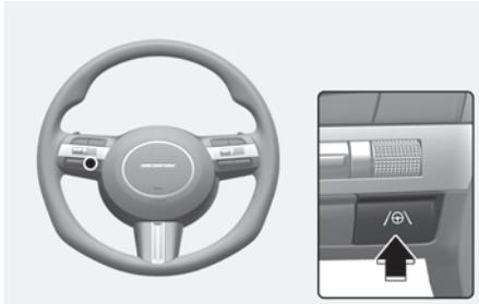
With the engine on, shortly press the Lane Driving Assist button located on the steering wheel to turn on Lane Following Assist. The gray or green (Ω) indicator light will illuminate on the instrument cluster.
