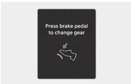
This message appears when the brake pedal is not depressed while shifting the gear.
