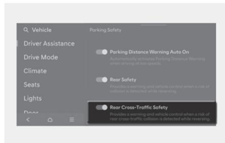
With the engine on, select **Setup > Vehicle > Driver Assistance > Parking Safety > Rear-Cross Traffic Safety** in the infotainment system to turn on Rear Cross-Traffic Collision-Avoidance Assist and deselect to turn off the function.
