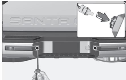
1. Using a flat-blade screwdriver, gently pry the lens cover from the light housing.
