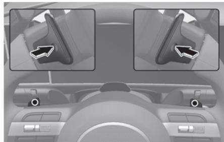
The paddle shifter is available when the gear is in the D (Drive) position.
