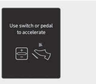
In traffic, your vehicle will stop if the vehicle ahead of you stops. Also, if the vehicle ahead of you starts moving, your vehicle will start as well. In addition, after the vehicle has stopped and a certain time have passed, the '**Use switch or pedal to accelerate**' message will appear on the instrument cluster. Depress the accelerator pedal or operate the + switch, - switch or II $\square$  switch to start driving.
