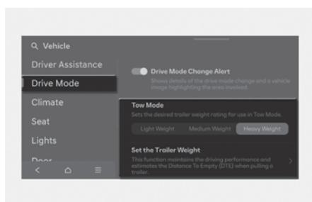
When the gear is in P (Park), select **Setup** > **Vehicle** > **Drive Mode** > **Tow Mode** from the infotainment system to set the weight of trailer to be towed.
