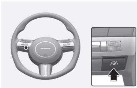
You can turn on and off Lane Keeping Assist (/θ＼) by pressing and holding the Lane Driving Assist (/＼) button while the vehicle is 'ON'.
