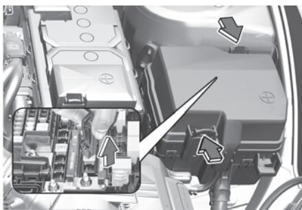
6. Check the removed fuse and replace it if it is blown. To remove or insert the fuse, use the fuse puller in the engine compartment fuse panel.
