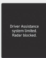
When the rear bumper around the rear corner radar or sensor is covered with foreign material, such as snow or rain, or installing a trailer or carrier, it can reduce the detecting performance and temporarily limit or disable Blind-Spot Collision-Avoidance Assist.
