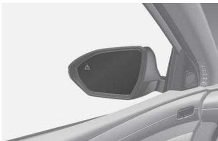
When the vehicle is detected in the rear left and right lanes, to warn the driver a vehicle is detected, the warning light on the side view mirror and Head-Up-Display (if equipped) will illuminate. Vehicle detection operates under following conditions.
