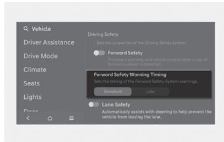
With the Engine Start/Stop button ON, select **Setup > Vehicle > Driver Assistance > Driving Safety > Forward Safety Warning Timing** from the Settings menu to change the initial warning activation time. Warning Timing is set to **Standard** at the factory.
