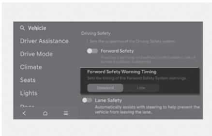
With the vehicle on, select **Setup > Vehicle > Driver Assistance > Driving Safety > Forward Safety Warning Timing** settings menu in the infotainment system to change the initial warning activation time for Forward Collision-Avoidance Assist. The warning time can be set to either **Standard** or **Late**.
