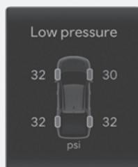
This warning message appears if the tire pressure is low. The corresponding tire on the vehicle is illuminated.
