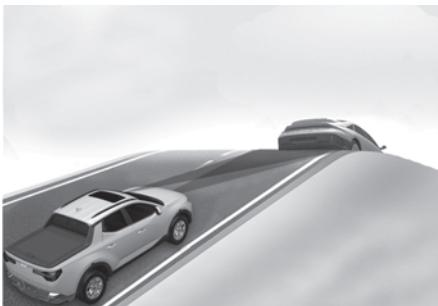
During uphill or downhill driving, the Smart Cruise Control may not detect a moving vehicle in your lane, and cause your vehicle to accelerate to the set speed. Also, vehicle speed will rapidly decrease when the vehicle ahead is detected suddenly.
