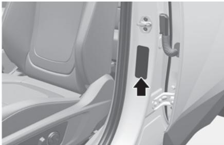
The vehicle certification label attached on the driver's side center pillar gives the vehicle identification number (VIN).
