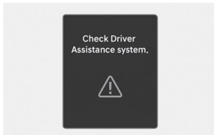
When Intelligent Speed Limit Assist is not working properly, the '**Check Driver Assistance system.**' warning message will appear on the instrument cluster for several seconds, and the master (⚠) warning light and (✉) warning light will illuminate on the instrument cluster. If this occurs, have your vehicle inspected by an authorized HYUNDAI dealer.
