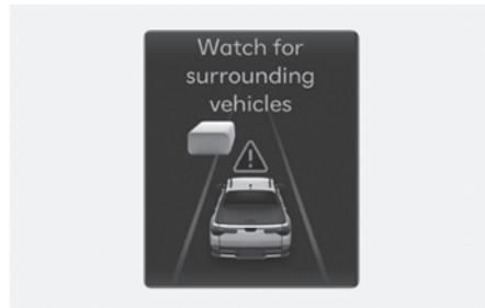
In the following situation, the '**Watch for surrounding vehicles**' warning message will appear on the instrument cluster, and an audible warning will sound and steering wheel will vibrate to warn the driver of road conditions ahead.
