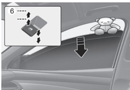
If a window senses any obstacle while it is closing automatically, it stops and lowers approximately 12 in. (30 cm) to allow the object to be cleared.
