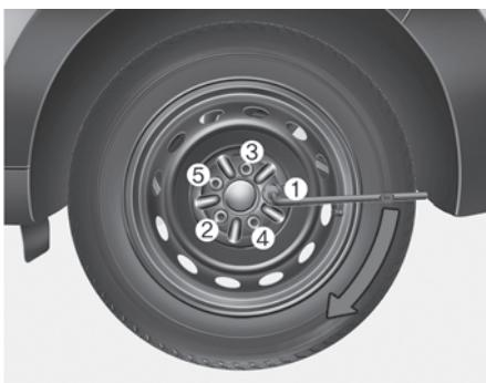
12. Use the wheel lug wrench to tighten the lug nuts in the order shown. Double-check each lug nuts until they are tight. After changing tires, have the vehicle inspected by an authorized HYUNDAI dealer tighten the lug nuts to their proper torque as soon as possible. The lug nut should be tightened to 79-94 lbf. ft (11-13 kgf.m).
