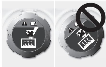
2. Make sure that the tiny protrusions inside the coolant cap is securely interlocked.
