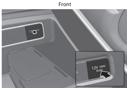
The power outlet is designed to provide power for mobile phones or other devices designed to operate with vehicle electrical systems. The devices should draw less than 12 V, 180 W with the engine running.
