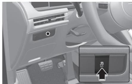
Electronic Stability Control helps stabilize the vehicle during cornering maneuvers. ESC checks where you are steering and where the vehicle is actually going. ESC applies braking pressure to any one of the vehicle's brakes and intervenes in the engine management system to assist the driver with keeping the vehicle on the intended path. It is not a substitute for safe driving practices. Always adjust your speed and driving to the road conditions.
