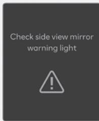
When the side view mirror warning light is not working properly, the '**Check side view mirror warning light**' warning message appears on the instrument cluster for several seconds, and the master (⚠) warning light illuminates on the instrument cluster. If this occurs, have your vehicle inspected by an authorized HYUNDAI dealer.
