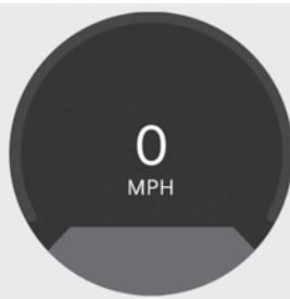
The speedometer indicates the speed of the vehicle and is calibrated in miles per hour (MPH) and/or kilometers per hour (km/h).
