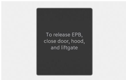
If the hood, liftgate, doors are open, and you try to drive with EPB applied, a warning sounds and a message appears.
