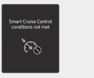
If the Driving Assist button, + switch, - switch or II $\square$  switch is operated when Smart Cruise Control operating conditions are not satisfied, the '**Smart Cruise Ctrl. conditions not met**' will appear on the instrument cluster, and an audible warning will sound.
