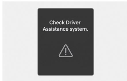
When Forward Collision-Avoidance Assist is not working properly, the '**Check Driver Assistance system.**' warning message will appear, and the (Δ) or (✖) warning lights will illuminate on the instrument cluster. Have your vehicle inspected by an authorized HYUNDAI dealer.
