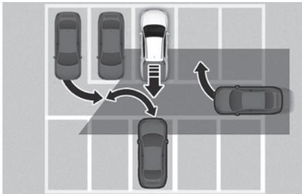
Rear Cross-Traffic Collision-Avoidance Assist may detect vehicles which are parking or pulling out near your vehicle (for example, a vehicle leaving beside your vehicle, a vehicle parking or pulling out in the rear area, a vehicle approaching your vehicle making a turn, etc.). If this occurs, the function may unnecessarily warn the driver and control the brake.
