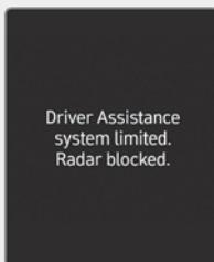
When the front windshield where the front view camera is located, front radar cover, bumper (if equipped) or sensor is covered with foreign material, such as snow or rain, it can reduce the detecting performance and temporarily limit or disable Forward Collision-Avoidance Assist.
