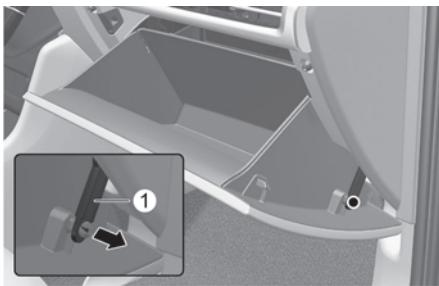
2. Push in both sides of the glove box to release the glove box stopper pins and allow the glove box to hang open.
