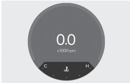
The engine coolant temperature gauge indicates the temperature of the engine coolant when the Engine Start/Stop button is in the ON position.
