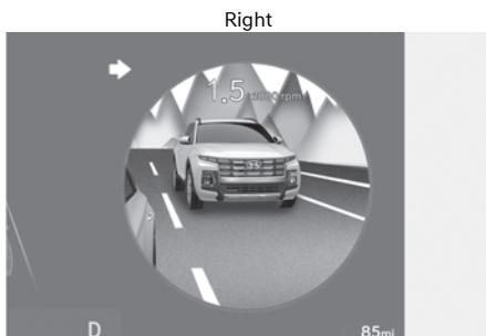
Blind-Spot View Monitor uses the wide-side view cameras to display the rear blind spot areas of your vehicle on the instrument cluster when the turn signal is turned on to help with safe lane changes.
