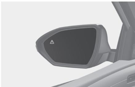
Your vehicle is equipped with both left-hand and right-hand side view mirrors. The mirrors can be adjusted remotely with the mirror adjustment control switch. Adjust the side view mirrors to your desired position before driving.
