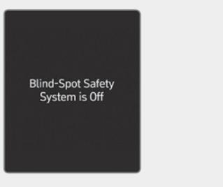
When the vehicle is restarted with Blind-Spot Collision-Avoidance Assist off, the **'Blind-Spot Safety System is Off'** message will appear on the instrument cluster.
