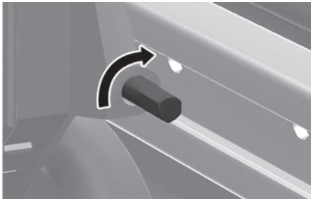
3. Rotate the pinion clockwise to increase the tension for faster opening.
