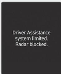
When the rear bumper around the rear corner radar or sensor is covered with foreign material, such as snow or rain, or installing a trailer or carrier, it can reduce the detecting performance and temporarily limit or disable Safe Exit Warning.
