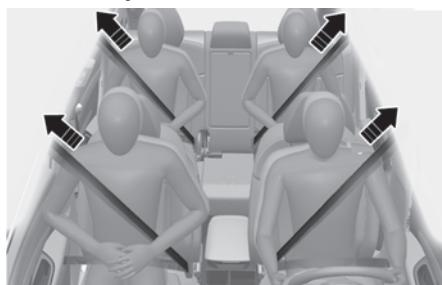
Your vehicle is equipped with driver's and front passenger's and rear passengers pretensioner seat belts (retractor pretensioner). The pretensioner makes sure the seat belts fit tightly against your body in certain frontal or side collision(s). The pretensioner seat belts may be activated in some crashes where the frontal or side collision(s) is severe enough, together with the airbags.
