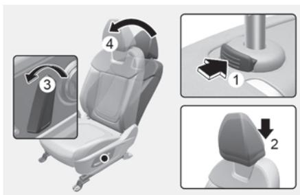
To reinstall the head restraint:
