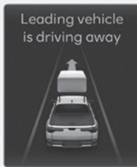
When a detected vehicle in front departs from a stop, Leading Vehicle Departure Alert will inform the driver by displaying the '**Leading vehicle is driving away**' message on the instrument cluster and an audible warning will sound.
