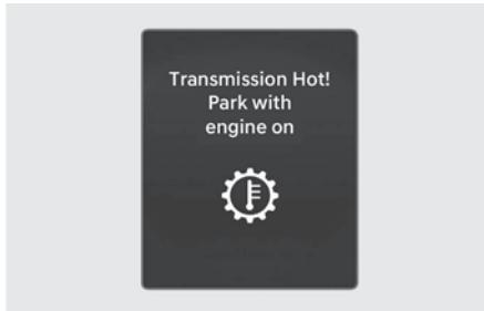
Repeated sudden acceleration and quick start may overheat the transmission. If the transmission is overheated, the self protection mode alarms the driver with an audible sound warning message.
