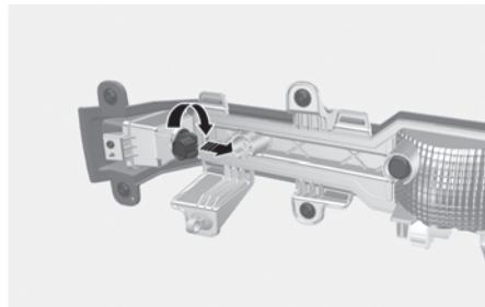
1. Remove the bulb by rotating to counterclockwise and pulling it straight out.
