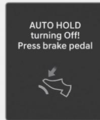
When the conversion from Auto Hold to EPB is not working properly, a warning sounds and a message appears.
