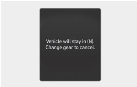
This message appears when pushing the **OK** button on the steering wheel after the message '**Press and hold the OK button on the steering wheel to stay in Neutral**' appears on the cluster display. The gear stays in N (Neutral) position after turning off the engine.
