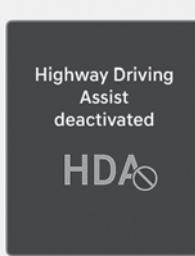
If the driver still does not have their hands on the steering wheel after the hands-off warning, '**Highway Driving Assist deactivated**' warning message will appear and Highway Driving Assist will be automatically canceled.
