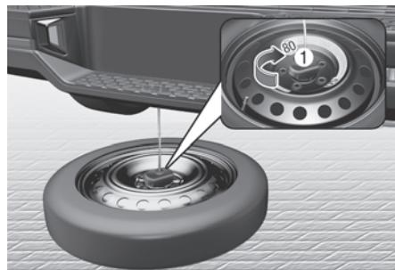
1. Lay the tire on the ground with the valve stem facing up.
