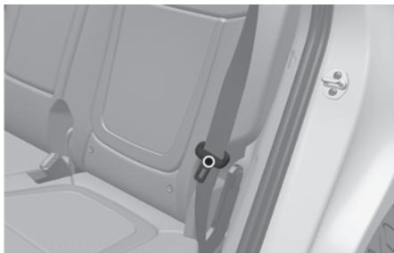
Routing the seat belt webbing through the rear seat belt guides will help keep the belts from being trapped behind or under the seats.
