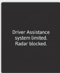
When the rear bumper around the rear-side radar or sensor is covered with foreign material, such as snow or rain, or installing a trailer or carrier, it can reduce the detecting performance and temporarily limit or disable Rear Cross-Traffic Collision-Avoidance Assist.
