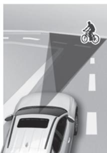
Forward Collision-Avoidance Assist may not detect other vehicles, powered two-wheelers, pedestrians or cyclists in front of you when driving on curved roads adversely affecting the performance of the sensors. This may result in no warning, braking assist when necessary.
