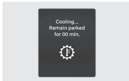
If you move the vehicle to a safe location and shift the gear to P (Park) with the engine running, the above warning message appears.
