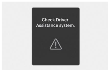
When Blind-Spot Collision-Avoidance Assist is not working properly, the '**Check Driver Assistance system.**' warning message will appear on the instrument cluster for several seconds, and the master (△) warning light will appear on the instrument cluster. If this occurs, have your vehicle inspected by an authorized HYUNDAI dealer.
