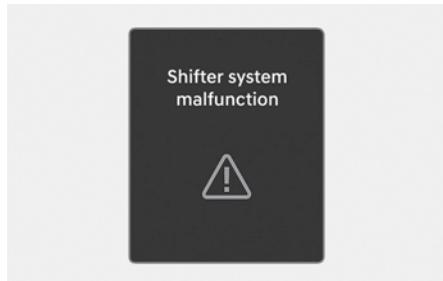
This message appears when the transmission or the shift lever does not properly operate in the P (Park) position.
