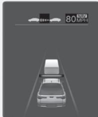
If you want to speed up temporarily without altering the set speed while Smart Cruise Control is operating, depress the accelerator pedal. While the accelerator pedal is depressed, the set speed, distance level and target distance will blink on the instrument cluster.
