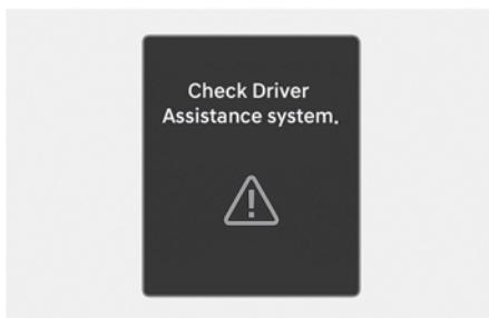
When Forward Collision-Avoidance Assist is not working properly, the '**Check Driver Assistance system.**' warning message will appear, and the (⚠) or (✖) warning lights will illuminate on the cluster display. Have the vehicle inspected by an authorized HYUNDAI dealer.
