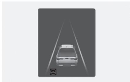
If the vehicle ahead and/or both lane markings are detected and your vehicle speed is below 110 mph (180 km/h), the green (Ω) indicator light appears on the cluster, and Lane Following Assist helps center the vehicle in the lane by assisting the steering wheel.
