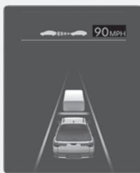
When driving at a speed higher than the displayed speed limit, the speed limit is displayed in red.
