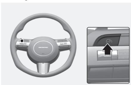
Press the Driving Assist button to turn Cruise Control off. The Cruise (C<sub>CRUISE</sub>) indicator will go off.
