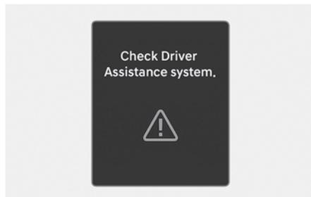
When Safe Exit Warning is not working properly, the '**Check Driver Assistance system.**' warning message will appear on the instrument cluster for several seconds, and the master warning light (⚠) will appear on the instrument cluster. If this occurs, have your vehicle inspected by an authorized HYUNDAI dealer.
