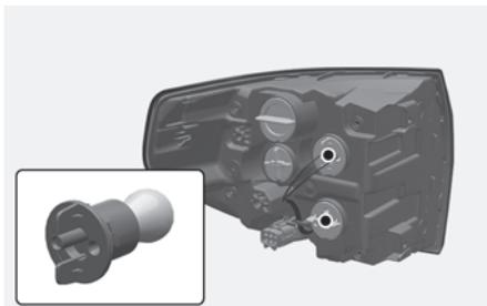
6. Remove the bulb from the socket by pressing it in and rotating it counterclockwise until the tabs on the bulb align with the slots in the socket. Pull the bulb out of the socket.
