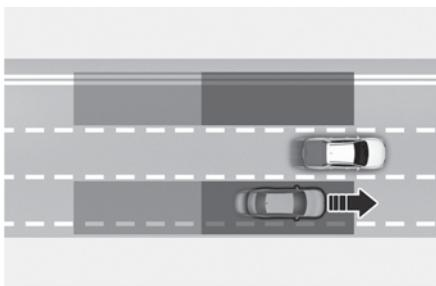
Blind-Spot Collision-Avoidance Assist helps detect and informs the driver that a vehicle is in the blind spot.
