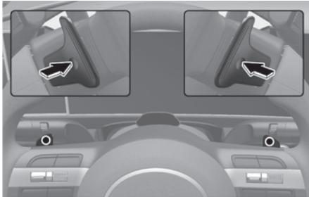
The paddle shifter is available when the shift lever is in the D (Drive) position or the manual shift mode.
