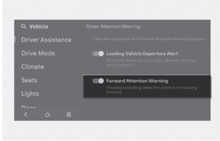
If **Forward Attention Warning** is enabled, the function warns the driver when the driver's gaze is not focused on the road.
