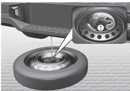
4. After the spare tire reaches the ground, continue to turn the wrench counterclockwise, and draw the spare tire outside. Never rotate the wrench excessively, otherwise the spare tire carrier may be damaged.
