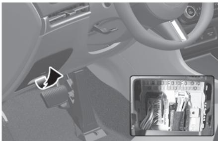
4. Refer to the label on the inside of the fuse panel cover to locate the suspected fuse location.
