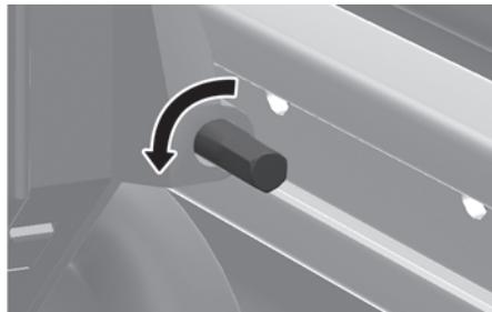
4. Rotate the pinion counterclockwise to decrease the tension for slower opening.
