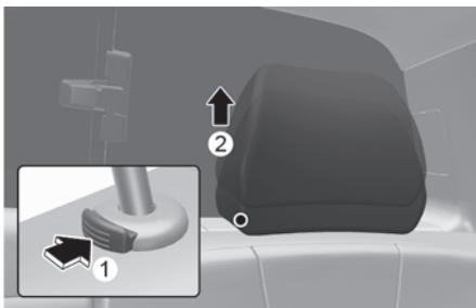
To remove the head restraint:
