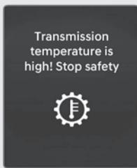
Repeated stop-and-go launches on steep grades, sudden take off or acceleration, or other harsh driving conditions may increase the clutch and transmission temperature.
