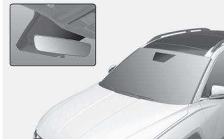
The Auto defogging reduces the possibility of fogging up the inside of the windshield by automatically sensing the moisture on inside the windshield. The auto defogging system operates when the heater or air conditioning is on.
