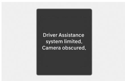
When the front windshield where the front view camera is located or the sensor is covered with foreign material, such as snow or rain, it can reduce the detecting performance and temporarily limit or disable Forward Collision-Avoidance Assist.
