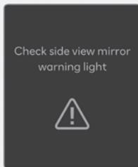
When the side view mirror warning light is not working properly, the '**Check side view mirror warning light**' warning message will appear on the instrument cluster for several seconds, and the master warning light (⚠) will appear on the instrument cluster. If this occurs, have your vehicle inspected by an authorized HYUNDAI dealer.
