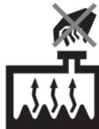
Never remove the engine coolant cap or the drain plug while the engine and radiator are hot.
