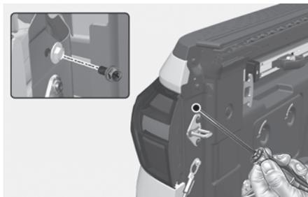
4. Remove the rear combination light assembly from the body of the vehicle.
