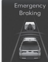
To warn the driver that emergency braking will be assisted, Forward Safety warning light (✉) blinking, the '**Emergency Braking**' warning message will appear on the cluster, an audible warning will sound, and the steering wheel will vibrate.
