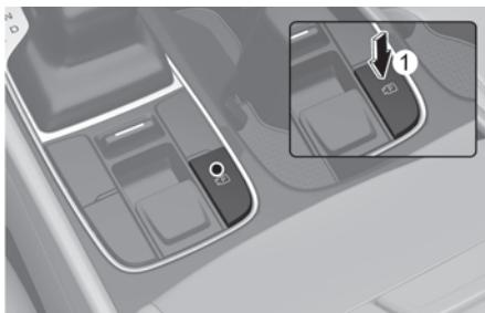
Press the Parking/View button (1) while the gear is in P (Park), D (Drive) or N (Neutral) to turn on the Rear View Monitor.
