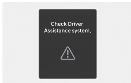
When Rear Cross-Traffic Collision-Avoidance Assist is not working properly, the '**Check Driver Assistance system.**' warning message appears on the instrument cluster for several seconds, and the master (Δ) warning light illuminates on the instrument cluster. If this occur, have vehicle inspected by an authorized HYUNDAI dealer.
