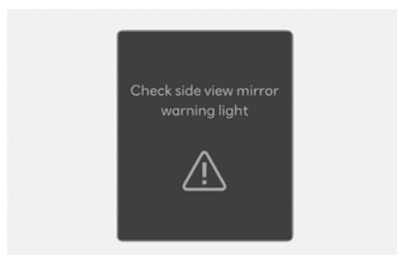
When the side view mirror warning light is not working properly, the '**Check side view mirror warning light**' warning message will appear on the instrument cluster for several seconds, and the master (△) warning light will illuminate on the instrument cluster. If this occurs, have your vehicle inspected by an authorized HYUNDAI dealer.
