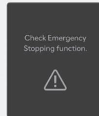
When Emergency Stop is not working properly, the '**Check Emergency Stopping function.**' warning message appears, and the master (△) warning light illuminates on the instrument cluster. If this occurs, have your vehicle inspected by an authorized HYUNDAI dealer.
