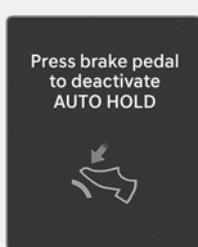
If you did not apply the brake pedal when you release Auto Hold by pressing the AUTO HOLD switch, a warning sounds and a message appears.
