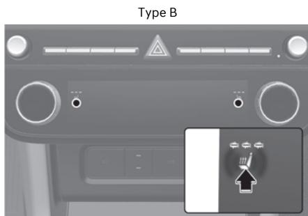
While the engine is running, press the button to warm the driver's seat or front passenger's seat.
