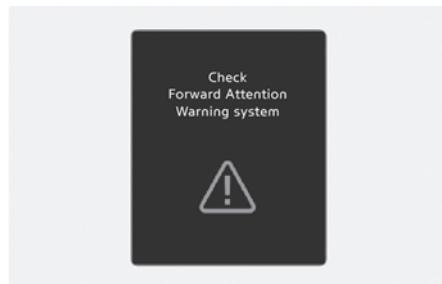
When Forward Attention Warning is not working properly, the '**Check Forward Attention Warning system**' warning message will appear on the cluster. If this occurs, have the vehicle inspected by an authorized HYUNDAI dealer.
