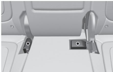
The rear seat belt buckles can be stowed in the pocket between the rear seatback and cushion when not in use.
