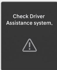
When Highway Driving Assist is not working properly, the '**Check Driver Assistance system.**' warning message and yellow Lane Keeping Assist (/
