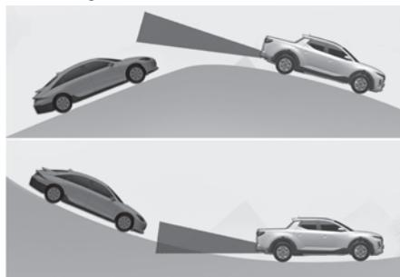
Blind-Spot Collision-Avoidance Assist may not operate properly when driving on a slope. The function may not detect the vehicle in the next lane or may incorrectly detect the ground or structure. Always pay attention to road and driving conditions while driving.
