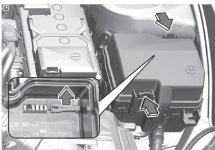
6. Check the removed fuse and replace it if it is blown. Spare fuses are provided in the instrument panel fuse panels (or in the engine compartment fuse panel).
