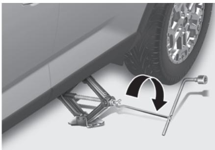
8. Insert the jack handle and wheel lug wrench into the jack and turn it clockwise, raising the vehicle until the tire clears the ground. Make sure the vehicle is stable on the jack.
