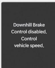
If Downhill Brake Control is not working properly, this warning message appears on the cluster display and you may hear a warning sound. If this occurs, control the vehicle speed by depressing the brake pedal.
