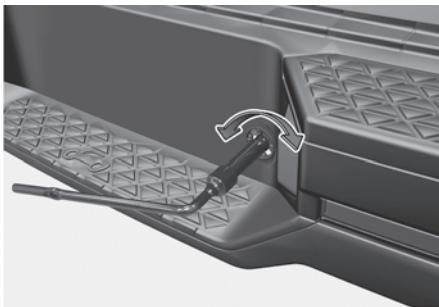
3. Use the wheel nut wrench to loosen the bolt enough to lower the spare tire. Turn the wrench counterclockwise until the spare tire reaches the ground.
