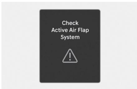
The active air flap system may not operate normally if the air flap is temporarily opened due to foreign factors or if the controller is contaminated by snow or rain, etc.
