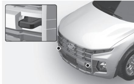
In the event of emergency off-road recovery and to minimize the risk of damaging the vehicle, it is recommended to use both recovery hooks.
