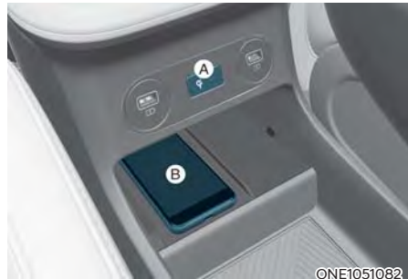
[A] : Indicator light, [B] : Charging pad
