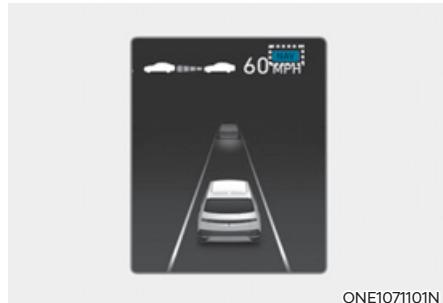
If temporary deceleration is required in the standby state and Navigation-based Smart Cruise Control is operating, the green **NAV** symbol will illuminate on the cluster.
