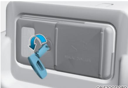
2. Use the smart key to unlock the power outlet cover.
