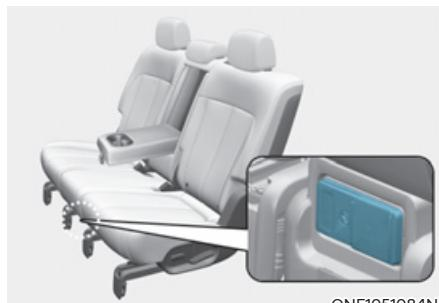
1. Connect to the power outlet located in bottom of the rear seat with the Vehicle Stop/Start button in the ON position.
