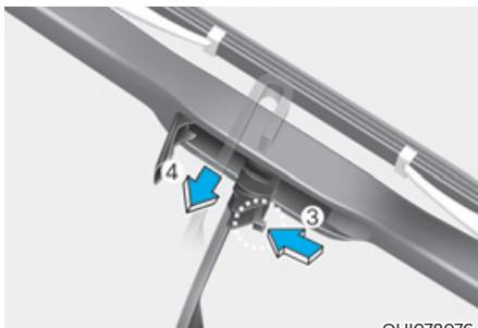
2. Press the clip (3). Then push the blade forward through the wiper arm to disassemble it (4).
