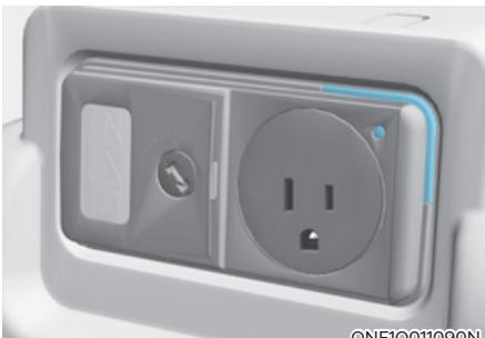
3. Check the operation status through the front indicator of the power outlet.
