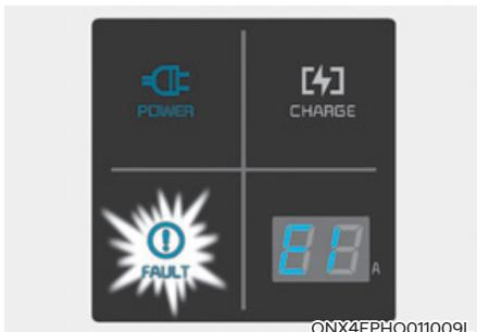
Plugged into vehicle (POWER Green ON, FAULT Red Blink)
