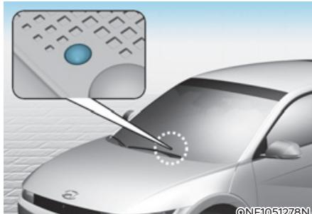
The high voltage indicator is located on top of the crash pad.
