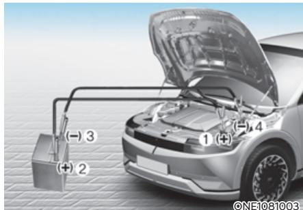
7. Connect the jumper cables in the exact sequence shown in the illustration. First connect one jumper cable to the red, positive (+) jumper terminal of your vehicle (1).
