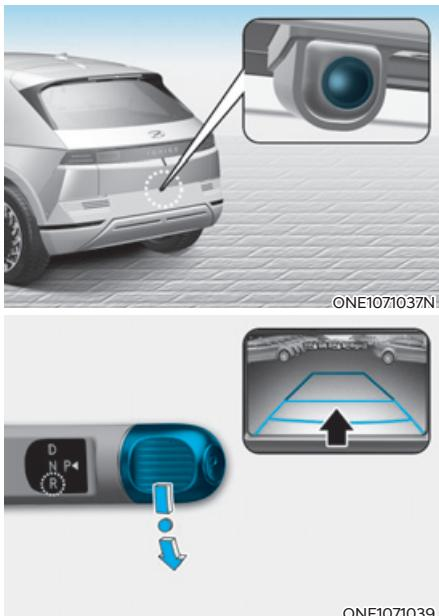
Rear View Monitor shows the area behind the vehicle to assist you when parking or backing up.
