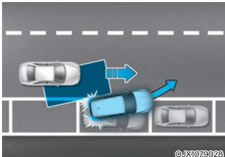
When you are driving forward out of a parking space, if Blind-Spot Collision-Avoidance Assist judges that there is a collision risk with an approaching vehicle in the blind spot, it helps avoid collision by applying the brake.
