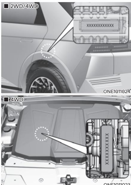
The motor numbers can be checked at the bottom of the vehicle.
