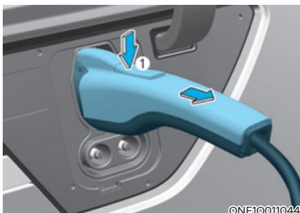
2. Hold the charging connector handle and pull it out.
