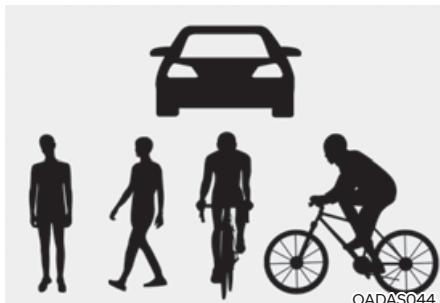
The illustration above shows the image the front view camera and front radar is capable of detecting as a vehicle, pedestrian and cyclist.
