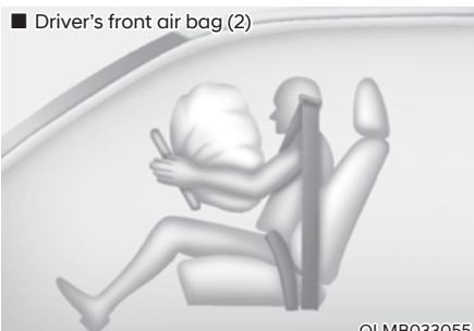
Upon deployment, tear seam molded directly into the pad cover will separate under pressure from the expansion of the air bags. Further opening of the covers allows full inflation of the air bags.
