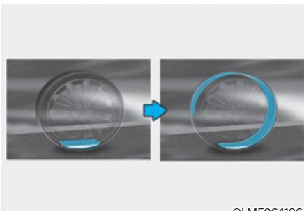
9. Immediately drive approximately 4~6 miles (7~10 km or, about 10min) to evenly distribute the sealant in the tire.
