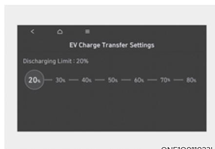
If the vehicle reaches to the limit, it automatically cut supply of electricity.
