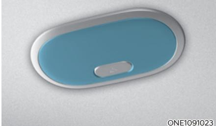
■ Rear seat room lamp (without vision roof/solar roof)
