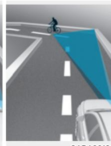
**Forward Collision-Avoidance Assist** may not detect other vehicles, pedestrians or cyclists in front of you while driving on curved roads adversely affecting the performance of the sensors. This may result in no warning, braking assist or steering assist (if equipped) when necessary.
