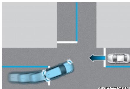
Junction Turning function helps avoid a collision with an oncoming vehicle in an adjacent lane when turning left at a crossroad with the turn signal on by applying emergency braking.
