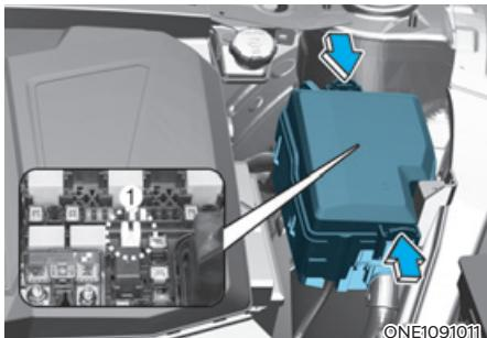
5. Pull the suspected fuse straight out. Use the removal tool (1) provided in the motor compartment fuses panel cover.
