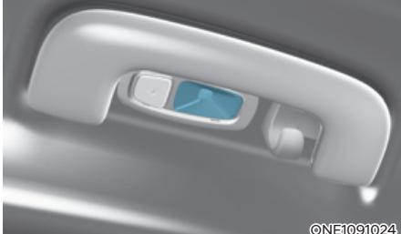
■ Rear seat personal lamp (with vision roof/solar roof)
