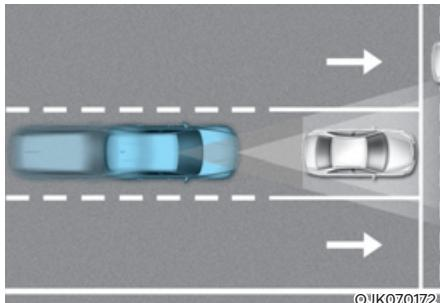
Forward Collision-Avoidance Assist is designed to help detect and monitor the vehicle ahead or help detect a pedestrian or cyclist in the roadway and warn the driver that a collision is imminent with a warning message and an audible warning, apply emergency braking.
