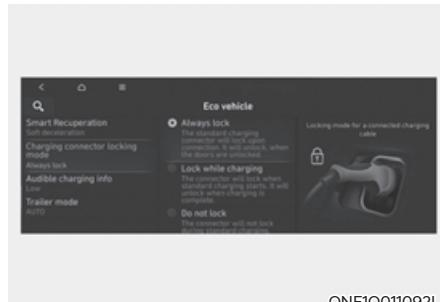
You may select when the charging connector can be locked and unlocked in the charging inlet.
