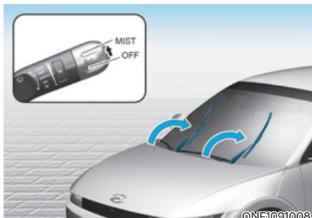
Within 20 seconds of turning off the vehicle, lift up and hold the wiper lever to the MIST position for about 2 seconds until the wipers move to the top wipe position.
