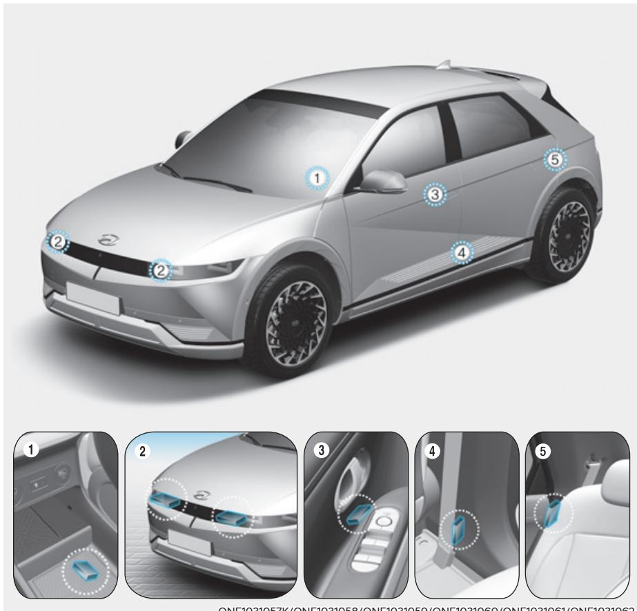
1. SRS control module / Rollover sensor
