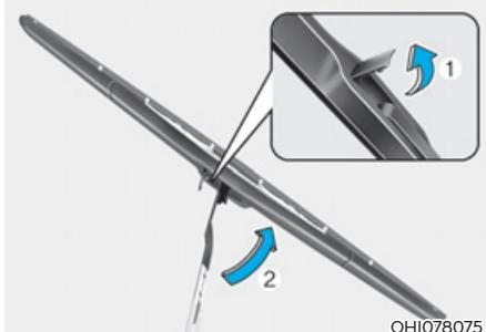
1. Lift up the wiper blade clip (1). Then lift up the wiper blade.
