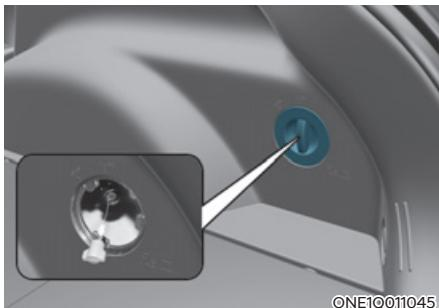
If the charging connector does not disconnect from the charging inlet due to battery discharge and failure of electric wires, open the liftgate and slightly pull the emergency cable in the cargo area. The charging connector will be disconnected from the charging inlet.
