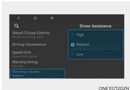
With the vehicle on, select 'Driver Assistance → Warning Volume' from the Settings menu to change the Warning Volume to 'High', 'Medium' or 'Low' for Reverse Parking Distance Warning.
