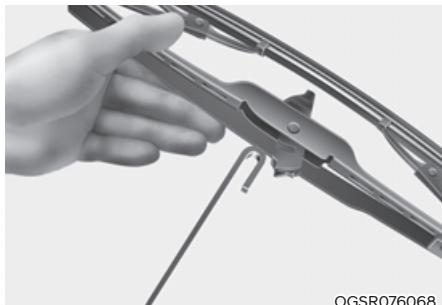
3. Remove the wiper blade from the wiper arm.
