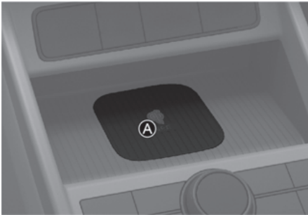
[A] Vehicle authentication pad (Wireless charging pad)
