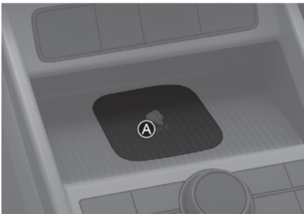
[A] Vehicle authentication pad (Wireless charging pad)
