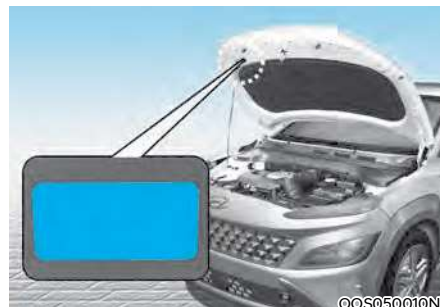
Air Conditioning refrigerant label
