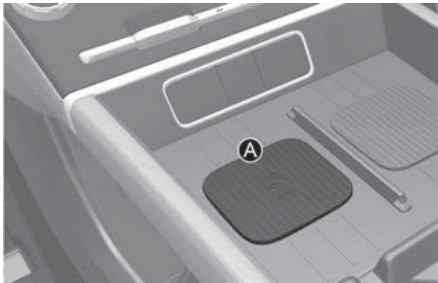
[A] Vehicle authentication pad (wireless charging pad)
