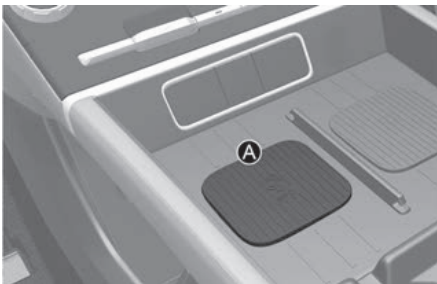
[A] Vehicle authentication pad (Wireless charging pad)
