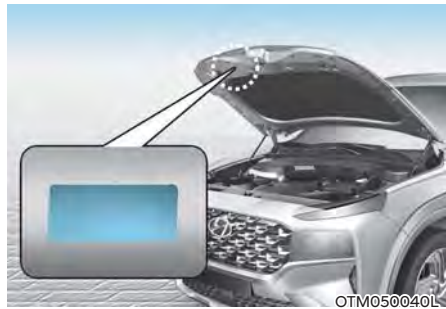
Air Conditioning refrigerant label
