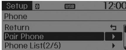
Bluetooth® Wireless Technology devices can be paired with the audio system.
