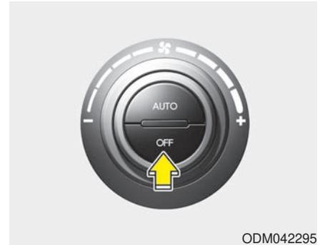
Push the OFF button to turn off the air climate control system. However, you can still operate the mode and air intake buttons as long as the ignition switch is in the ON position.
