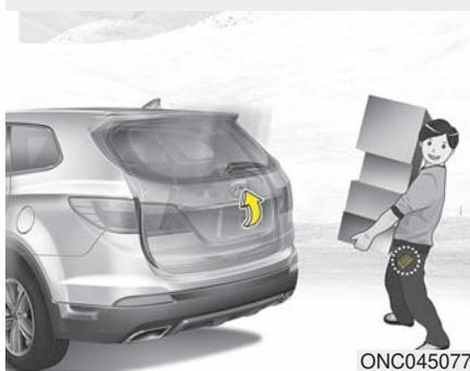
On the vehicle equipped with a smart key, the liftgate (tailgate) can be opened with no-touch activation using the Smart Liftgate (Smart Tailgate) system.
