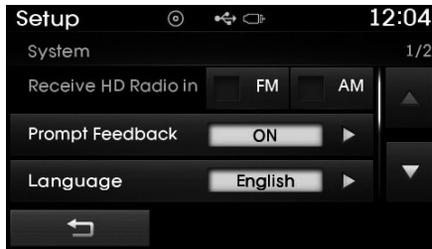
This feature is used to set whether to receive FM/AM HD Radio™ broadcasts.
