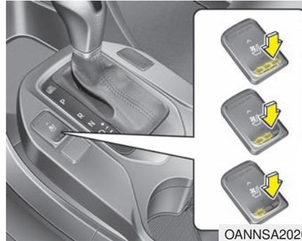
The air ventilation seat is provided to cool the front seats during hot weather by blowing air through small vent holes on the surface of the seats. While the engine is running, press the cooling portion (blue color) of the switch to cool the driver's seat or the front passenger's seat.
