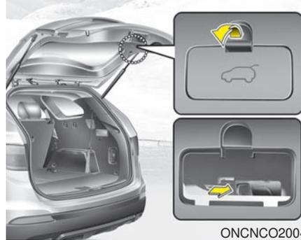
Your vehicle is equipped with the emergency liftgate (tailgate) safety release lever located on the bottom of the liftgate (tailgate). When someone is inadvertently locked in the luggage compartment, the liftgate (tailgate) can be opened by doing as follows:
