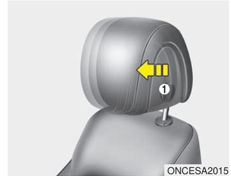
The headrest may be adjusted forward to 4 different positions by pulling the headrest forward to the desired detent. To adjust the headrest to backwards position, press and hold the release button (1), and adjust position of the headrest. Adjust the headrest so that it properly supports the head and neck.
