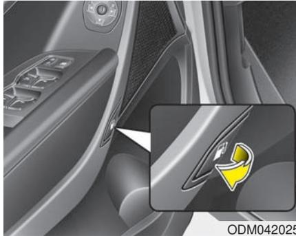
The fuel filler lid must be opened from inside the vehicle by pulling the fuel filler lid opener lever located on the driver's door.
