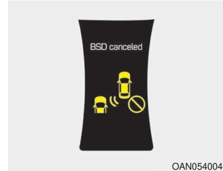
The message will appear to notify the driver if there are foreign substances on the rear bumper. The light on the switch and the system will turn off automatically.
