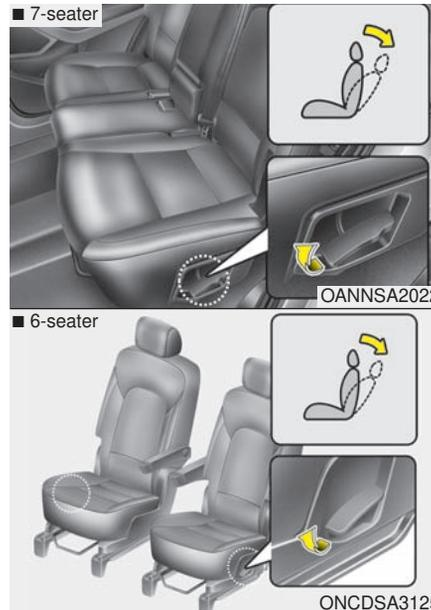
3. Release the lever and make sure the seatback is locked in place. (The lever **MUST** return to its original position for the seatback to lock.)
