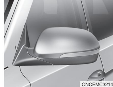
To fold outside rearview mirror, grasp the housing of mirror and then fold it toward the rear of the vehicle.
