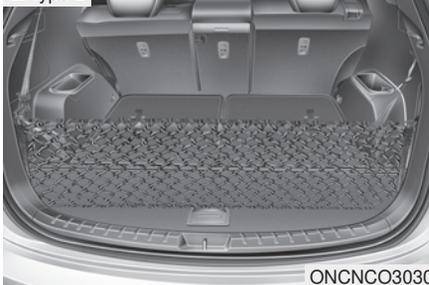
To keep items from shifting in the cargo area, you can use the four holders located in the cargo area to attach the luggage net.
