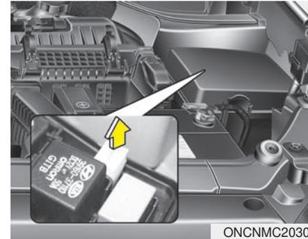
3. Pull the suspected fuse straight out. Use the removal tool provided in the engine compartment fuse panel.
