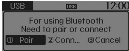
If *Bluetooth*® Wireless Technology devices are paired but none are currently connected, pressing the **PHONE** key or the
