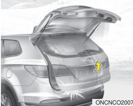
During power opening and closing if the power liftgate (power tailgate) is blocked by an object or part of the body, the power liftgate (power tailgate) will detect the resistance.
