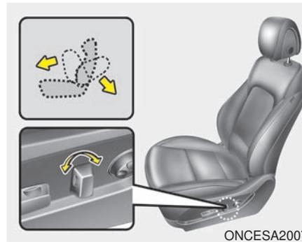
1. Push the control switch forward or backward to move the seatback to the desired angle.
