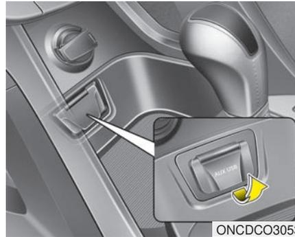
If your vehicle has an aux and/or USB(universal serial bus) port or iPod® port, you can use an aux port to connect audio devices and a USB port to plug in a USB and also in an iPod®.
