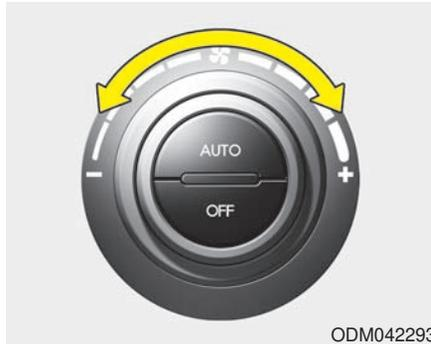
The fan speed can be set to the desired speed by turning the fan speed control knob.
