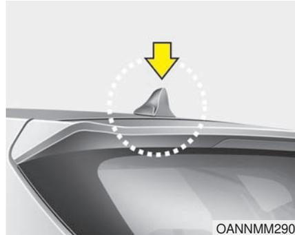
Your vehicle uses a roof antenna to receive both AM and FM broadcast signals.
