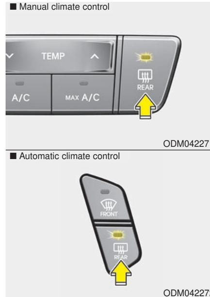
The defroster heats the window to remove frost, fog and thin ice from the rear window, while the engine is running.
