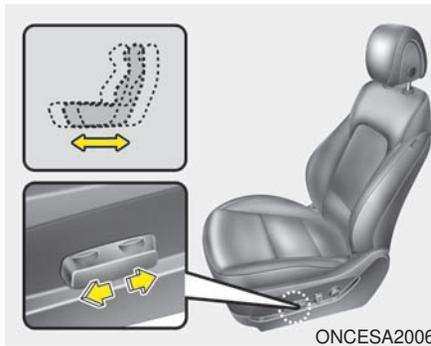
1. Push the control switch forward or backward to move the seat to the desired position.
