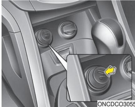
For the cigarette lighter to work, the ignition switch must be in the ACC position or the ON position.
