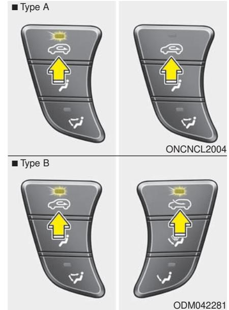
This is used to select outside (fresh) air position or recirculated air position.
