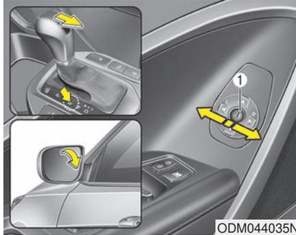
When you shift the shift lever to the R (Reverse) position, the outside rearview mirror(s) will move downward to aid reverse parking. According to the position of the outside rearview mirror control switch (1), the outside rearview mirror(s) will operate as follows:
