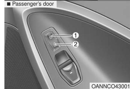
Operate by depressing the central door lock switch.
