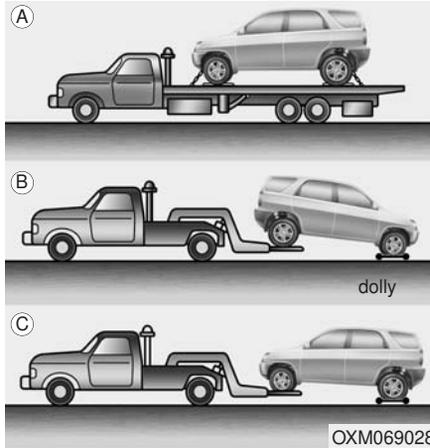
If emergency towing is necessary, we recommend having it done by an authorized HYUNDAI dealer or a commercial tow-truck service. Proper lifting and towing procedures are necessary to prevent damage to the vehicle. The use of wheel dollies or flatbed is recommended.
