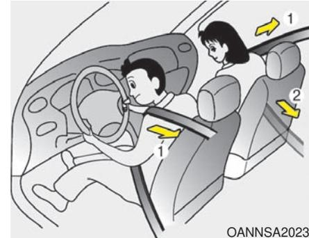
Your vehicle is equipped with pre-tensioner seatbelts in the front seating positions (driver side with retractor pre-tensioner, passenger side with retractor and EFD (Emergency Fastening Device)).
