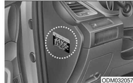
Air bag warning labels, some required by the U.S. National Highway Traffic Safety Administration (NHTSA), are attached to alert the driver and passengers of potential risks of the air bag system.
