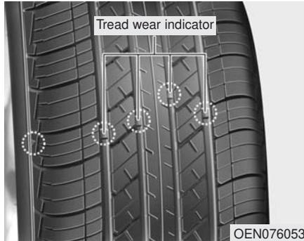
If the tire is worn evenly, a tread wear indicator will appear as a solid band across the tread. This shows there is less than 1/16 in. (1.6 mm) of tread left on the tire. Replace the tire when this happens.
