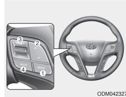
The steering wheel incorporates audio control buttons on the left hand side of the steering wheel.
