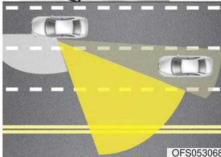
The blind zone mirror (BZM) is supplemental mirror to reduce a driver's blind zone that will show the rear side territory of your vehicle. The blind zone mirror is equipped with the driver's outside rearview mirror.
