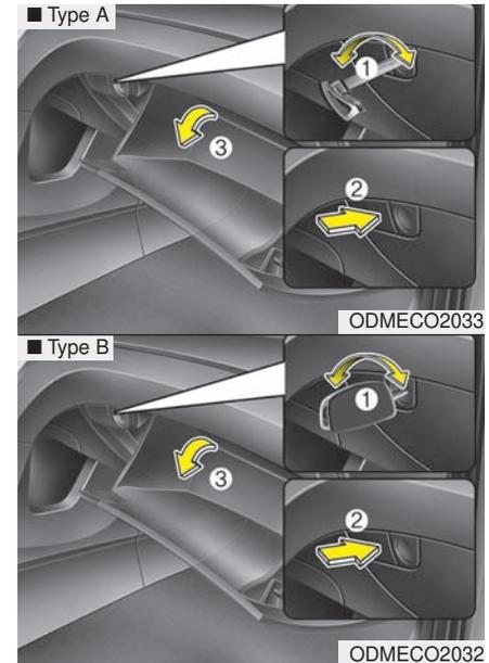
The glove box can be locked and unlocked with the mechanical key (1). To open the glove box, push the button (2) and the glove box will automatically open (3). Close the glove box after use.
