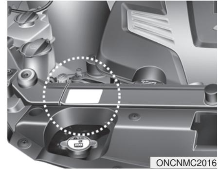
The refrigerant label is located at the front of the engine room.
