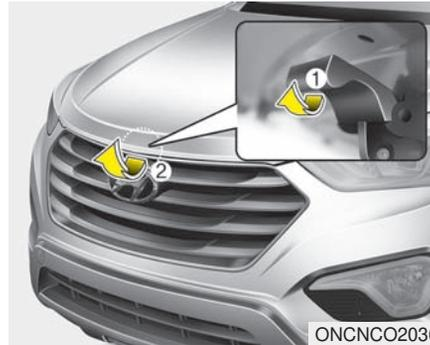
2. Go to the front of the vehicle, raise the hood slightly, pull the secondary latch (1) inside of the hood up and lift the hood (2).
