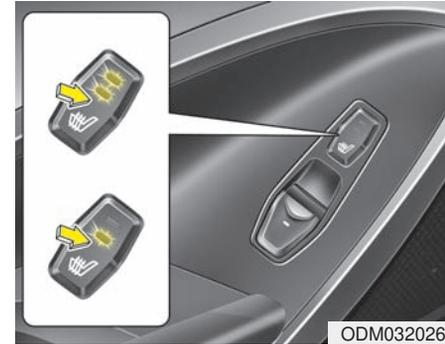
The seat warmer is provided to warm the rear seats during cold weather. With the ignition switch in the ON position, push either of the switches to warm the rear seats.
