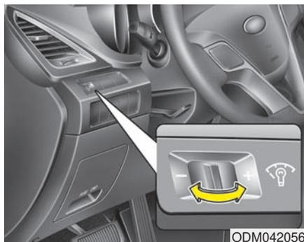
The brightness of the instrument panel illumination is changed by moving the illumination control knob right or left when the ignition switch or Engine Start/Stop button is ON, or the tale lights are turned on.
