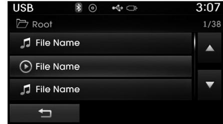
Turn the **TUNE** knob left/right to search for files. Once the desired file is displayed, press the knob to select and play.
