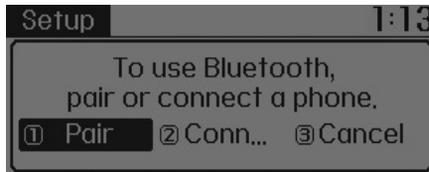
If *Bluetooth*® Wireless Technology devices are paired but none are currently connected, pressing the **PHONE** key or the
