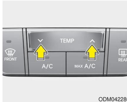
The temperature control switch allows you to control the temperature of the airflow in the vehicle.
