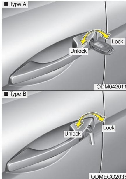
If the smart key or folding key does not operate normally, you can lock or unlock the doors as follows:
