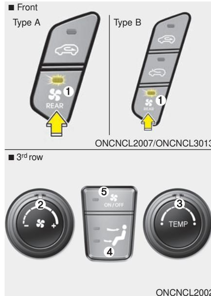
1. To turn the 3<sup>rd</sup> row climate control on or off, press the 3<sup>rd</sup> row climate control ON/OFF button (1 or 5).
