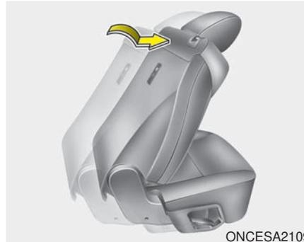
3. The 2nd row seatback will be folded and push the seat to the farthest forward position.
