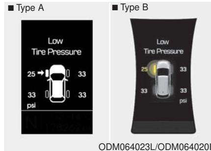
When the tire pressure monitoring system warning indicators are illuminated and warning message displayed on the cluster LCD display, one or more of your tires is significantly under-inflated. The low tire pressure position telltale light will indicate which tire is significantly under-inflated by illuminating the corresponding position light.
