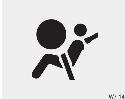
The purpose of the air bag warning light in your instrument panel is to alert you of a potential problem with your airbag system, which includes side and/or curtain airbags used for rollover protection.
