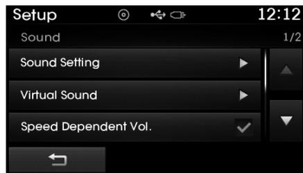
The volume level is controlled automatically according to the vehicle speed. SDVC can be set by selecting from On/Off.
