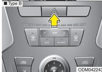
This causes all turn signal lights to blink. The hazard warning lights will operate even though the key is not in the ignition switch.
