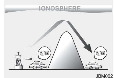
AM broadcasts can be received at greater distances than FM broadcasts. This is because AM radio waves are transmitted at low frequencies. These long distance, low frequency radio waves can follow the curvature of the earth rather than travelling straight. In addition, they curve around obstructions resulting in better signal coverage.
