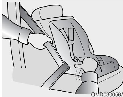
5. Remove as much slack from the belt as possible by pushing down on the child restraint system while feeding the shoulder belt back into the retractor.
