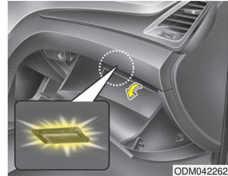
The glove box lamp comes on when the light switch is in the parking light position or headlight position and the glove box is opened.
