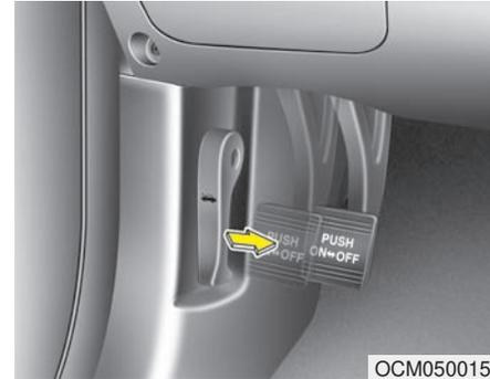
Check whether the stroke is within the recommended specification when the parking brake pedal is fully engaged. When engaged, the parking brake alone should hold the vehicle securely. If the stroke is more or less than specified, have the parking brake adjusted by an authorized HYUNDAI dealer.
