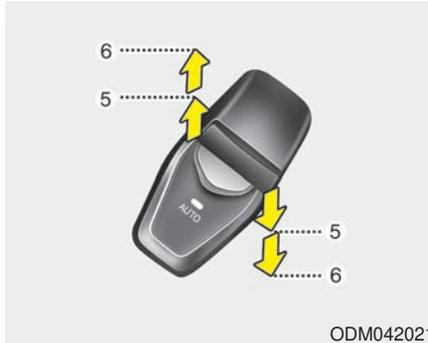
Pressing down or pulling up the power window switch momentarily to the second detent position (6) completely lowers or lifts the window even when the switch is released. To stop the window at the desired position while the window is in operation, momentarily pull or push the switch in the direction opposite of the window's movement.
