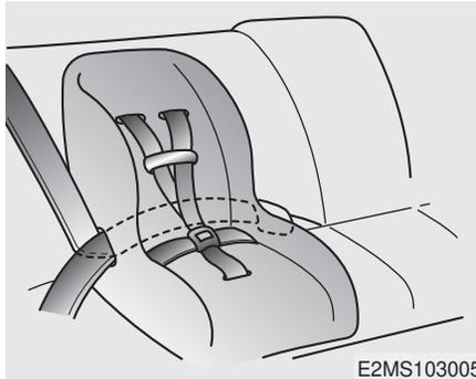
The automatic locking mode will help prevent the normal movement of the child in the vehicle from causing the seat belt to loosen and compromise the child restraint system. To secure a child restraint system, use the following procedure.
