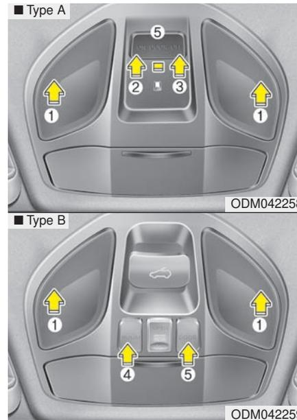
Press the lens (1) to turn the map lamp on or off
