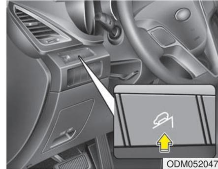
The Downhill Brake Control (DBC) assists the driver when descending a steep hill without the driver depressing the brake pedal. It slows the vehicle to approximately 6.3 mph (10 km/h) and lets the driver concentrate on steering the vehicle.
