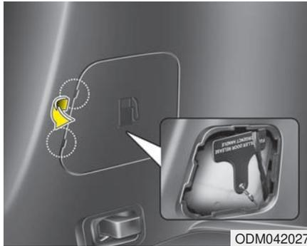
If the fuel filler door does not open using the remote fuel filler door release, you can open it manually. Unsnap and remove the panel in the cargo area. Pull the handle outward slightly.
