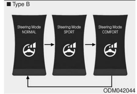
When the steering mode button is pressed, the selected steering mode will appear on the LCD display.
