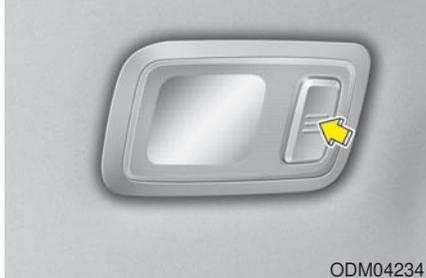
Press the button to turn the light on or off.
