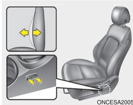
1. Press the front portion of the switch to increase support or the rear portion of the switch to decrease support.
