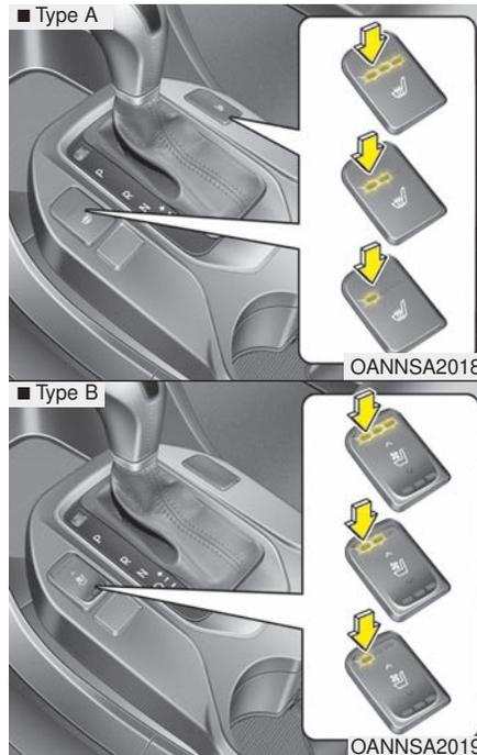
With the ignition switch in the ON position, push either of the switches (red color) to warm the driver's seat or the front passenger's seat.
