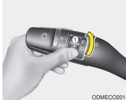
Fog lights are used to provide illumination close to the road surface when visibility is poor due to fog, rain or snow, etc. The fog lights will turn on when the fog light switch (1) is turned to the on position after the headlight is turned on.
