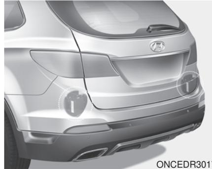
The sensors are located on the inside of the rear bumper.
