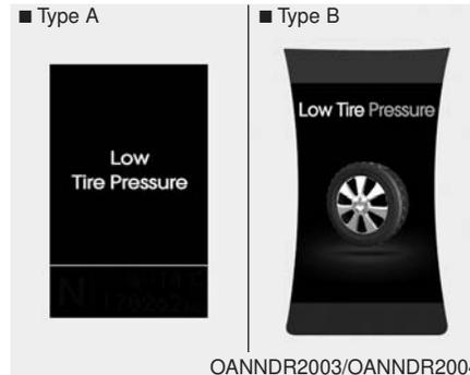
When the tire pressure monitoring system warning indicator is illuminated, one or more of your tires is significantly under-inflated.
