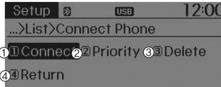
This feature is used to view mobile phones that have been paired with the audio system. Upon selecting a paired phone, the setup menu is displayed.
