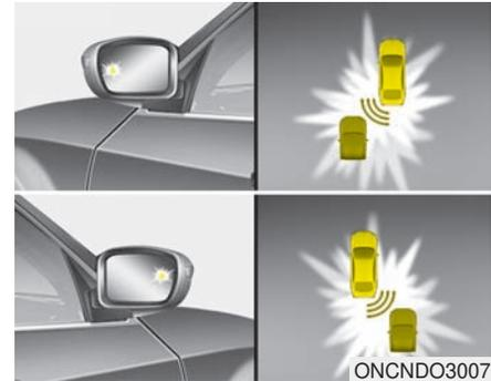
If a vehicle is detected within the boundary of the system, a yellow warning light will illuminate in the outside rearview mirror glass.
