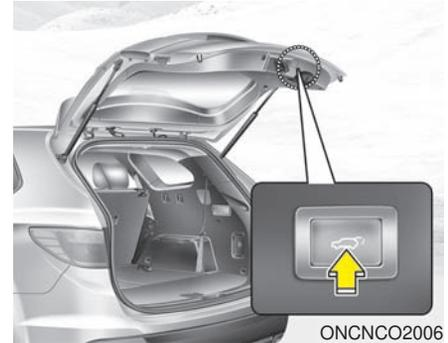
1. Press the power liftgate (power tailgate) close button (approximately 1 second).
