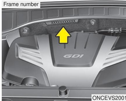
The vehicle identification number (VIN) is the number used in registering your vehicle and in all legal matters pertaining to its ownership, etc. The number is punched on the engine compartment bulkhead.
