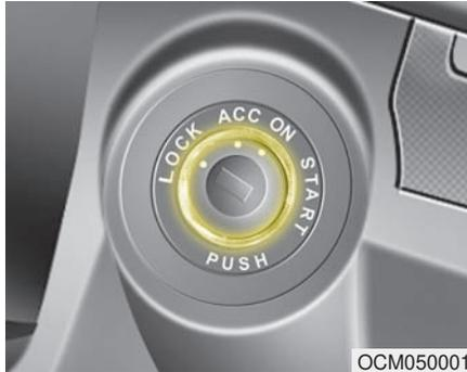
Whenever a front door is opened, the ignition switch will be illuminated for your convenience, provided the ignition switch is not in the ON position. The light will go off immediately when the ignition switch is turned on or go off after about 30 seconds when the door is closed.
