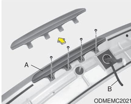
5. Remove the high mounted stop lamp assembly (A) after loosening the nuts and washer nozzle (B).
