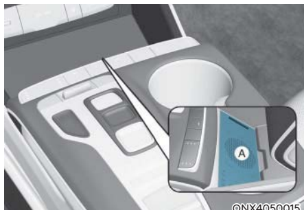
(A): Vehicle authentication pad (Wireless charging pad)
