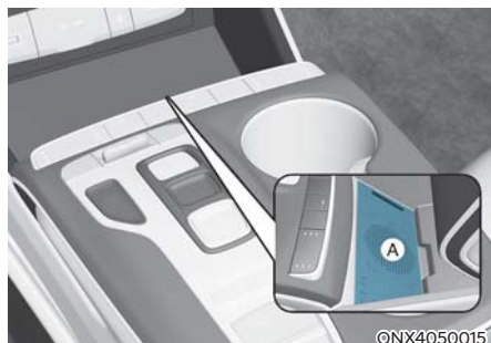
[A] : Wireless Charging Pad (In-vehicle Authentication Pad)
