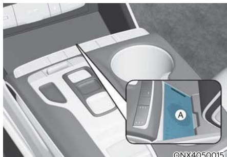
[A] : Wireless Charging Pad (In-vehicle Authentication Pad)
