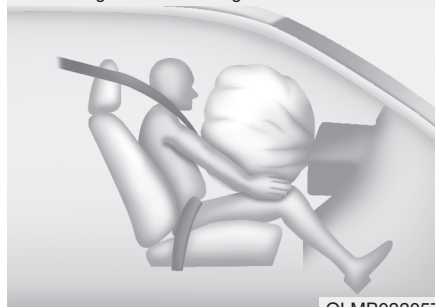
■ Passenger's front air bag
