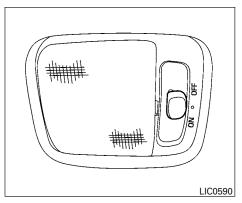
The cargo light on the overhead trim has a threeposition switch. To operate, push the switch to the desired position.
