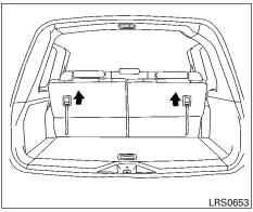
To return the 3rd row seats to a seating position, use the pull straps to raise each seatback. Pull back until the seatbacks latch into position.
