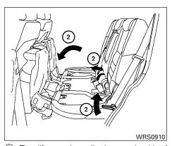
Then lift up on the recline lever on the side of the outboard seats to fold the outboard seatbacks flat. To fold the center seatback flat. pull up on the strap on the edge of the center seat cushion and fold the seatback toward the front of the vehicle.
