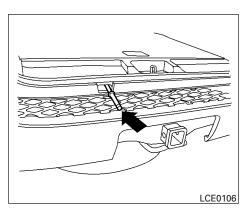
4. Find the oval-shaped opening above the middle of the bumper. Pass the T-shaped end of the jack rod through the opening and direct it toward the spare tire winch, located directly above the spare tire.
