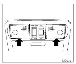
To turn the map lights on, press the switches. To turn them off, press the switches again.
