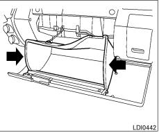
Open the glove box and press in on the sides so that it will open completely allowing it to hang by the cord.
