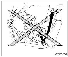
Even with the NISSAN Advanced Air Bag System, never install a rear-facing child restraint in the front seat. An inflating front air bag could seriously injure or kill your child. See "Child restraints" earlier in this section for details.
