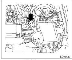
**VQ40DE** engine CHECKING ENGINE OIL LEVEL
