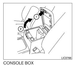
Pull up on the lever 1 to open the console box lid
