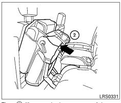
Then ② lift up on the lower corner of the seat base and tip the outboard seating position of the 2nd row bench seat forward. To exit the 3rd row bench seat, lift up on the same seatback latch and fold the seatback forward onto the seat base. Then lift up on the seat base and tip it forward.
