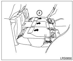
There is a carpet panel flap on the back of each seat that can be folded toward the back of the vehicle.
