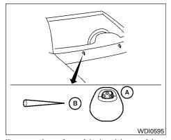
If you wax the surface of the hood, be careful not to let wax get into the washer nozzle (a). This may cause clogging or improper windshield washer operation. If wax gets into the nozzle, remove it with a needle or small pin (a).
