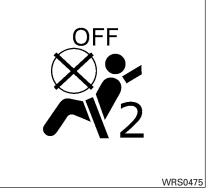
7. If the booster seat is installed in the front passenger seat, place the ignition switch in the ON position. The front passenger air bag status light \* may or may not illuminate, depending on the size of the child and the type of booster seat being used. See "Front passenger air bag and status light" later in this section.
