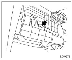
2. Lift upward on the retainer to release the filter cover and remove the filter cover.
