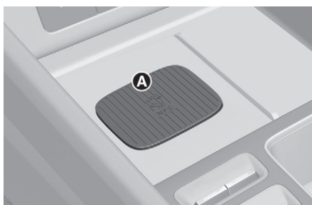
[A] Vehicle authentication pad (Wireless charging pad)
