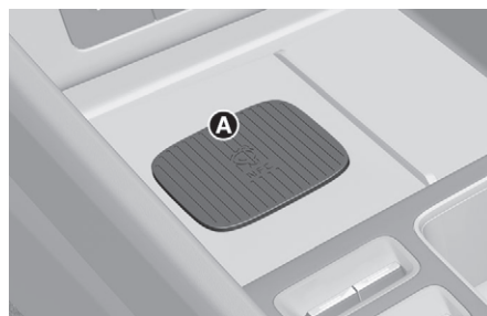
[A] Vehicle authentication pad (wireless charging pad)
