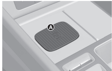
[A] Vehicle authentication pad (Wireless charging pad)
