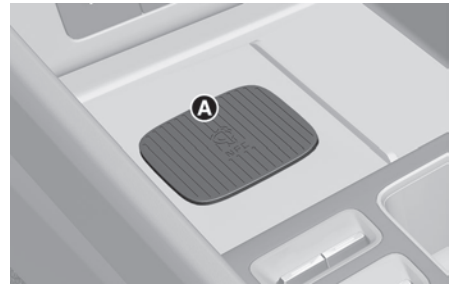
[A] Vehicle authentication pad (wireless charging pad)
