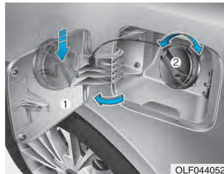
3. Pull the fuel filler door (1) out to fully open.
