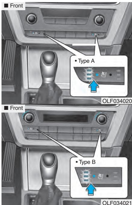
The air ventilation seats are provided to cool the front seats by blowing air through small vent holes on the surface of the seat cushions and seatbacks.
