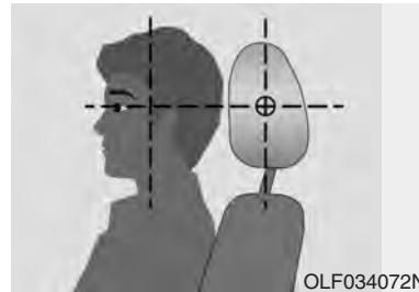
Adjust the head restraints so the middle of the head restraints is at the same height as the height of the top of the eyes.
