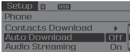
This feature is used to automatically download mobile contacts entries once a *Bluetooth®* Wireless Technology phone is connected.
