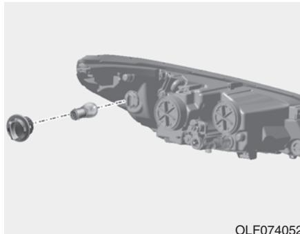
5. Insert a new bulb by inserting it into the socket and rotating it until it locks into place.
