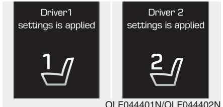
"Driver 1(or 2) settings is applied" will appear on the LCD display.
