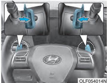
The paddle shifter is available when the shift lever is in the D (Drive) position or Sports Mode.
