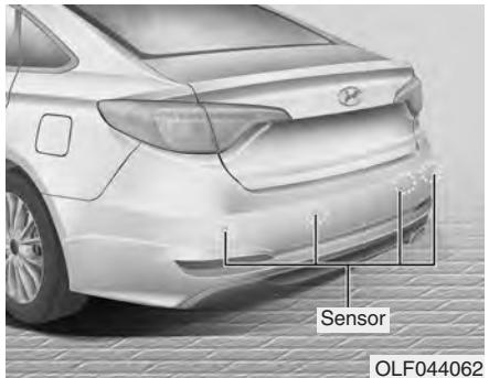
The Rear Parking Assist System assists the driver during reverse movement of the vehicle by chiming if any object is sensed within the distance of 50 inches (120 cm) behind the vehicle.
