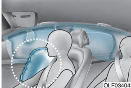
The side air bags are designed to deploy only during certain side impact collisions, depending on the crash severity, angle, speed and point of impact.
