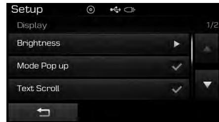
This feature is used to display the Pop-up Mode screen when entering radio and media modes.
