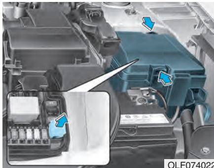
5. Pull the suspected fuse straight out. Use the removal tool provided in the engine compartment fuses panel.
