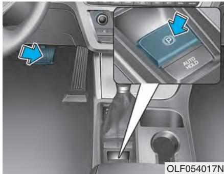
To release the EPB (Electric Parking Brake), press the EPB switch in the following condition:
