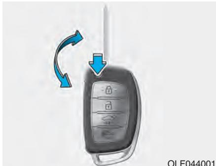
Press the release button then the key will unfold automatically.
