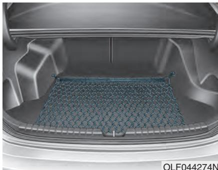
To keep items from shifting in the trunk, you can use the 4 holders located in the trunk to attach the luggage net.
