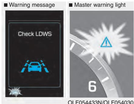
When the LDWS is not working properly, the warning light will illuminate and the warning message will come on for a few seconds. After the message disappears, the master warning light will illuminate.
