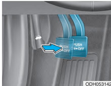
Check whether the stroke is within specification when the parking brake pedal is depressed with 44 lb (20 kg, 196 N) of force. Also, the parking brake alone should securely hold the vehicle on a fairly steep grade. If the stroke is more or less than specified, have the parking brake adjusted by an authorized HYUNDAI dealer.
