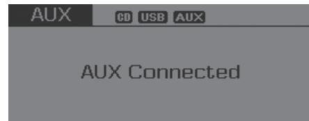
\* AUX mode cannot be started unless there is an external device connected to the AUX terminal.
