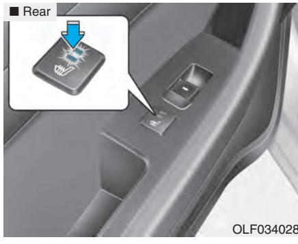
While the engine is running, push either of the switches to warm the driver's seat or passengers' seat.
