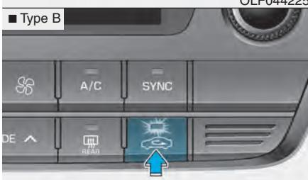
This button is used to select the outside (fresh) air position or recirculated air position.
