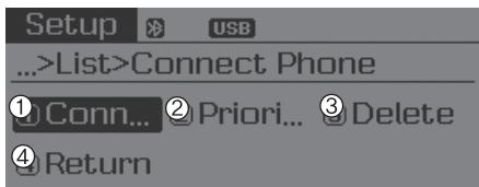
This feature is used to view mobile phones that have been paired with the audio system. Upon selecting a paired phone, the setup menu is displayed.
