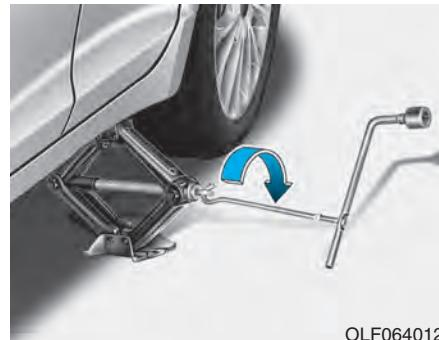
9. Insert the jack handle into the jack and turn it clockwise, raising the vehicle until the tire clears the ground. Make sure the vehicle is stable on the jack.
