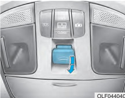
4. Push the sunroof control lever forward in the direction of close until the sunroof operates as follows:
