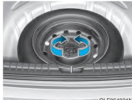
Turn the winged hold down bolt counterclockwise to remove the spare tire.
