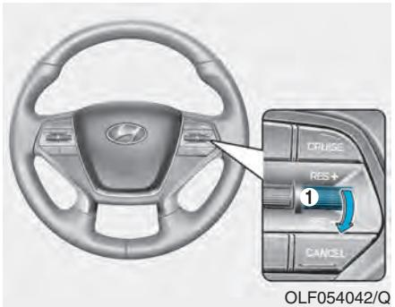
3. Push the lever (1) down (SET-), and release it. The SET indicator light will illuminate.
