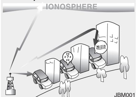
This can be due to factors, such as the distance from the radio station, closeness of other strong radio stations or the presence of buildings, bridges or other large obstructions in the area.
