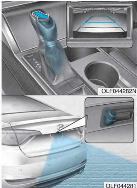
The Rear View Camera will activate when the engine is running and the shift lever is in the R (Reverse) position.
