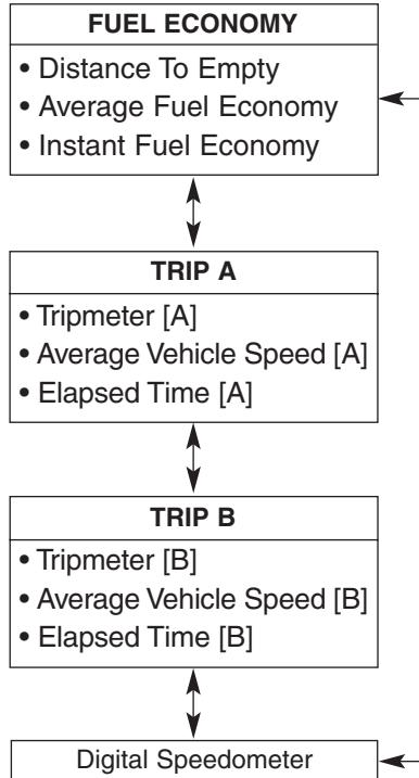
To change the trip mode, rotate the MOVE switch “▲, ▼” on the steering wheel.
