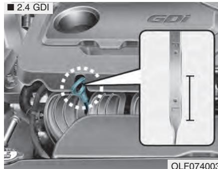
6. Pull the dipstick out again and check the level. The level should be between F and L.
