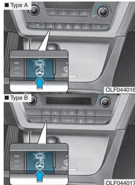
When the ignition switch is in the ON position or when the engine is running, press the heated steering wheel button to warm the steering wheel. The indicator on the button will illuminate.
