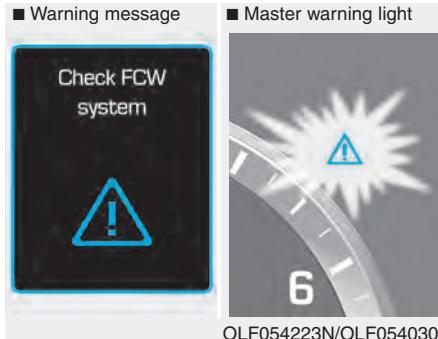
When the FCWS is not working properly, the warning message will come on for a few seconds. After the message disappears, the master warning light will illuminate.
