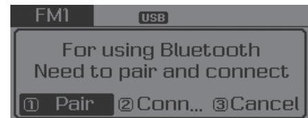
If *Bluetooth®* Wireless Technology devices are paired but none are currently connected, pressing the **PHONE** key or the
