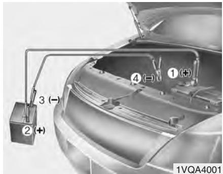
4. Connect the jumper cables in the exact sequence shown in the illustration. First connect one jumper cable to the red, positive (+) jumper terminal of your vehicle (1).
