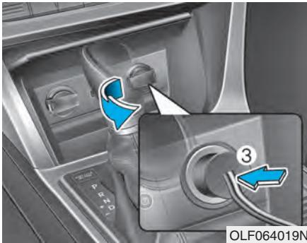
7. Plug the compressor power cord (3) into the vehicle power outlet.
