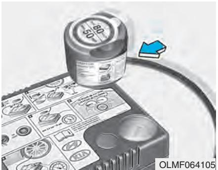
5. Insert the sealant bottle into the housing (4) of the compressor so that the bottle is upright.
