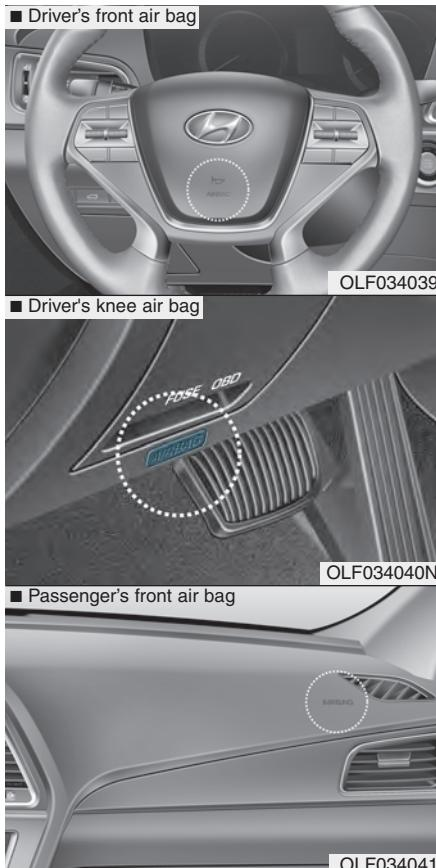
The purpose of the SRS is to provide the vehicle's driver and front passengers with additional protection than that offered by the seat belt system alone. The SRS uses sensors to gather information about the driver's and front passenger's seat belt usage and impact severity.
