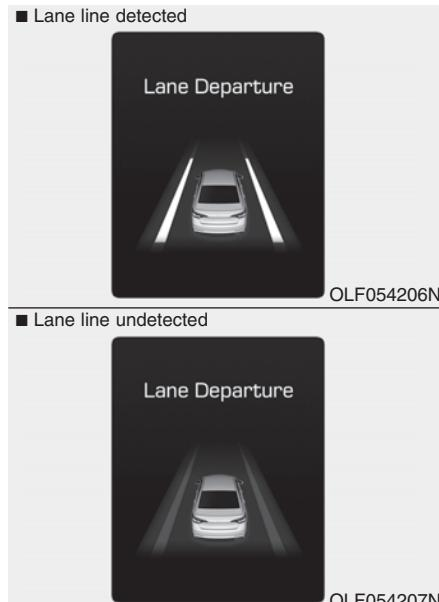
If the vehicle leaves the lane when the LDWS is operating and vehicle speed exceeds 44mph (70km/h), the warning operates as follows:
