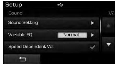
The volume level is controlled automatically according to the vehicle speed. SDVC can be set by selecting from On / Off.
