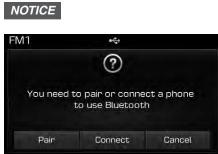
If **Bluetooth® Wireless Technology** devices are paired but none are currently connected, pressing the **PHONE** key or the
