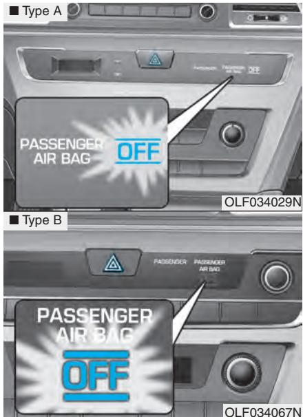
Your vehicle is equipped with an Occupant Classification System (OCS) in the front passenger's seat.
