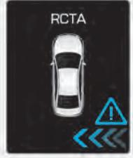
If the vehicle detected by the radars approaches your vehicle, the warning chime will sound, the warning light on the outside rearview mirror will blink and a message will appear on the LCD display.
