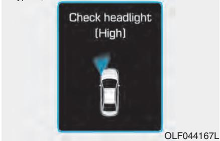
This warning message illuminates if there is a malfunction (burned-out bulb except LED lamp or circuit malfunction) with the headlamp. In this case, have your vehicle inspected by an authorized HYUNDAI dealer.
