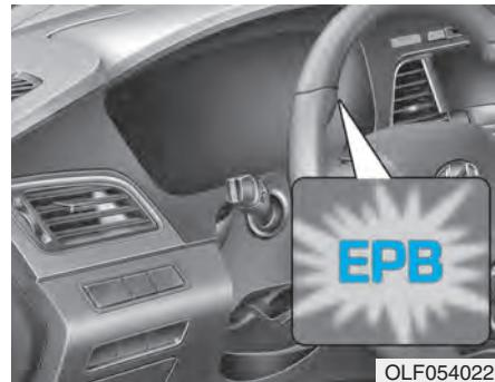
If the EPB Malfunction Indicator remains on, comes on while driving, or does not come on when the Engine Start/Stop button is in the ON position, this indicates the EPB may have malfunctioned. Have your vehicle checked by an authorized HYUNDAI dealer as soon as possible.
