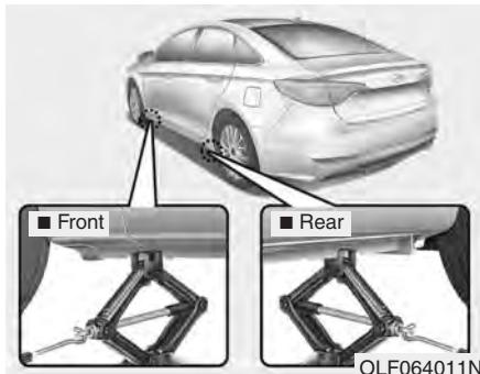
8. Place the jack at the designated jacking position under the frame closest to the tire you are changing. The jacking positions are plates welded to the frame with two notches and two dimples. Never jack any other position or part of the vehicle. It may damage to the side seal molding.
