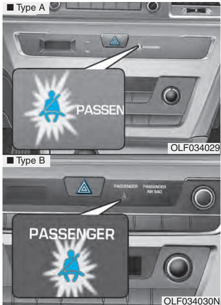
The front passenger's seat belt warning light will activate to the following table when the ignition switch is in "ON" position.
