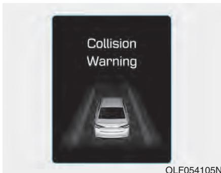
Go to the User Settings Mode (Driving Assist) and select FCW (Forward Collision Warning) on the LCD display (**For more details, refer to "LCD Display" in chapter 3.**). The system will turn on and standby to activate. The system will activate when vehicle speed is above 25 mph (40 km/h) and below 90 mph (145 km/h).
