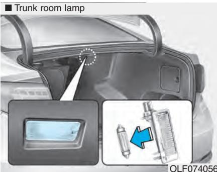
1. Using a flat-head screwdriver, gently pry the lens from the interior light housing.
