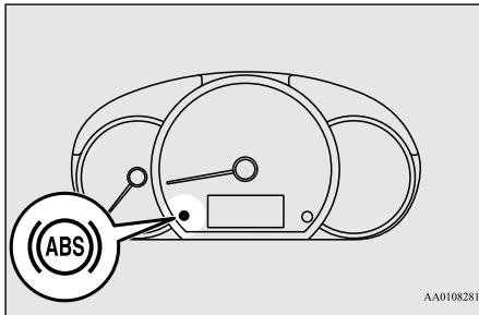
If there is a malfunction in the system, the anti-lock braking system warning light will come on.
