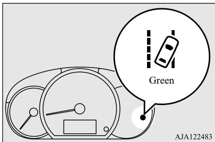
To turn off the LDW, press the LDW switch. The LDW indicator (green) in the meter cluster will then go out.
