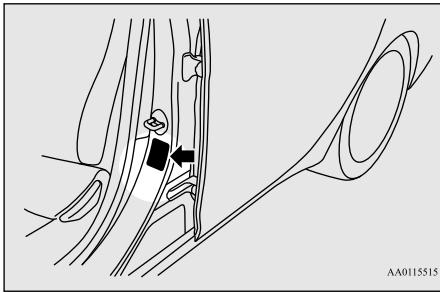
This placard shows the maximum number of occupants permitted to ride in your vehicle as well as “the combined weight of occupants and cargo” (A), which is called the vehicle capacity weight. This placard also tells you the size and recommended inflation pressure for the original equipment tires on your vehicle. For more information, refer to “Tires” on page 9-13.
