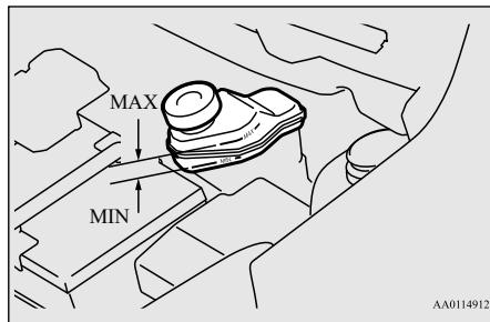
The fluid level falls slightly with wear of the brake pads, but this does not indicate any abnormality.
