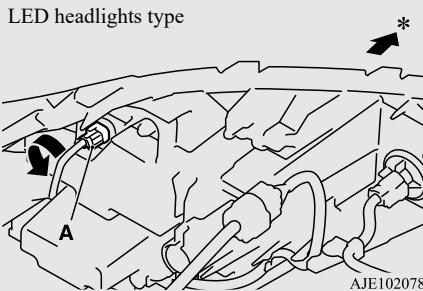
2. Pull the bulb out of the socket.
