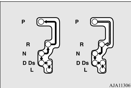
The CVT selects an optimum ratio automatically when the selector lever is in the “D” (DRIVE) position, depending on the speed of the vehicle and the position of the accelerator pedal.
