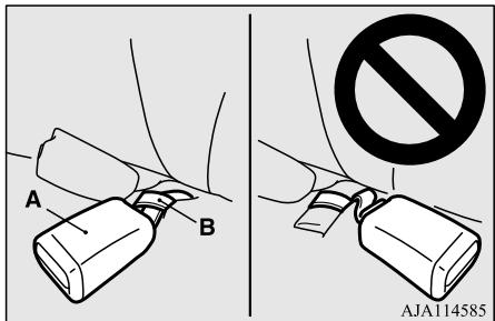
2. Route the seat belt through the child restraint system according to the instructions provided by the child restraint system's manufacturer. Then insert the seat belt latch plate into the buckle. Make sure you hear a "click" when you insert the latch plate into the buckle.
