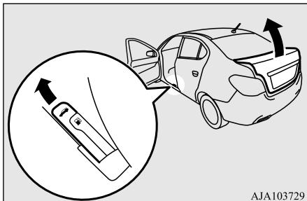
Pull the trunk lid release lever, located to the left of the driver's seat, up to open the trunk.
