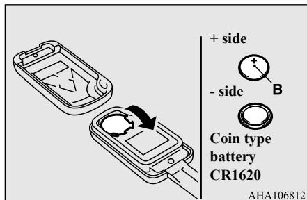
6. Close the remote control transmitter firmly.
