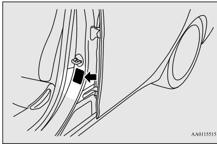
This placard shows the maximum number of occupants permitted to ride in your vehicle as well as “the combined weight of occupants and cargo” (A), which is called the vehicle capacity weight. This placard also tells you the size and recommended inflation pressure for the original equipment tires on your vehicle. For more information, refer to “Tires” on page 9-12.
