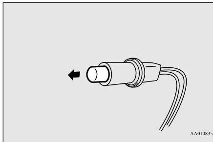
2. Remove the bulb from the socket by turning it counterclockwise while pressing in.
