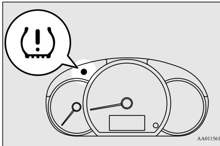
When the ignition switch is turned to the "ON" position or the operation mode is put in ON, the tire pressure monitoring system warning light normally illuminates and goes off a few seconds later.
