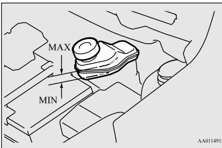
The fluid level falls slightly with wear of the pump, but this does not indicate any abnormality.
