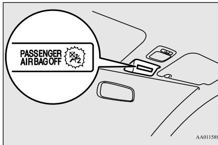
The indicator normally comes on when the ignition switch is turned to the “ON” position or the operation mode is put in ON, and goes out a few seconds later. In the following situations, the indicator will stay on to show that the passenger front airbag is not operational.
