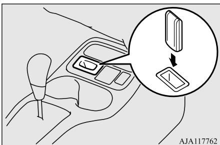
4. With the first valid F.A.S.T.-key, press the UNLOCK button for 4 to 8 seconds and press the LOCK button during this time.
