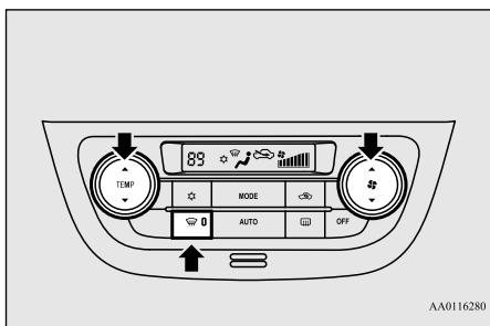
1. Push the defogger switch to change to the “
