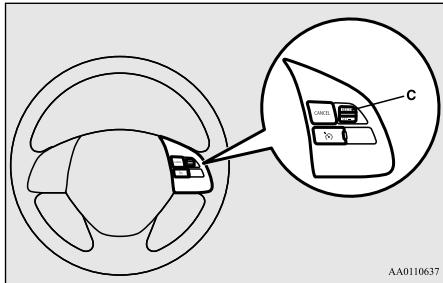
To increase your speed in small amounts, press the RES + switch for less than about 1 second and release it.
