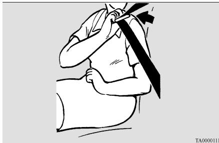
4. The lap part of the belt must always be worn low and snug across the hips. Pull up on the shoulder portion of the belt to take up any slack in the lap belt.
