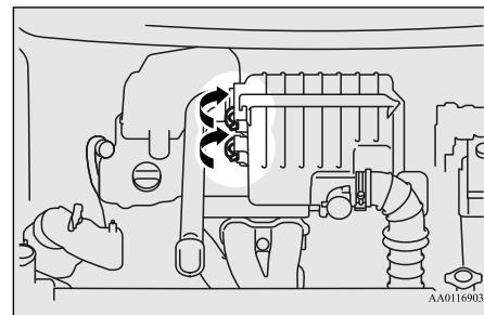
2. Replacing the air cleaner filter and put the cover back on in its original position.
