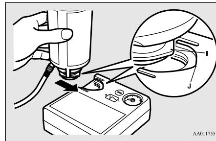
● When installing the bottle, align the projection (I) on the bottle with the indentation (J) in the compressor.
