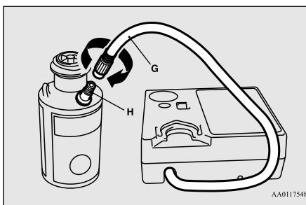
10. Install the bottle onto the compressor.
