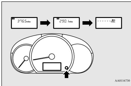
2. Press and hold the multi-information display switch for about 1 second or more to make the spanner mark start flashing. (If there is no operation for about 10 seconds with flashing, the display will revert to its original indication.)
