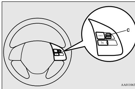
To increase your speed in small amounts, press the RES + switch for less than about 1 second and release it.
