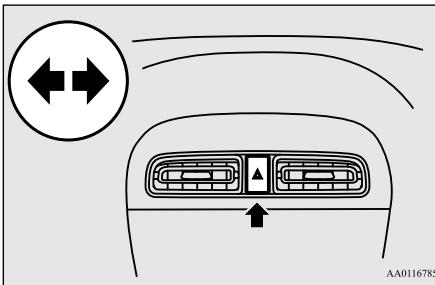
If you press the flasher switch, the turn signals will flash intermittently, and so will the hazard warning lights. This is an emergency warning system and should not be used when the vehicle is in motion, except for emergencies.
