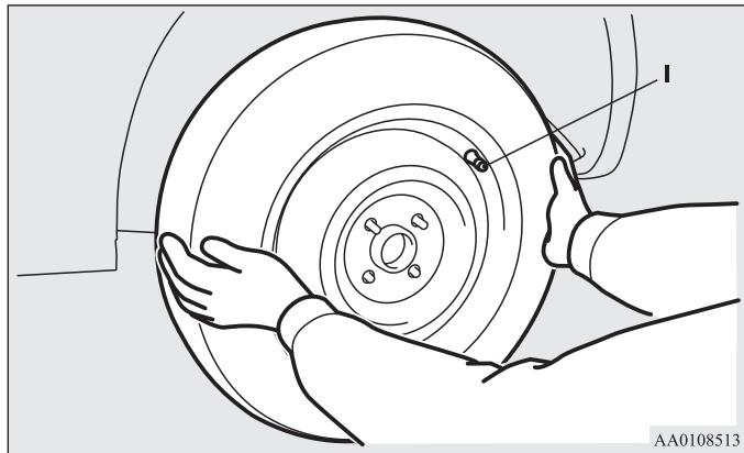
7. Install the wheel nuts with their tapered ends facing inward, then tighten by hand until the wheel is no longer loose.
