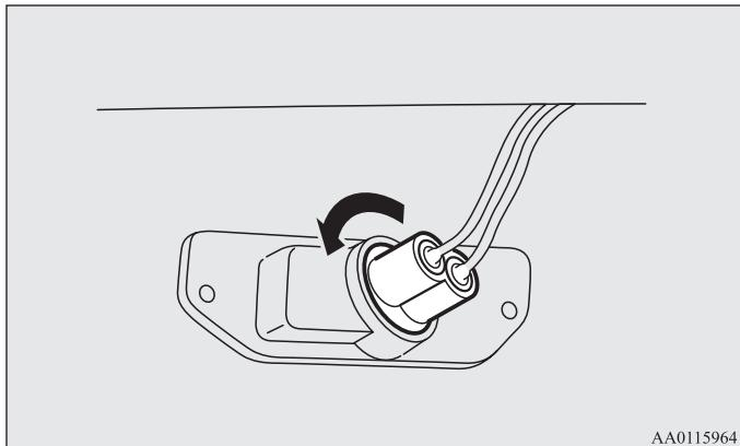
3. Pull the bulb out of the socket.
