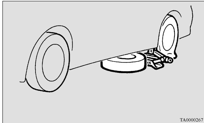
3. Rotate the jack by hand until the flange portion (B) fits in the groove (C) at the top of the jack.
