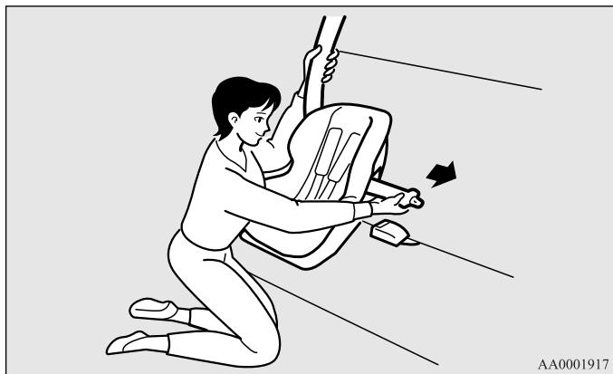
3. To activate the ALR child restraint installation function, slowly pull the shoulder part of the belt all the way out of the retractor until it stops. Then let the belt feed back into the retractor.
