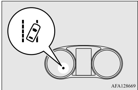
To turn the LDW back on, press the LDW switch again. The LDW indicator in the instrument cluster will then come on.
