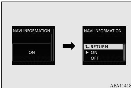
3. Press the **▼** switch or **▲** switch to select the setting, and then press the **□** switch to confirm the setting.
