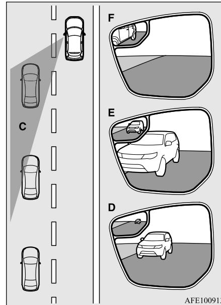
D- When a vehicle is traveling far behind your vehicle, the main mirror (B) shows an image of the vehicle and the Integrated Blind Spot Mirror (A) shows a small image of the vehicle.
