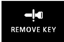
If the ignition switch is turned to the "OFF" position and the driver's door is opened with the key in the ignition switch, the key reminder buzzer will sound intermittently to remind you to remove the key.
