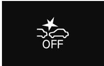
To turn on the FCM again, press the FCM ON/OFF switch. The
