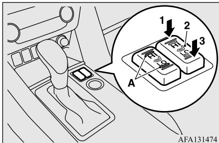
1 (HI) - Heater high (for quick heating)
