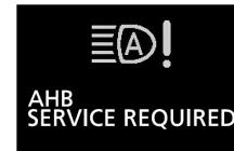
[When the sensor is malfunctioning]
