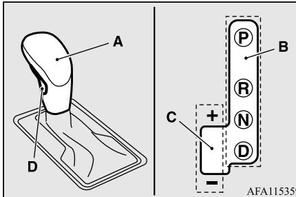
In the main gate, selector lever has four positions, and is equipped with a lock button (D) to avoid inadvertent selection of the wrong gear.
