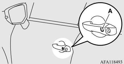
Front passenger's door lock/unlock switch
