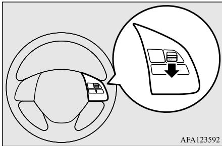
To slow down your speed in small amounts, push down the “SET -” switch for less than approximately 1 second and release it. Each time you push down the “SET -” switch, your vehicle will slow down by approximately 1 mph (1.6 km/h).
