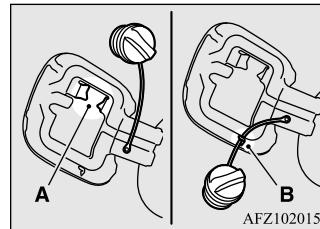
4. Fueling correctly depends mainly on correct handling of the fuel filler nozzle. Do not tilt the nozzle. Insert the nozzle in the fuel tank filler port as far as it goes.
