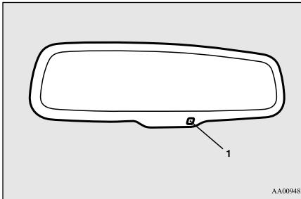
When the operation mode is put in ON, the reflection factor of the mirror is automatically changed.
