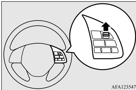
While the ACC system is in the stationary vehicle hold state, if it is possible to resume following the vehicle in front because it has started moving, “ACC READY TO RESUME” will appear on the meter. To start
