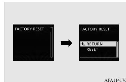
3. Press the **▼** switch or **▲** switch to select “RESET”, and then press and hold the **□** switch for approximately 5 seconds or more to confirm the setting.
