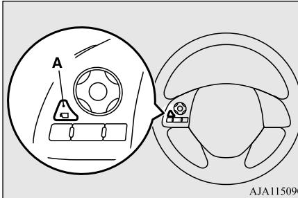
3. Press and hold down the switch (A) until the vehicle icon blinks to enter the selection mode of the vehicle icon color in the bird's eye-view.
