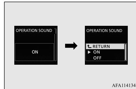
3. Press the **▼** switch or **▲** switch to select the sound, and then press the **■** switch to confirm the setting. The setting is changed to the selected condition.
