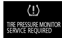
Each tire, should be checked monthly when cold and inflated to the inflation pressure recommended by the vehicle manufacturer on the vehicle placard or tire inflation pressure label. (If your vehicle has tires of a different size than the size indicated on the vehicle placard or tire inflation pressure label, you should determine the proper tire inflation pressure for those tires.)
