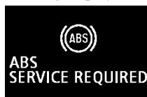
If there is a malfunction in the system, the ABS warning light will come on and the warning display will appear on the information screen in the multi-information display. Under normal conditions, the ABS warning light only comes on when the operation mode
