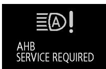
[When the sensor is malfunctioning]
