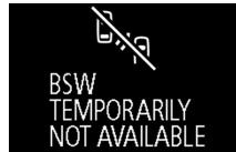
When the warning display appears, the sensor is temporarily not available for some reason such as the environmental condition or increase of the sensor temperature. When the warning display does not disappear after waiting for a while, contact a certified Mitsubishi EV dealer.
