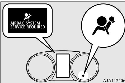
The system checks itself every time the operation mode of the power switch is put in ON. The SRS warning light will come on for several seconds and then go out. This is normal and means the system is working properly.
