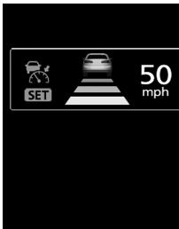
When the front vehicle stops, the ACC will automatically apply the brakes to stop your vehicle.
