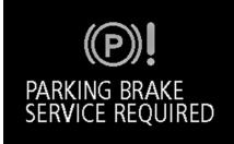
If there is a malfunction in the system, the warning light will come on. In addition, the warning display appears on the information screen in the multi-information display.
