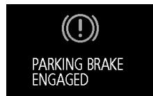
If the Electric parking brake cannot be applied automatically due to the system malfunction, the message will appear on the information screen in the multi-information display. Depress the brake pedal.
