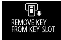
If the operation mode is in OFF and the driver's door is opened with the F.A.S.T.-key in the key slot, a warning is issued with the warning display and the buzzer buzzing for approximately 3 seconds to remind you to remove the key.
