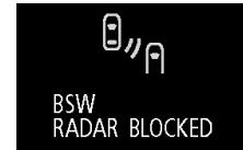
When the warning display appears, the sensor cannot detect a vehicle traveling side by side or an approaching vehicle, because foreign objects, such as dirt, snow or ice, adhere to the bumper surface around the sensor.
