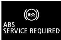
If there is a malfunction in the system, the ABS warning light will come on and the warning display will appear on the information screen in the multi-information display. Under normal conditions, the ABS warning light only comes on when the operation mode
