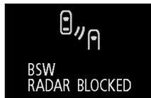
When the warning display appears, the sensor cannot detect a vehicle traveling side by side or an approaching vehicle, because foreign objects, such as dirt, snow or ice, adhere to the bumper surface around the sensor. Remove a dirt, freezing or foreign material on the bumper surface around the sensor. When the warning display does not disappear after having cleaned the bumper surface around the sensor, contact a certified Mitsubishi EV dealer.
