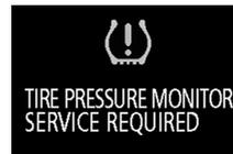
Each tire, should be checked monthly when cold and inflated to the inflation pressure recommended by the vehicle manufacturer on the vehicle placard or tire inflation pressure label. (If your vehicle has tires of a different size than the size indicated on the vehicle placard or tire inflation pressure label, you should determine the proper tire inflation pressure for those tires.)
