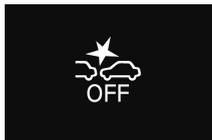
To turn on the FCM again, press and hold the FCM ON/OFF switch. The
