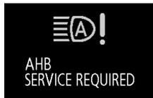
[When the sensor is malfunctioning]
