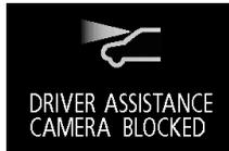
When the sensor performance returns, the FCM functions will resume operation. If the message continues showing, there is a possibility that the sensor has a malfunction. Contact a certified Mitsubishi EV dealer for inspection of the sensor.
