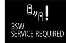
When the warning display appears, the BSW does not operate normally because there are some malfunctions in the system or the sensor. Have the vehicle inspected at a certified Mitsubishi EV dealer as soon as possible.
