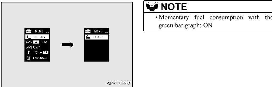
3. Press and hold the multi-information meter switch (for about 5 seconds or more), the buzzer sounds and all of the function settings are returned to the factory settings.
