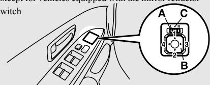
Vehicles equipped with the mirror retractor switch
