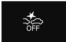
To turn on the FCM again, press the FCM ON/OFF switch. The
