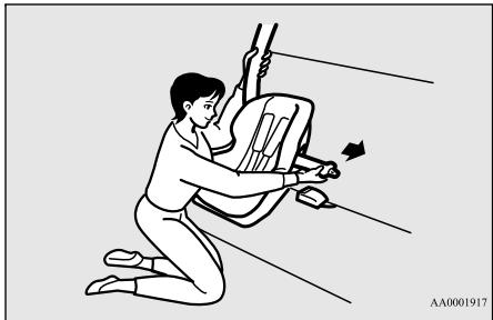
3. To activate the ALR child restraint installation function, slowly pull the shoulder part of the belt all the way out of the retractor until it stops. Then let the belt feed back into the retractor.
