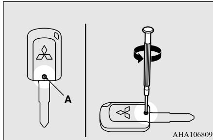
3. With the Mitsubishi mark facing you, insert the cloth-covered tip of a flat-blade screwdriver into the notch in the remote control transmitter case and use it to open the case.
