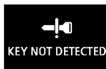
When the operation mode in any mode other than OFF, if the door(s) are opened, the F.A.S.T.-key is removed from the passenger compartment, and then the door(s) are closed, the warning display is displayed and the buzzer sounds 4 times as a warning since it's impossible to verify the ID codes of the F.A.S.T.-key and vehicle.
