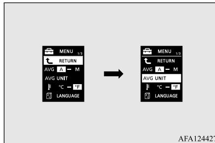
3. Press and hold the multi-information meter switch (for about 2 seconds or more) to display “AVG UNIT” (fuel consumption display unit setting).
