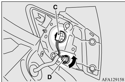
C- Rear side-marker light, stop light, and tail and stop light (LED)
