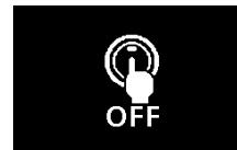
If the driver's door is opened while the engine is stopped and the operation mode is in any position other than OFF, the operation mode ON buzzer will sound intermittently to remind you to put the operation mode in OFF. The warning display will be displayed on the information screen in the multi-information display.
