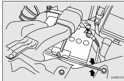
The electrolyte level must be between the limits shown on the outside of the battery. Fill it with distilled water as needed. The inside of the battery is divided into several compartments. Take the cap off of each compartment and fill to the mark.
