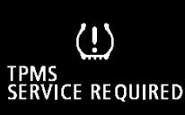
Each tire, including the spare (if provided), should be checked monthly when cold and inflated to the inflation pressure recommended by the vehicle manufacturer on the vehicle placard or tire inflation pressure label. (If your vehicle has tires of a different size than the size indicated on the vehicle placard or tire inflation pressure label, you should determine the proper tire inflation pressure for those tires.)
