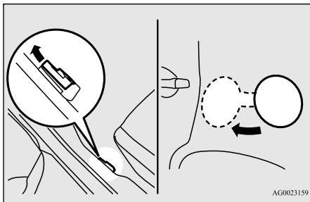
3. Open the fuel tank filler pipe by slowly turning the fuel tank filler cap counter-clockwise.
