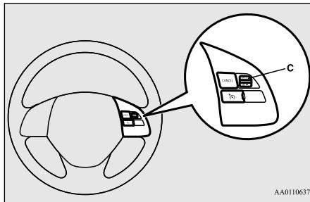
To increase your speed in small amounts, push up the RES + switch for less than about 1 second and release it.
