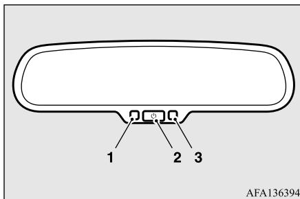
Normally, use the automatic mode. When the ignition switch is turned to the “ON” position or the operation mode is put in ON, the indicator (1) illuminates and the reflection factor of the mirror is automatically changed.
