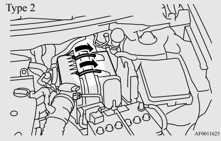
4. Replacing the air cleaner filter and put the cover back on in its original position.
