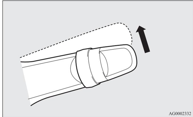
The wipers will operate once if the lever is moved to the “AUTO” position and the knob (C) is turned in the “+” direction when the ignition switch or the operation mode is in ON.
