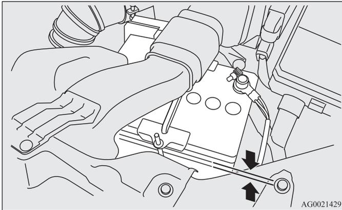
7 The electrolyte level must be between the limits shown on the outside of the battery. Fill it with distilled water as needed. The inside of the battery is divided into several compartments. Take the cap off of each compartment and fill to the mark. Do not fill above the top line because a spill during driving could cause damage.
