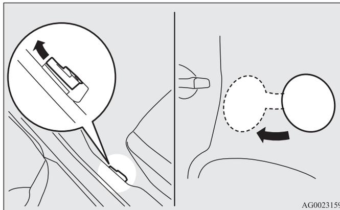
3. Open the fuel tank filler pipe by slowly turning the fuel tank filler cap counterclockwise.
