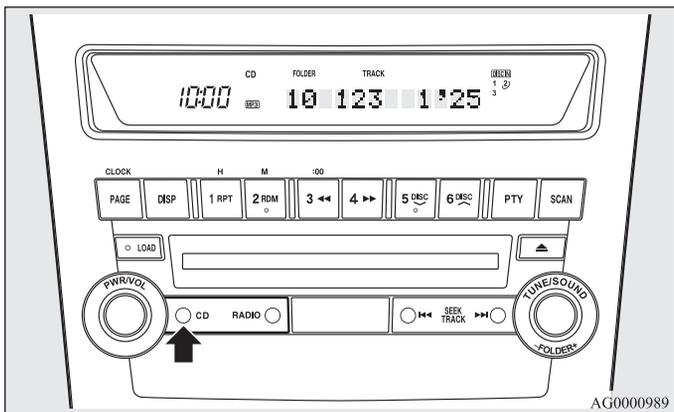
Push the CD button if a disc is already in the audio system. The display shows “READING”, then playback begins. The folder number, the track number, the playing-time, and “MP3” indicator will appear on the display.
