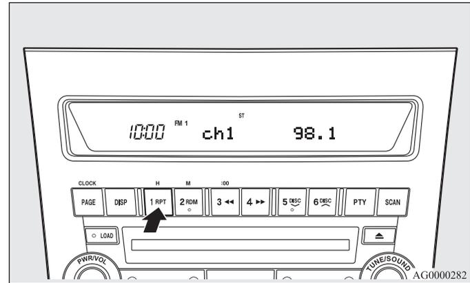
3. To recall a frequency that has been saved in memory, press the corresponding button briefly for no longer than about 1 second.
