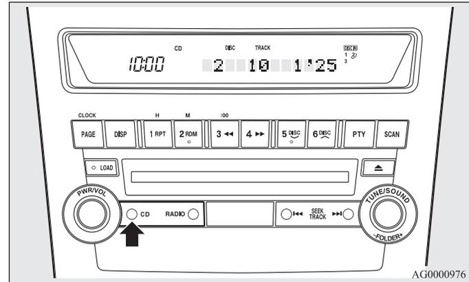
Push the CD button if a disc is already in the audio system. The audio system will enter CD mode and start playback. The disc number (if the audio system is equipped with the CD changer), the track number, and the playing time will appear on the display. The discs in the CD changer unit will be played consecutively and continuously.
