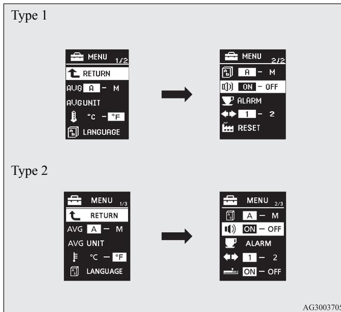
3. Press and hold the multi-information meter switch (for about 2 seconds or more) to switch in sequence from ON (operation sound on) → OFF (operation sound off) → ON (operation sound on).
