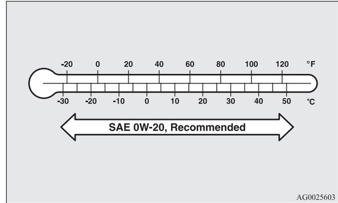
SAE 0W-20 engine oil is strongly recommended for optimum fuel economy and cold starting. If SAE 0W-20 is not available, the ILSAC certification oil of other viscosity grades can be temporarily used.
