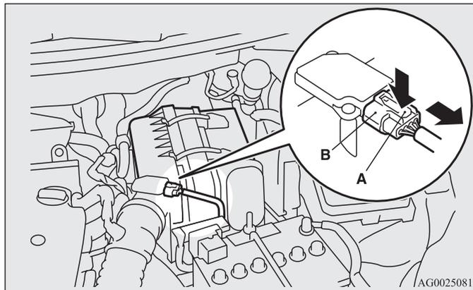
3. Unclamp the cover. Open up the top of the cover and take out the air cleaner filter.
