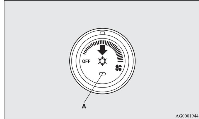
Push the switch again and the air conditioning compressor will stop and the indicator light (A) goes off.
