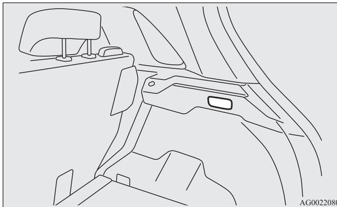
The light illuminates when the liftgate is opened, and goes out when the liftgate is closed.
