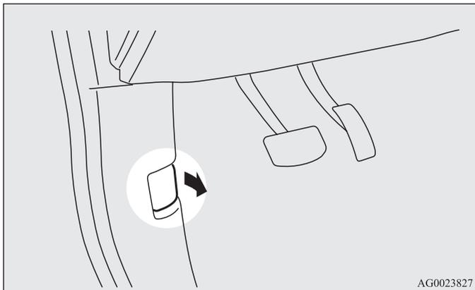
Release the lever and lift the engine hood.
