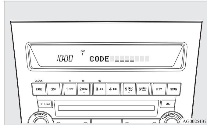
6. If the entered code is correct, "UNLOCKED" will be shown and the locked channel(s) will be unlocked. The satellite radio will then return to the LOCK setting mode. If the entered code is incorrect, a warning sound will be emitted and "CODE ERROR" will be displayed. The code entry window will then be shown again. You can try to enter the code again, no matter how many times an incorrect code has been entered.
