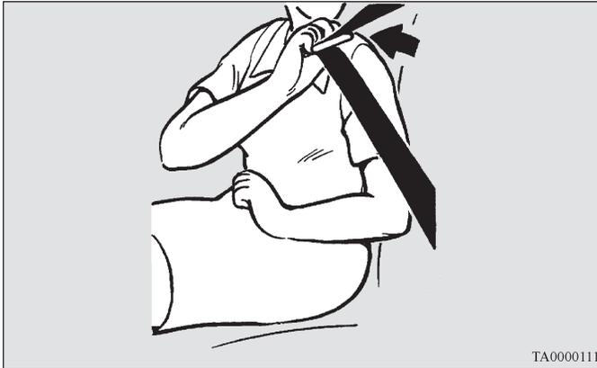
4. Pull the seat belt out slowly while holding the latch plate. Push the latch plate into the buckle until you hear a “click”. Pull up on the belt to be sure the latch plate is locked securely in the buckle.
