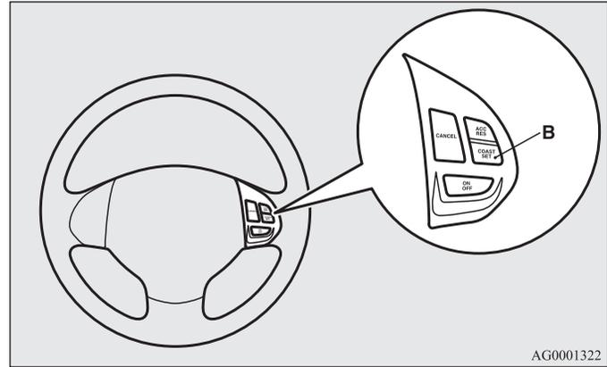
To slow down your speed in small amounts, press the “COAST SET” switch for less than about 1 second and release it. Each time you press the “COAST SET” switch, your vehicle will slow down by about 1 mph (1.6 km/h).
