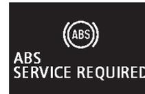
If there is a malfunction in the system, the anti-lock braking system warning light will come on and the warning display will appear on the information screen in the multi-information display.
