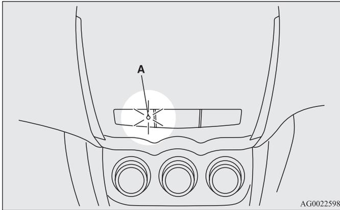
4. The system has entered the armed stage after about 20 seconds, when the theft-alarm indicator (A) flashing becomes slower.
