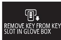
If the operation mode is in OFF and the driver’s door is opened with the F.A.S.T.-key in the key slot, a warning is issued with
