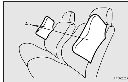
A label is attached to the seatbacks in vehicles equipped with side airbags.
