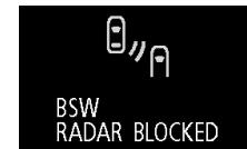
When the warning display appears, the radar sensor cannot detect a vehicle traveling side by side or an approaching vehicle, because foreign objects, such as dirt, snow or ice, adhere to the bumper surface around the sensor.
