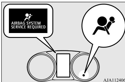
The system checks itself every time the ignition switch is turned to the "ON" position or the operation mode is put in ON. The SRS warning light will come on for several seconds and then go out. This is normal and means the system is working properly.
