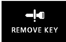
If the ignition switch is turned off and the driver's door is opened with the key in the ignition switch, the key reminder buzzer will sound intermittently to remind you to remove the key.
