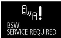
When the warning display appears, the BSW does not operate normally because there are some malfunctions in the system or the sensor. Have the vehicle inspected at an authorized Mitsubishi Motors dealer as soon as possible.
