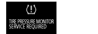
Each tire, including the spare (if provided), should be checked monthly when cold and inflated to the inflation pressure recommended by the vehicle manufacturer on the vehicle placard or tire inflation pressure label. (If your vehicle has tires of a different size than the size indicated on the vehicle placard or tire inflation pressure label, you should determine the proper tire inflation pressure for those tires.)
