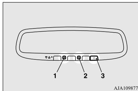
Normally, use the automatic mode. When the ignition switch is turned to the “ON” position or the operation mode is put in ON, the green indicator (1) illuminates and the reflection factor of the mirror is automatically changed.
