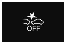
To turn on the FCM again, press and hold the FCM ON/OFF switch. The
