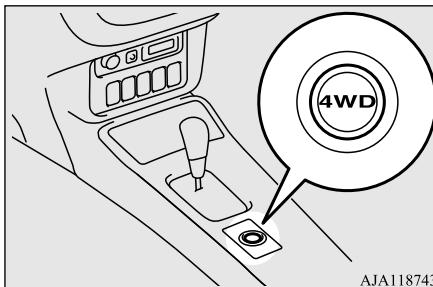
If you press the switch, you can change the drive mode in the order of 4WD ECO, 4WD AUTO, 4WD LOCK, 4WD ECO.
