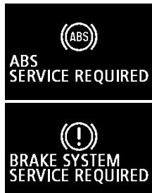
The anti-lock braking system and brake force distribution function may not work, so hard braking could make the vehicle unstable. Avoid hard braking and high-speed driving. Stop the vehicle in a safe place and contact an authorized Mitsubishi Motors dealer or repair facility of your choice.
