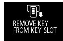
If the operation mode is in OFF and the driver's door is opened with the F.A.S.T.-key in the key slot, a warning is issued with the warning display and the buzzer buzzing for approximately 3 seconds to remind you to remove the key.
