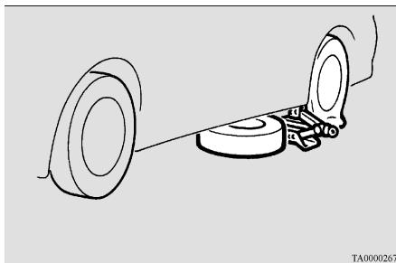
3. Rotate the jack by hand until the flange portion (B) fits in the groove (C) at the top of the jack.
