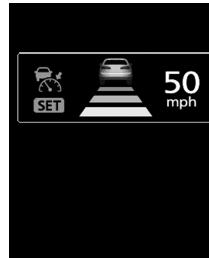
When the front vehicle stops, the ACC will automatically apply the brakes to stop your vehicle.
