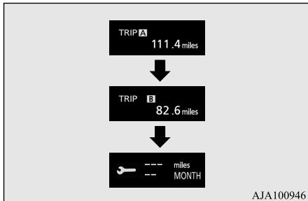
2. Press and hold the multi information display switch (for about 2 seconds or more) to display “---” and make it flash. (If there is no operation for about 10 seconds with this indicator flashing, the display returns to the previous screen.)
