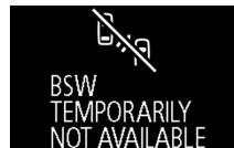
When the warning display appears, the sensor is temporarily not available for some reason such as the environmental condition or increase of the sensor temperature. When the warning display does not disappear after waiting for a while, contact an authorized Mitsubishi Motors dealer.
