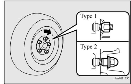
7. Turn the wheel nut clockwise by hand to initially tighten them.
