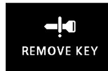
If the ignition switch is turned off and the driver's door is opened with the key in the ignition switch, the key reminder buzzer will sound intermittently to remind you to remove the key.
