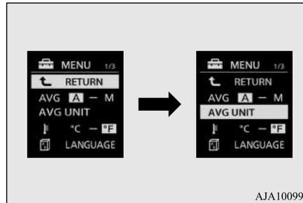
3. Press and hold the multi information display switch (for about 2 seconds or more) to display “AVG UNIT” (fuel consumption display unit setting).
