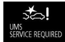
If the Ultrasonic misacceleration Mitigation System detects a malfunction in the system, the Ultrasonic misacceleration Mitigation System will not operate normally and this message is displayed.
