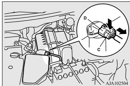
3. Unclamp the cover. Open up the top of the cover and take out the air cleaner filter.
