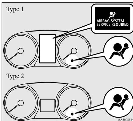
The system checks itself every time the ignition switch is turned to the "ON" position or the operation mode is put in ON. The SRS warning light will come on for several sec-
