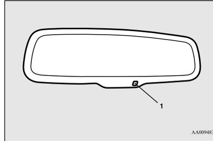
Normally, use the automatic mode. When the ignition switch is turned to the "ON" position or the operation mode is put in ON, the reflection factor of the mirror is automatically changed.
