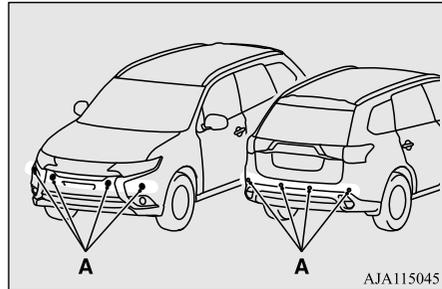
When the Ultrasonic misacceleration Mitigation System operates, the warning display will appear on the information screen of the multi information display, and a buzzer will sound intermittently.
