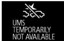
This display will appear if more than one sensor is temporarily not available for some reason such as an environmental condition. This can typically occur when the sensor is heated. When the radar sensor performance returns, the message will disappear and the system will resume operation.
