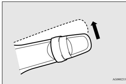
The wipers will operate once if the lever is moved to the “AUTO” position and the knob (C) is turned in the “+” direction when the ignition switch or the operation mode is in ON.
