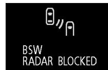
When the warning display appears, the radar sensor cannot detect a vehicle traveling side by side or an approaching vehicle, because foreign objects, such as dirt, snow or ice, adhere to the bumper surface around the sensor.
