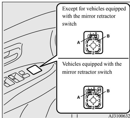
Press the switch (B) to adjust the mirror position.
