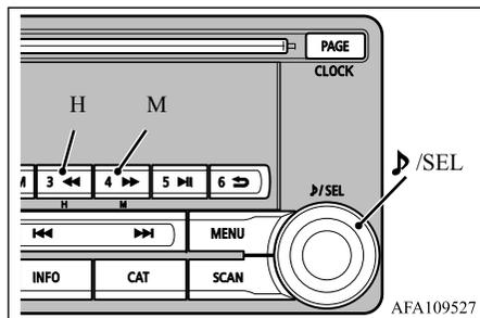
1. Select “YES” at the “Adjust time” screen, and press the **▶/SEL** key.
