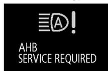
[When the sensor is malfunctioning]
