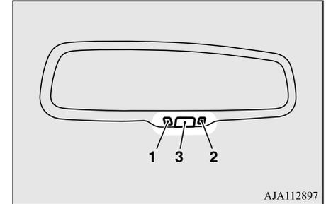
Normally, use the automatic mode. When the ignition switch is turned to the "ON" position or the operation mode is put in ON, the green indicator (1) illuminates and the reflection factor of the mirror is automatically changed.
