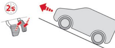
**Facing uphill, with the vehicle stationary, the vehicle is held for a short time when the driver releases the brake pedal:**
