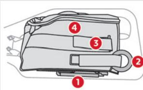
The space inside the passenger footwell is narrow. In order to be able to close the hatch, store the tools in their initial locations: chock **1** outside the bag, removable eye **2** on top of the bag with the buckle facing outwards, Torx key **3** on top of the bag, 12 V compressor with sealant cartridge **4** inside the bag.
