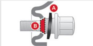
If the vehicle is fitted with alloy wheels, the washers A do not make contact with the steel spare wheel. The wheel is held in place by the conical contact surface B of each bolt.
