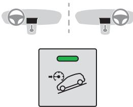
► To select the system, at speeds below 31 mph (50 km/h), press this button until its lamp lights up; this indicator lamp appears in green on the instrument panel.
