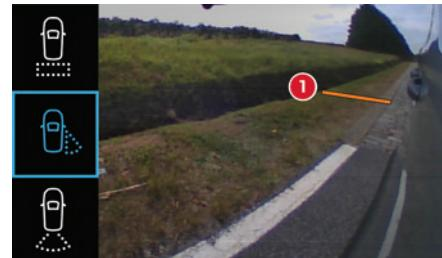
– **Passenger side view:** shows the area at the passenger side of the vehicle.
