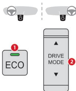
1. Pressing the control activates **Eco** mode. The indicator lamp comes on. (Petrol or Diesel)
