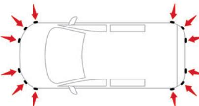
This system detects and signals the proximity of obstacles (e.g. pedestrian, vehicle, tree, barrier) using sensors located in the bumper.
