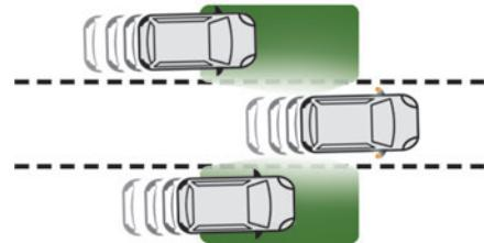
This system warns the driver of a potential danger posed by the presence of another vehicle (car, lorry, motorcycle) in the vehicle's blind spots (areas hidden from the driver's field of vision) using sensors located on the sides of the bumpers.
