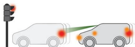
This function, also called automatic emergency braking, intervenes following the alerts if the driver does not react quickly enough and does not operate the vehicle's brakes.
