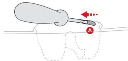
► From inside the vehicle, insert a small screwdriver into hole **A** on the lock to unlock the tailgate.
