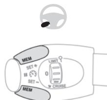
With this button, you can select a memorised speed setting to use with the speed limiter or the programmable cruise control. For more information on the **Speed limiter** or **Programmable cruise control**, refer to the corresponding section.
