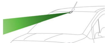
The vehicle has a camera located at the top of the windscreen.
