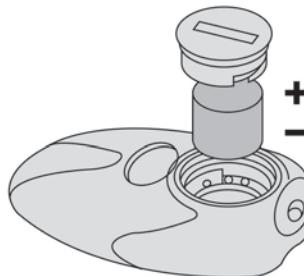
► Use a coin to unscrew the cap and replace the battery.
