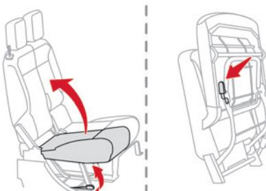
► Lift the yellow crank at the base of the seat to unlock and lift the assembly into folded position (seat raised against the backrest) until it locks. This position allows the transport of high loads inside the cab.
