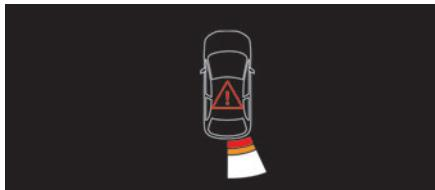
This supplements the audible signal, without taking account of the vehicle's trajectory, by displaying bars on the screen whose location represents the distance between the obstacle and the vehicle (white: more distant, orange: close, red: very close).
