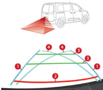
The blue lines 1 represent the general direction of the vehicle (the gap corresponds to the width of your vehicle with the mirrors).
