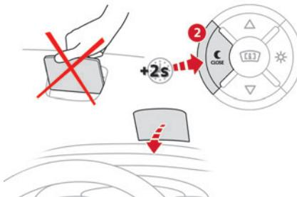
► Press and hold button 2 to deactivate the system and retract the projection blade. The state of the system is saved when the engine is switched off and restored on restarting.
