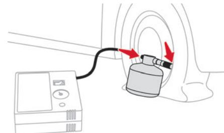
▶ Connect the pipe from the bottle of sealant to the valve of the tyre to be repaired and tighten firmly.
