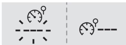
In the event of a malfunction, dashes are displayed flashing and then fixed instead of the speed setting.
