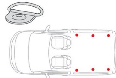
Use the stowing rings on the rear floor to secure loads.
