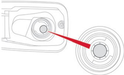
When a petrol filler nozzle is introduced into the fuel filler neck of a Diesel vehicle, it comes into contact with the flap. The system remains closed and prevents filling.
