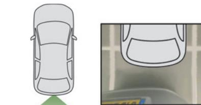
The camera records the vehicle's surroundings during the manoeuvre in order to create a view from above the rear of the vehicle in its near surroundings, allowing the vehicle to be manoeuvred around nearby obstacles.
