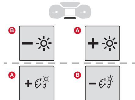
With the lamps on (not in the AUTO position), press button **A** to increase the brightness of the lighting, or button **B** to decrease it. Release the button when the desired brightness is reached.
