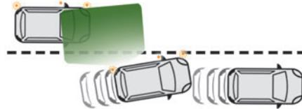
While the direction indicators are activated and for a few seconds after switching them off, the system considers that a change of trajectory is intentional and no correction is triggered during this period.
