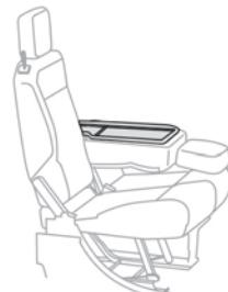
The backrest of the central seat of the bench seat tilts to form a work table, creating a mobile office (for use while stationary).
