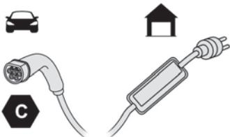
Identification label **C** on the charging connector (vehicle side).
