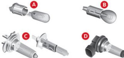
**Type A** All-glass bulb: pull gently as it is fitted by pressure.
