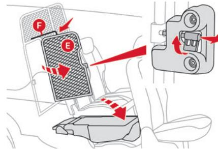
► Open/close the hatch **E** using the latch.
