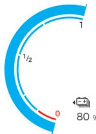
The traction battery's actual charge level and the remaining range are displayed continuously when the vehicle is started.
