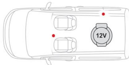
► Plug in a 12 V accessory (with a maximum rated power of 120 W) using a suitable adapter.
