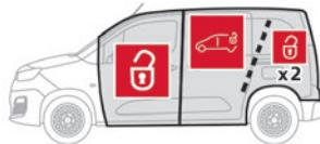
Selective unlocking unlocks either the **cabin** doors, or the doors of the **loading area** (side and rear).
