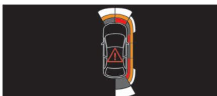
Using four additional sensors located on the sides of the bumpers, the system records the position of obstacles during the manoeuvre and indicates them when they are located alongside the vehicle.
