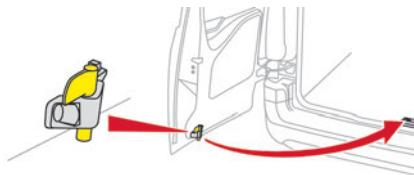
**i** It is possible to drive with the right-hand door open, to enable the transportation of long loads.
