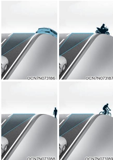
**Forward Collision-Avoidance Assist** may not detect a vehicle, a powered two-wheeler, a pedestrian or a cyclist in front of you while driving uphill or downhill adversely affecting the performance of the sensors.
