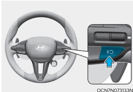
Press the **CII** switch to temporarily pause the set speed limit. The set speed limit will turn off but the Manual Speed Limit Assist (**LIMIT**) indicator will stay on.
