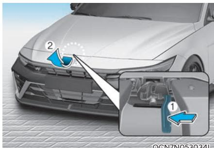
3. Go to the front of the vehicle, raise the hood slightly, push up the secondary hood release lever (1) inside of the hood center and lift the hood (2).
