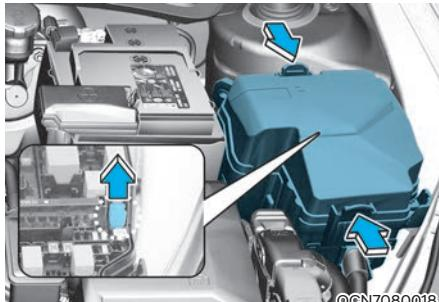
5. Pull the suspected fuse straight out. Use the removal tool provided in the engine compartment fuse panel.
