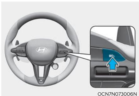
Press the Driving Assist (⌚) button to turn Cruise Control off. The Cruise (⌚CRUISE) indicator will go off. Always press the Driving Assist (⌚) button to turn Cruise Control off when not in use.
