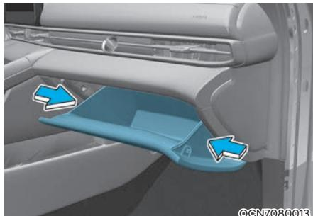
1. Push in both sides of the glove box as shown. This will ensure that the glove box stopper pins will get released from its holding location allowing the glove box to hang.
