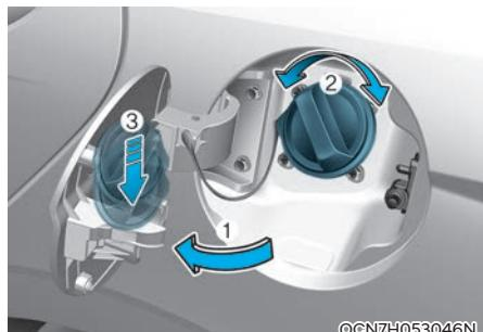
3. Pull the fuel filler door (1) out to fully open.
