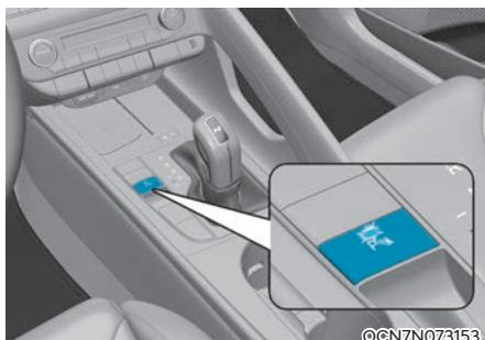
Press the Parking Safety button to turn on Forward/Reverse Parking Distance Warning. Press the button again to turn off the function.
