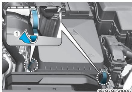
1. Loosen the air cleaner cover attaching clip (1) and open the cover.
