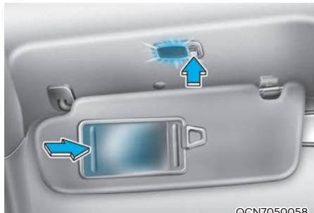
Push the switch to turn the light on or off.
