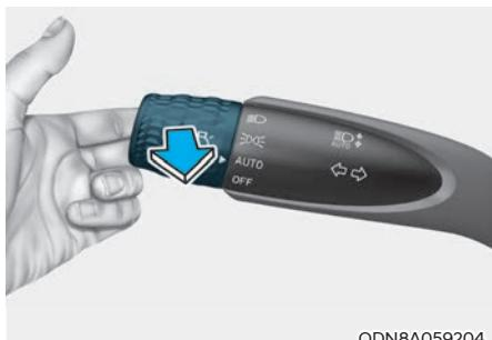
To flash the high beam headlight, pull the lever towards you, then release the lever. The high beams will remain ON as long as you hold the lever towards you.
