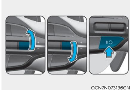
To resume Manual Speed Limit Assist after the function was paused, operate the **+, CII** switch.
