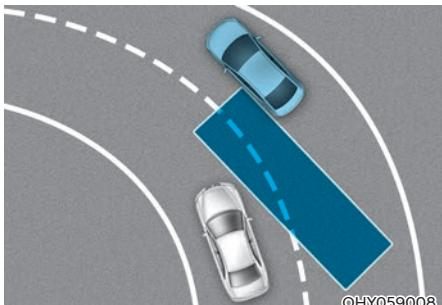
**Blind-Spot Collision-Avoidance Assist** may not operate properly when driving on a curved road. **Blind-Spot Collision-Avoidance Assist** may not detect the vehicle in the next lane.
