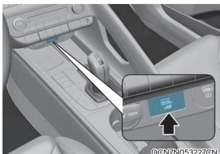
This is a convenient device that allows external sound devices such as MP3 and USB storage devices to be connected to the vehicle and played back through the vehicle infotainment system.
