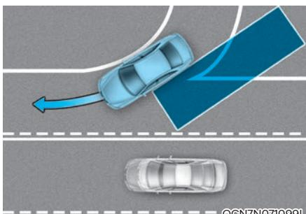
**Blind-Spot Collision-Avoidance Assist** may not operate properly when driving where the road merges or divides. **Blind-Spot Collision-Avoidance Assist** may not detect the vehicle in the next lane.
