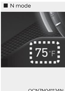
This gauge indicates the current outside air temperatures either in Celsius (°C) or Fahrenheit.
