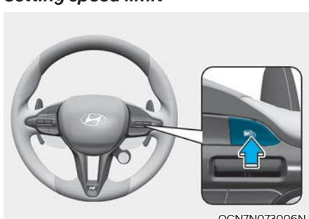
1. Press and hold Driving Assist (LIMIT) button at the desired speed. The Manual Speed Limit Assist (LIMIT) indicator will illuminate on the instrument cluster.
