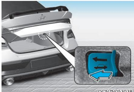
Your vehicle is equipped with an Emergency Trunk Safety Release lever located inside the trunk. When someone is inadvertently locked in the trunk, the trunk can be opened by moving the lever in the direction of the arrow and pushing the trunk open.
