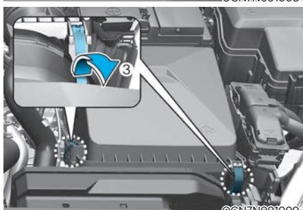
3. Insert the air cleaner cover in the hinge (2) and engage the clip (3) after closing the cover.
