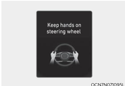
If the driver takes their hands off the steering wheel for several seconds, the 'Keep hands on the steering wheel' warning message will appear and an audible warning will sound in stages.
