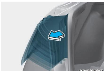
4. Remove the rear combination light assembly from the body of the vehicle.
