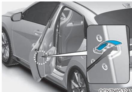
In case of emergency such as when the battery is discharged, the only way to lock the door(s) is with the mechanical key from the outside key hole.
