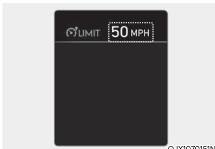
3. The set speed limit will be displayed on the instrument cluster. If you would like to drive over the preset speed limit, depress the accelerator pedal beyond the pressure point to activate the kickdown function.
