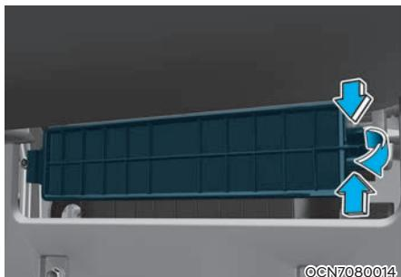
2. Remove the cabin air filter case while pressing the lock on the right side of the cover.
