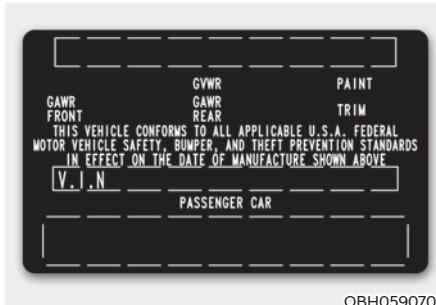
The certification label is located on the driver's door sill at the center pillar and shows the maximum allowable weight of the fully loaded vehicle. This is called the GVWR (Gross Vehicle Weight Rating). The GVWR includes the weight of the vehicle, all occupants, fuel and cargo. This label also tells you the maximum weight that can be supported by the front and rear axles, called Gross Axle Weight Rating (GAWR).
