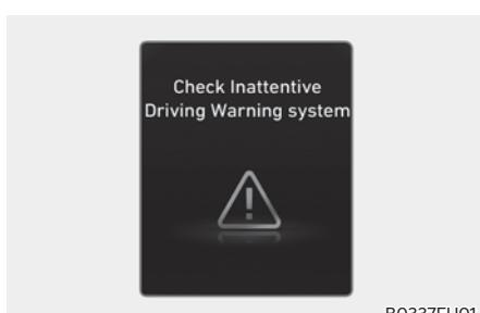
When Driver Attention Warning is not working properly, the 'Check Inattentive Driving Warning system' warning message will appear on the instrument cluster for several seconds, and the master (⚠) warning light and Driver Attention Warning light (⚠) will illuminate on the instrument cluster. If this occurs, have the vehicle inspected by an authorized HYUNDAI dealer.
