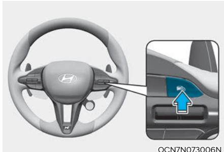
2. Press the Driving Assist (☞) button at the desired speed. The set speed and Cruise (☞CRUISE) indicator will illuminate on the instrument cluster.
