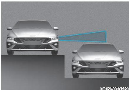
Blind-Spot Collision-Avoidance Assist may not operate properly when driving where the heights of the lanes are different. Blind-Spot Collision-Avoidance Assist may not detect the vehicle on a road with different lane heights (underpass joining section, grade separated intersections, etc.).
