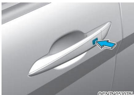
To lock the doors, press the button on the outside door handle while carrying the smart key with you or press the door lock button on the smart key.
