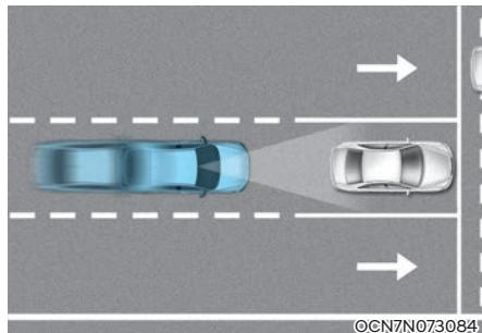
Forward Collision-Avoidance Assist helps detect a vehicle, a powered two-wheeler, a pedestrian, or a cyclist ahead on the road and may warn you of a possible collision with a warning message on the instrument cluster and a warning sound. Also, Forward Collision-Avoidance Assist may assist with braking your vehicle to help reduce collision speed or avoid a collision.
