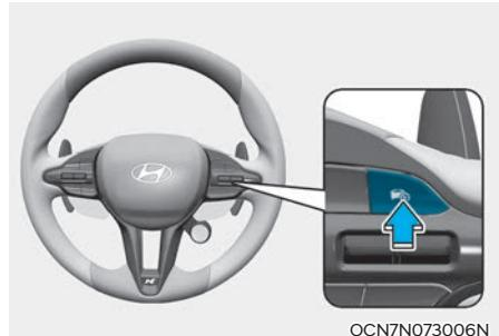
Press the Driving Assist (**DA**) button to turn Manual Speed Limit Assist off. The Manual Speed Limit Assist (**LIMIT**) indicator will go off.
