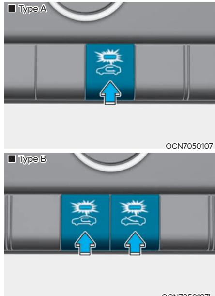
The air intake control button is used to select either Fresh mode (outside air) or Recirculation mode (cabin air).
