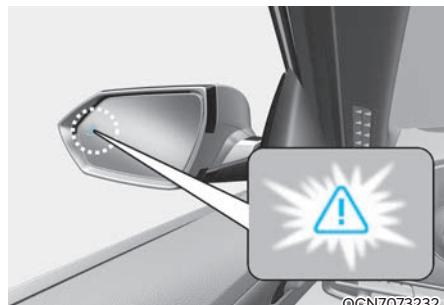
To warn the driver a vehicle is detected, the warning light on the side view mirror will illuminate.
