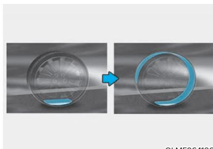
10. Immediately drive approximately 4~6 miles (7~10 km or, about 10min) to evenly distribute the sealant in the tire.
