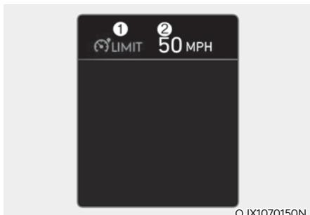
[1] : Manual Speed Limit Assist enabled indicator
