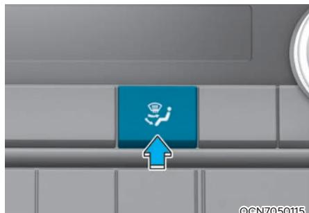
The mode selection switch controls the direction of the air flow through the ventilation system.
