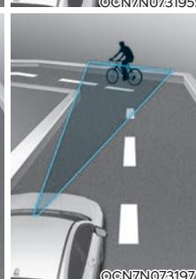
**Forward Collision-Avoidance Assist** may not detect other vehicles, powered two-wheelers, pedestrians or cyclists in front of you on curved roads that adversely affect the performance of the sensors. This may result in no warning or braking assist when necessary.
