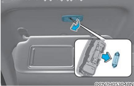
1. Using a flat-blade screwdriver, gently pry the lens or assembly from the interior light housing.
