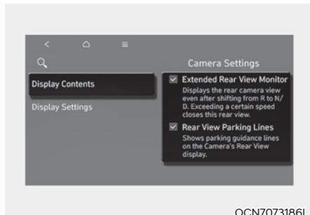
You can change Rear View Monitor **Display contents** by touching the setup icon (⚙) on the screen while Rear View Monitor is operating, or selecting **Setup > Vehicle > Driver Assistance > Parking Safety > Camera Settings** from the Settings menu in the infotainment system when the engine is on.
