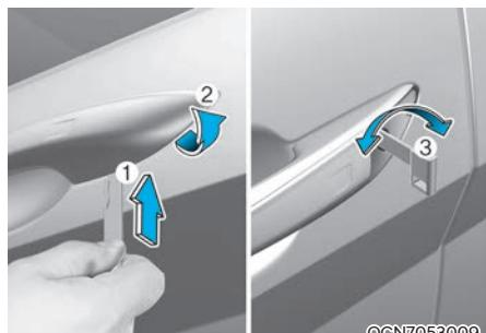
1. Press the lever located under the cover with mechanical key. (1)
