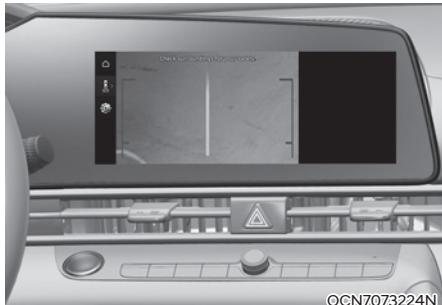
When you touch the
