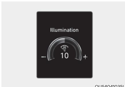
When the vehicle's parking lights or headlights are on, press the illumination control switch to adjust the brightness of the instrument panel illumination.
