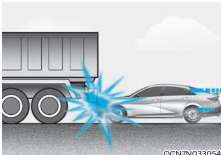
Just before impact, drivers often brake heavily. Such heavy braking lowers the front portion of the vehicle causing it to "ride" under a vehicle with a higher ground clearance. Air bags may not inflate in this "underride" situation because deceleration forces that are detected by sensors may be significantly reduced by such "underride" collisions.
