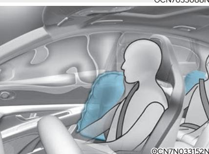
Your vehicle is equipped with a side air bag in each front and outboard second row seat. The purpose of the air bag is to provide the vehicle's additional protection than that offered by the seat belt alone.
