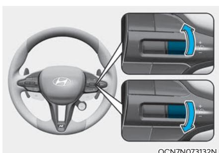
2. Push the + switch up or - switch down, and release it at the desired speed.
