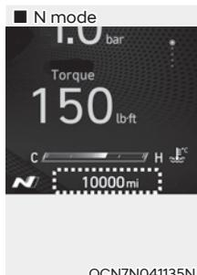
The odometer indicates the total distance that the vehicle has been driven and should be used to determine when periodic maintenance should be performed.
