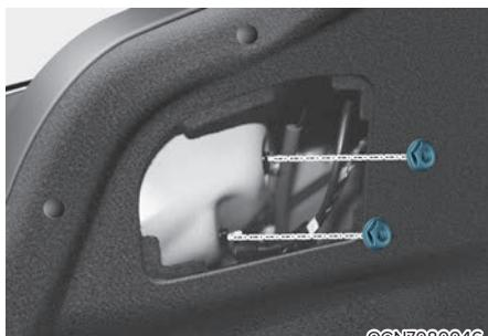
3. Loosen the assembly retaining nuts.
