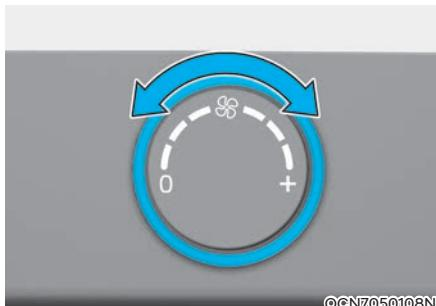
Turn the knob to the right to increase the fan speed and airflow. Turn the knob to the left to decrease fan speed and airflow.
