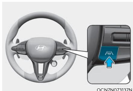
With the engine on, short press the Lane Driving Assist button located on the steering wheel to turn on Lane Following Assist. The white or green
