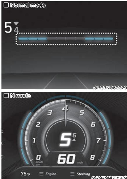
When engine is operating in a high RPM area, it is indicated on the cluster according to the corresponding engine RPM.
