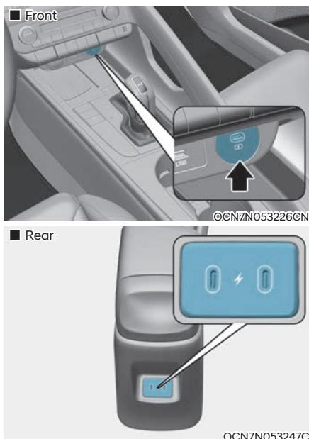
The USB charger is located inside the console box between the driver's seat and the front passenger's seat. Insert the USB charger into the USB port, and recharge a smartphone or a tablet PC.
