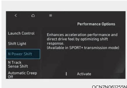
When the driver depresses the accelerator pedal fully (100%) in N mode for faster acceleration, it controls by (up-) shifting with minimal energy loss.
