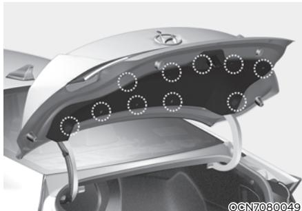
2. Loosen the retaining screw of the trunk lid cover and then remove the cover.
