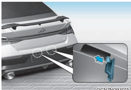
1. Using a flat-blade screwdriver gently pry the lens cover from the lamp housing.
