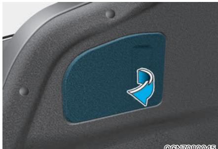
2. Remove the service cover by pulling out the service cover.
