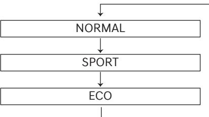
When NORMAL mode is selected, it is not displayed on the instrument cluster.
