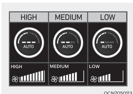
You can control the blower strength in three stages by pushing the AUTO button during automatic operation.
