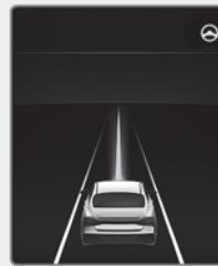
If the vehicle ahead and/or both lane markings are detected and your vehicle speed is below 120 mph (200 km/h), the green
