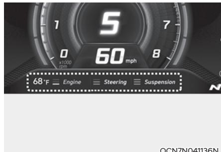
The main settings of CUSTOM mode is displayed at the bottom of the cluster. The CUSTOM mode can be set on the infotainment system.
