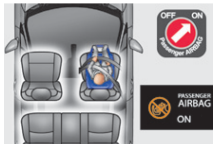
Passenger seat adjusted to the intermediate longitudinal and highest position.
