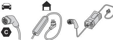
Identification label **C** on the charging connector (vehicle side).
