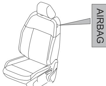
This system protects the driver and front passenger in the event of a serious side impact, limiting the risk of injury to the chest, between the hip and the shoulder.
