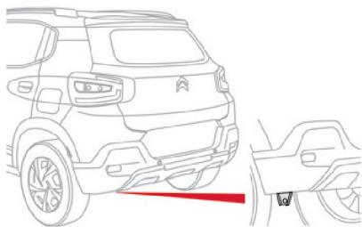
The rear towing bracket is provided under the rear bumper, on the left side of the vehicle.
