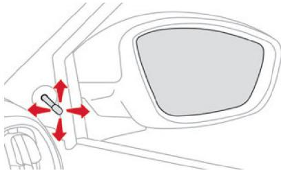
Move the lever in any direction to adjust it. If the mirror unit has come out of its initial position, with the vehicle stationary, push it back into place manually or use the control. There is no risk of breakage, even in frosty weather.
