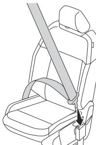
To fasten the seat belt, pull the webbing and insert the tongue into the buckle.
