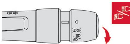
Turn and align the selection ring to switch between dipped and main beam headlamps. In the lighting off and sidelamps modes, the driver can switch on the main beam headlamps temporarily ("headlamp flash") by pulling up the stalk.
