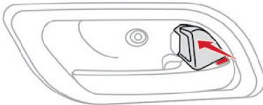
► Push/pull this knob located on the driver's door handle to lock/unlock the doors from inside the vehicle.
