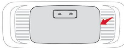
Using a thin, flap tip screwdriver, unclip the entire console surrounding the courtesy light.
