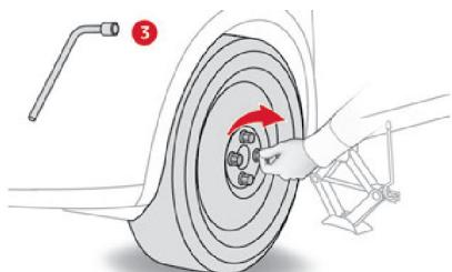
Tighten the bolts using the wheel wrench 3 only.
