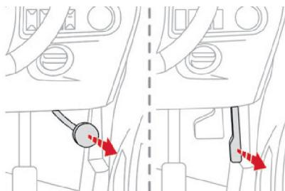
Pull the release lever located below the steering wheel towards you.
