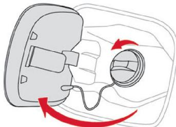
Turn the filler cap to the left and remove it.
