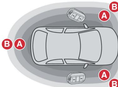
This system allows the auto-locking of the vehicle, while carrying the electronic key away/out of the recognition zone **B**.
