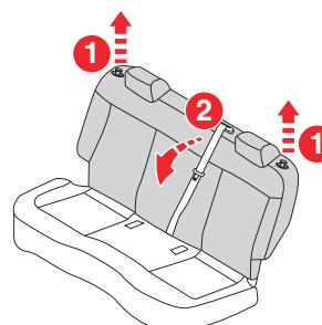
Pull the Latch knob 1 up and fold the backrest 2 inwards to increase boot space.
