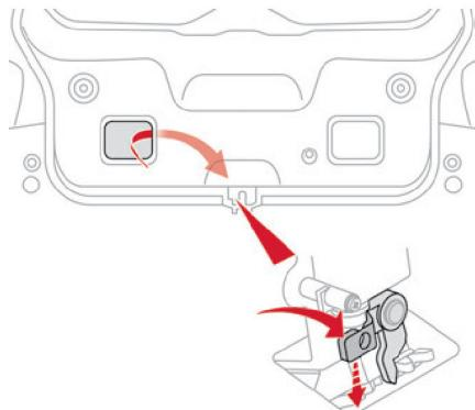
Fold the rear seats to gain access to the lock from inside the boot.
