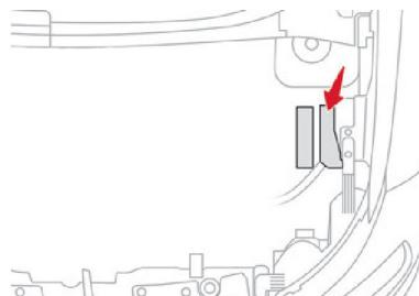
The puller is located inside the engine fuse box. Open the bonnet.
