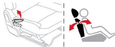
To adjust the seatback, lift the lever located on the outboard side of the seat, lean back to the desired position and release the lever. To return the seatback, lift the lever, lean forward and release the lever.
