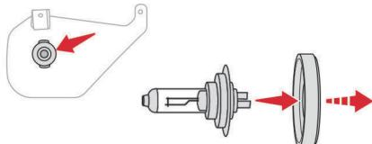
Remove the protective cover by pulling on the tab.
