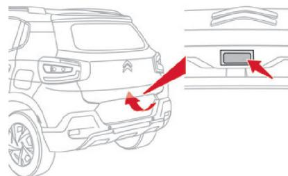
Press the switch located on the tailgate bottom to open the tailgate.
