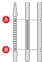
Reinsert the dipstick and push fully down, then pull it out again to visually check the oil level: the correct level is between marks **A (max)** and **B (min)**.
