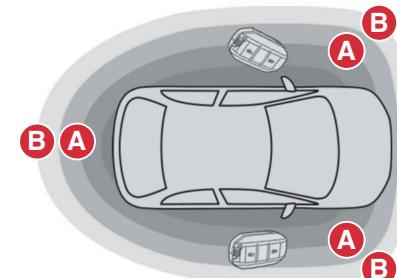
The system allows the unlocking and starting of the vehicle, while carrying the electronic key on your person in the recognition zone **A**.
