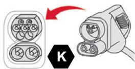
► Follow the instructions for use of the fast public charger and connect the cable from the fast public charger to the vehicle's connector.
