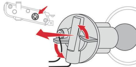
Turn the bulb holder a eighth of a turn anticlockwise and remove it.
