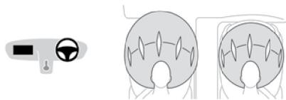
This system protects the driver and front passenger in the event of a serious front impact, in order to limit the risk of head and chest injuries.
