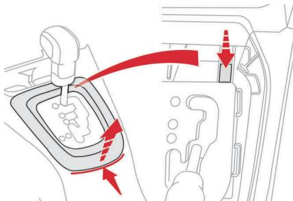
In this case, the following steps will allow you to take manually the gear selector out of mode **P**:
