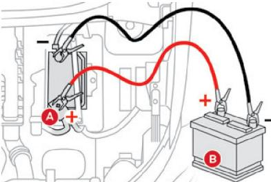
Lift the cover on the (+) terminal, if the vehicle has one.
