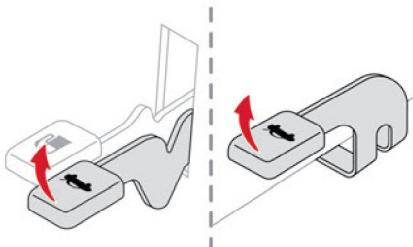
Lift the opening lever located besides the driver's seat to open the tailgate.
