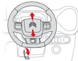
When stationary, hold the steering wheel on one hand and pull the control lever to release the steering wheel.
