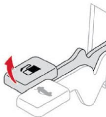
Lift the fuel filler flap lever, located on the floor beside the driver's seat, to open the flap.
