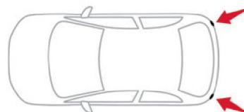
Using sensors located in the bumper, this system signals the proximity of obstacles (e.g. pedestrian, vehicle, tree, barrier) present in their field of detection.
