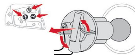
Turn the bulb holder a eighth of a turn anticlockwise and remove it.
