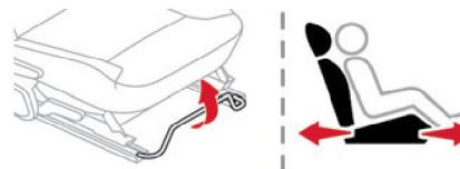
Raise the control bar and slide the seat forwards or backwards.
