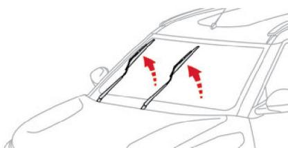
Within one minute after switching off the ignition, operate the wiper stalk to position the wiper blades vertically on the windscreens.
