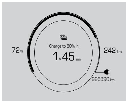
The traction battery's actual charge level is displayed continuously when the vehicle is started.
