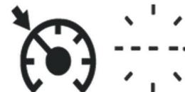
In the event of a malfunction, dashes are displayed flashing and then fixed instead of the speed setting.
