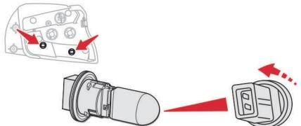
Turn the bulb holder a quarter of a turn and pull it out.
