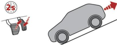
**Facing downhill, with the vehicle stationary and reverse gear engaged, the vehicle is held for a short time when the driver releases the brake pedal.**
