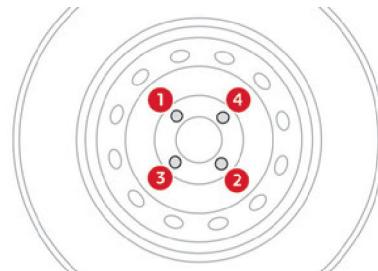
Loosen the nuts on the wheel in diagonal sequence. Do not remove wheel nuts.
