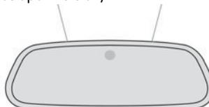
The electrochrome system uses a sensor that detects the level of exterior brightness and that coming from the rear of the vehicle, in order to automatically and gradually switch between day and night usage.
