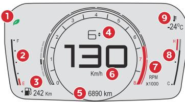
4. Gear engaged (manual gearbox)
