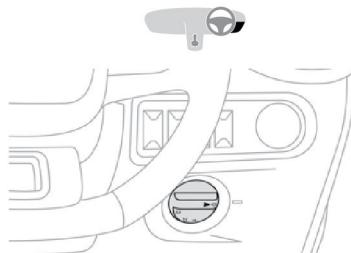
To avoid disturbing other road users, the height of the headlamp beams should be adjusted according to the load in the vehicle.
