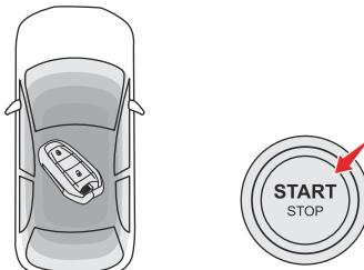
With the electronic key in the passenger compartment, pressing the "**START/STOP**" button, **without depressing any of the pedals**, allows the ignition to be switched on without starting the engine (the instrument panel and accessories such as the audio system and the lighting will come on).
