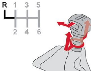
► Raise the ring under the knob and move the gear selector to the left, then forwards.
