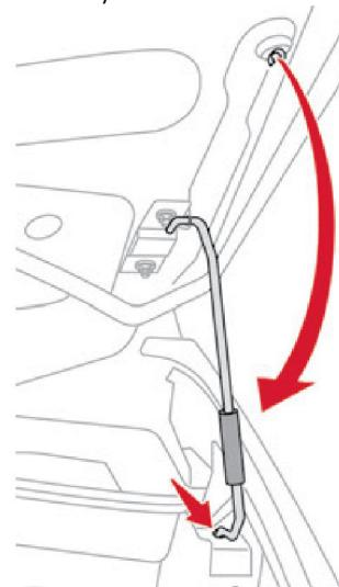
Unclip the stay from its housing and place it in the support slot to hold the bonnet open.
