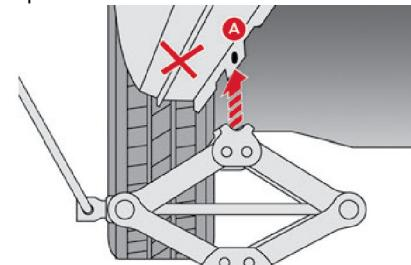
Extend jack **1** with the jack handle **2** and wheel wrench **3** until its head comes into contact with jacking point **A** or **B**; contact area **A** or **B** on the vehicle must be properly inserted into the central part of the head of the jack.
