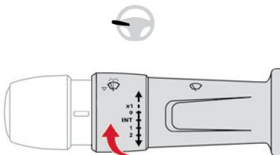
To select the wiping speed: raise or lower the stalk to the desired position.
