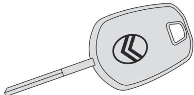
The key allows the central locking or unlocking of the vehicle using the door lock. It also allows the engine to be started or switched off.
