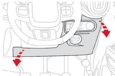
Unclip the cover by pulling at the top left, then right.
