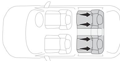
The mountings comprise three rings for each seat, indicated by a marking:
