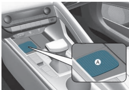
[A] Charging pad
