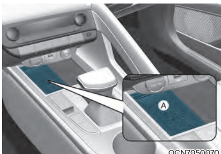
[A] : Wireless Charging Pad (In-vehicle Authentication Pad)
