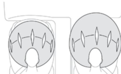
System which protects the driver and front passenger in the event of a serious front impact in order to limit the risk of injury to the head and thorax.
