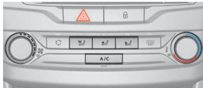
**i** If you put the air flow control in the **minimum** position (system off), the temperature is no longer controlled. However, a slight flow of air can still be felt, resulting from the movement of the vehicle.
