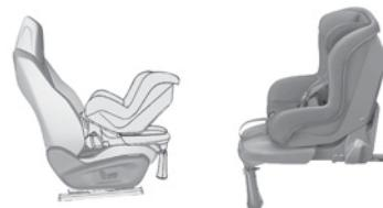
Installed rearward facing using an ISOFIX base which is attached to the anchorage rings **A**. The base has a support leg, adjustable for height, which sits on the vehicle's floor. This child seat can also be used forward facing. This seat can **not** be secured with a seat belt. We recommend that you use the seat in the rearward facing position up to the age of 3 years.
