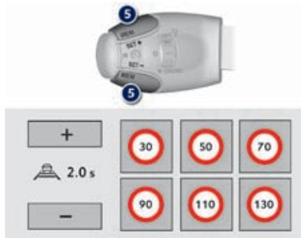
Press button 5, the six memorised speeds and the inter-vehicle time setting are displayed in the touch screen.
