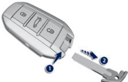
The integral key is used to lock and unlock the vehicle when the electronic key cannot operate:
