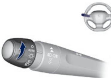
When a low level of ambient light is detected by a sunshine sensor, the number plate lamps, sidelamps and dipped beam headlamps are switched on automatically, without any action on the part of the driver. They can also come on if rain is detected, at the same time as automatic operation of the windscreens wipers. As soon as the brightness returns to a sufficient level or after the windscreens wipers are switched off, the lamps are switched off automatically.
