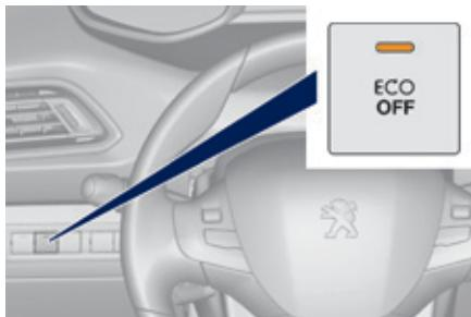
In the event of a fault with the system, this warning lamp comes on continuously.
