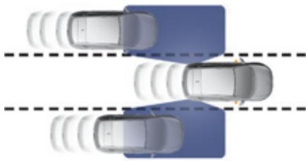
This driving assistance system warns the driver of the presence of another vehicle in the blind spot angle of their vehicle (areas masked from the driver's field of vision), as soon as this presents a potential danger.
