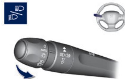
Pull the stalk to switch the lighting between dipped / main beam headlamps.
