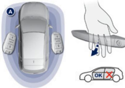
With the electronic key on your person and in the recognition zone A, pass your hand behind one of the front door handles to unlock the vehicle, then pull on the handle to open the door.
