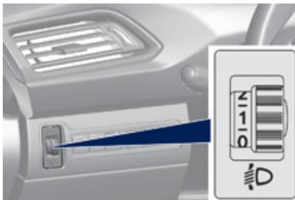
To avoid causing a nuisance to other road users, the beams of the halogen headlamps should be adjusted according to the load in the vehicle.
