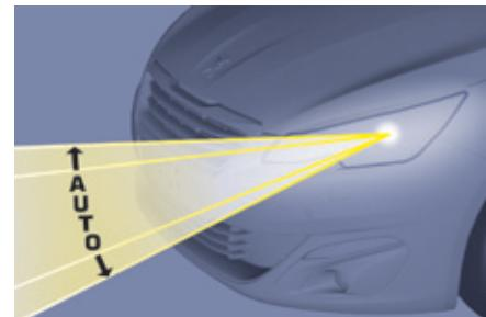
In order to avoid causing a nuisance to other road users, this system corrects the height of the "full LED" headlamps beam automatically, according to the load in the vehicle.
