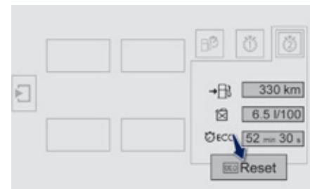
☞ When the desired trip is displayed, press the reset button or on the end of the wiper control stalk.
