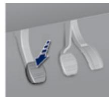
With a manual gearbox, place the gear lever in neutral then fully depress the clutch pedal.
