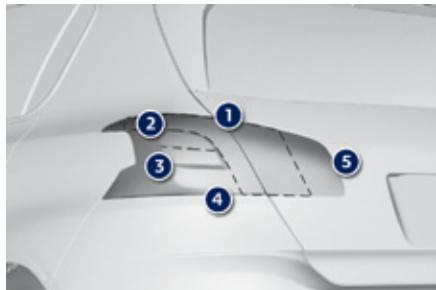
1. Sidelamps (light emitting diodes - LEDs).
