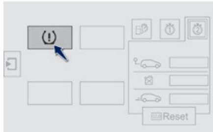
Reinitialisation of the system is done with the ignition on and the vehicle stationary.
