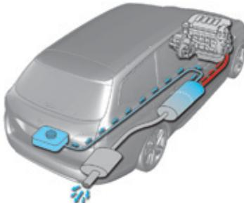
The AdBlue® additive is held in a special tank located under the boot at the rear of the vehicle. It has a capacity of 17 litres: this provides a driving range of about 12 500 miles (20 000 km), after which an alert is triggered warning you when the reserve remaining is enough for just 1 500 miles (2 400 km).
