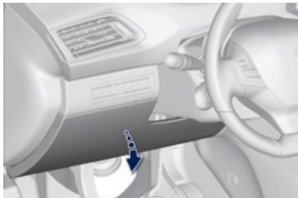
The fusebox is placed in the lower dashboard (left-hand side).
