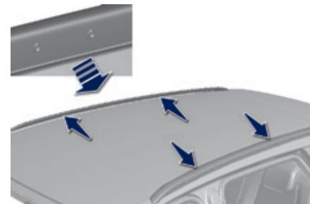
You must fit the transverse bars to the longitudinal bars at the fixing points indicated by engraved markings on the longitudinal bars.
