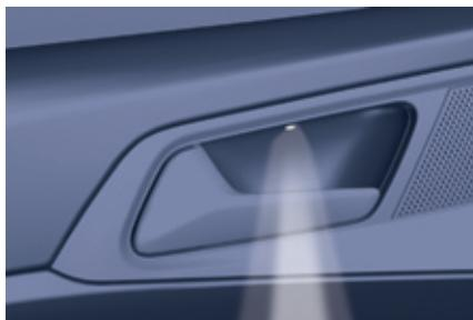
At night, the courtesy lamps and lighting for the interior opening controls on the front doors come on automatically when the sidelamps are switched on.
