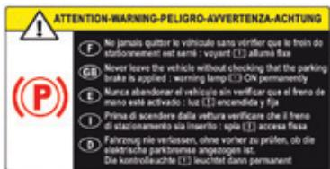
**i** Before leaving the vehicle, check that parking brake is applied: the indicator lamps in the instrument panel and the control lever must be on fixed, not flashing.
