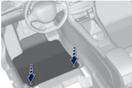
When fitting the mat for the first time, on the driver's side use only the fixings provided in the wallet attached.
