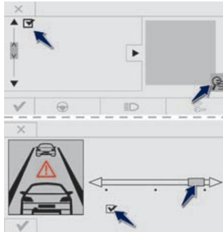
The emergency collision alert system can be activated or deactivated by the driver. From the secondary page of the "Driving assistance" menu:
