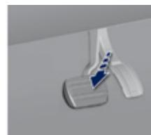
With an automatic gearbox, place the gear lever in position **N** or **P** then firmly press the brake pedal.
