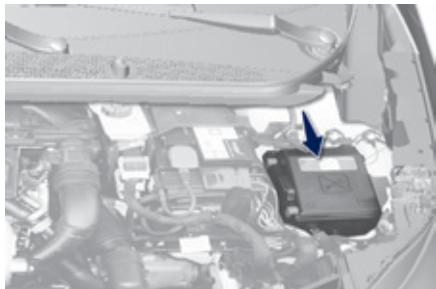
The fusebox is located in the engine compartment near the battery.
