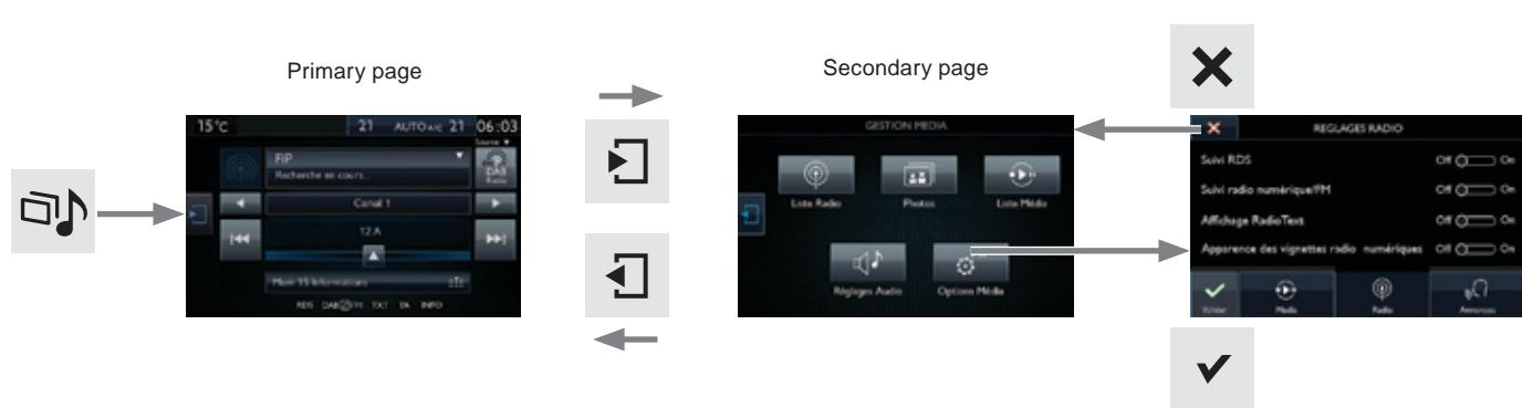
Shortcuts: using virtual buttons in the top band of the touch screen, it is possible to go directly to the choice of audio source, the list of stations (or titles depending on the source) or to temperature adjustment.
