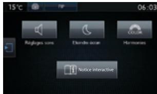
Adjust settings for audio (balance, ambience, ...), colour scheme, brightness of the instruments and controls, display (language, units, date, time, ...) and access the interactive help for the vehicle's main systems and warning lamps.
