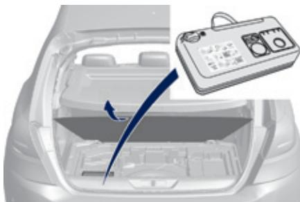
This kit is installed in the storage box, under the boot floor.
