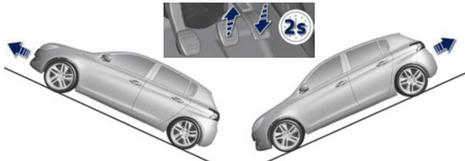
**On an ascending slope, with the vehicle stationary, the vehicle is held for a momentarily when you release the brake pedal:**
