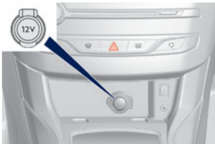
To connect a 12 V accessory (maximum power: 120 Watts), lift the cover and connect a suitable adaptor.
