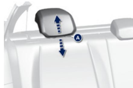
These have one position for use (up) and a stowed position (down). They can be removed and are interchangeable.
