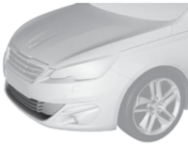
**i** The operation of the radar, located in the front bumper, may be disturbed in certain weather conditions, for example: with accumulations of snow, ice, mud, ...
