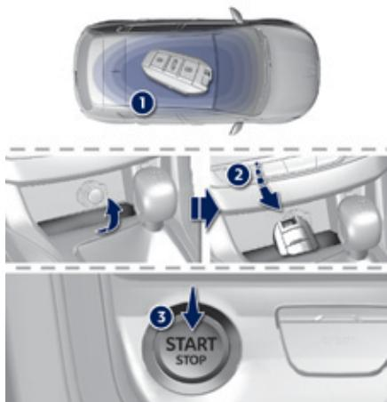
When the electronic key is in the recognition zone and your vehicle does not start after pressing the "START/STOP" button:
