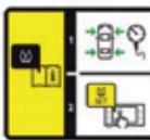
It is necessary to reinitialise the system every time one or more tyre pressures are adjusted, and after changing one or more wheels. A label attached to the middle pillar, driver's side, gives a reminder of this.
