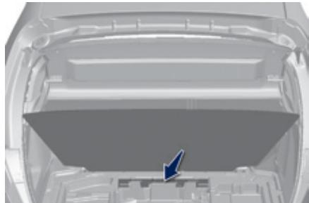
The towing eye is installed in the boot under the floor.
