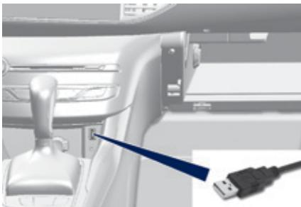
It allows the connection of a portable device, such as a digital audio player of the iPod® type or a USB memory stick.
