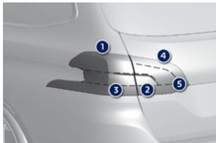
1. Sidelamps (light emitting diodes - LEDs).
