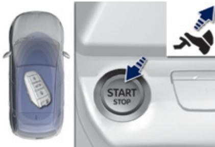
Pressing the "START/STOP" button, with no action on the pedals, allows the ignition to be switched on and so activate the ancillary equipment.
