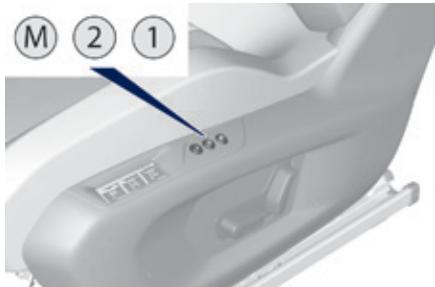
System which registers the electrical settings of the driver's seat and the door mirrors. You can store and recall two positions using the buttons on the side of the driver's seat.
