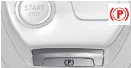
The system allows the application of the parking brake on switching off the engine and release as the vehicle moves off.
