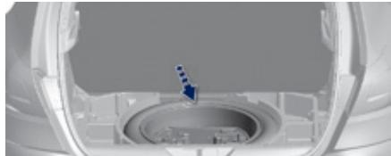
The spare wheel is located in the boot under the floor.
