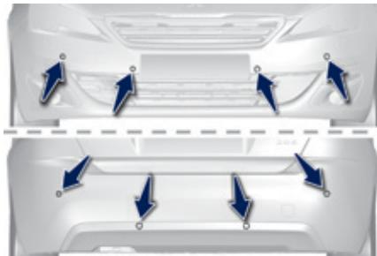
This system indicates the proximity of an obstacle (person, vehicle, tree, gate, etc.) which comes within the field of detection of sensors located in the bumper.
