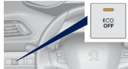
At any time, press the "ECO OFF" switch to deactivate the system.
