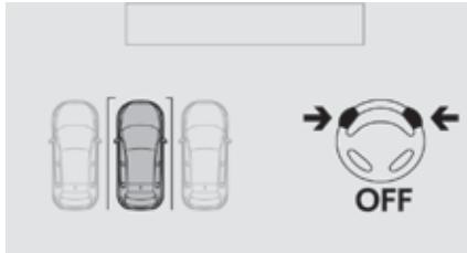
At the end of the manoeuvre, the operating indicator lamp goes off in the instrument panel, accompanied by a message and an audible signal.
