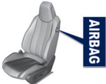
System which protects the driver and front passenger in the event of a serious side impact in order to limit the risk of injury to the chest, between the hip and the shoulder.
