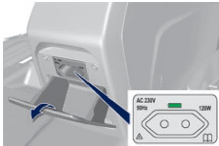
A 230 V / 50 Hz socket (maximum power: 120 W) is fitted in the rear storage box. This socket works with the engine running, as well as in STOP mode with Stop & Start.
