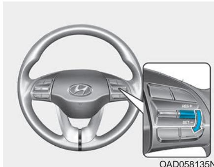
3. Push the toggle switch down (SET-). The Set Speed and Vehicle-to-Vehicle Distance on the LCD display will illuminate.
