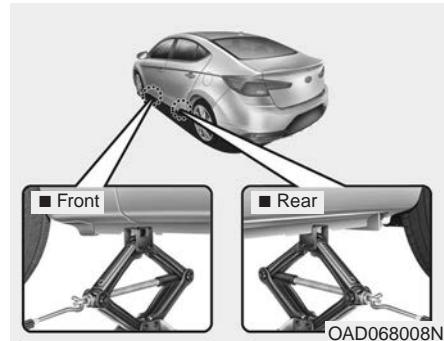
7. Place the jack at the designated jacking position under the frame closest to the tire you are changing. The jacking positions are plates welded to the frame with two notches. Never jack any other position or part of the vehicle. Doing so may damage the side seal molding or other parts of the vehicle.
