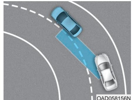
The system may not operate properly when driving on a curved road. In certain instances, the system may recognize a vehicle in the same lane.
