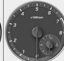
The tachometer indicates the approximate number of engine revolutions per minute (rpm).
