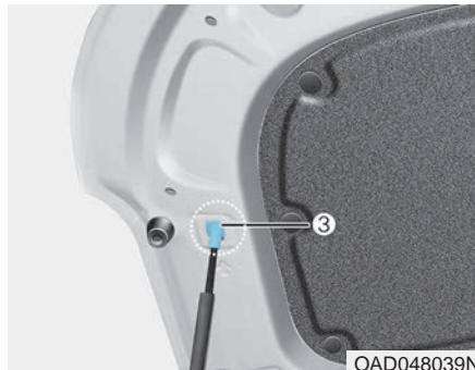
4. Pull out the support rod and prop the hood open with the support rod (3).
