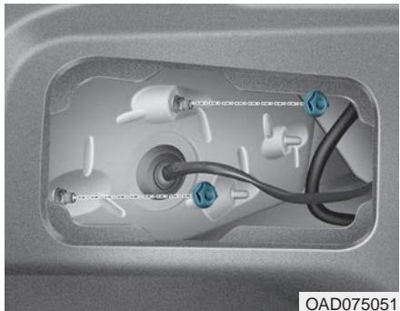
3. Loosen the assembly retaining nuts.
