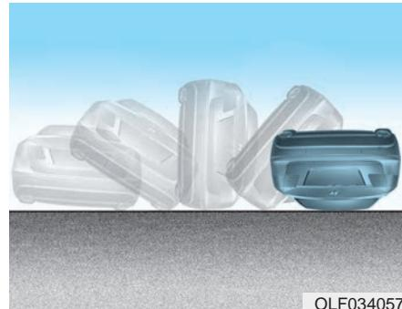
Front air bags may not inflate in rollover accidents because air bag deployment could not provide protection to the occupants. However, side and curtain air bags may inflate when the vehicle is rolled over by a side impact collision.
