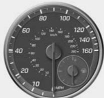
The speedometer indicates the speed of the vehicle and is calibrated in miles per hour (mph) and/or kilometers per hour (km/h).
