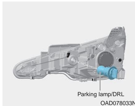
5. Install a new bulb by inserting it into the socket and rotating it until it locks into place.
