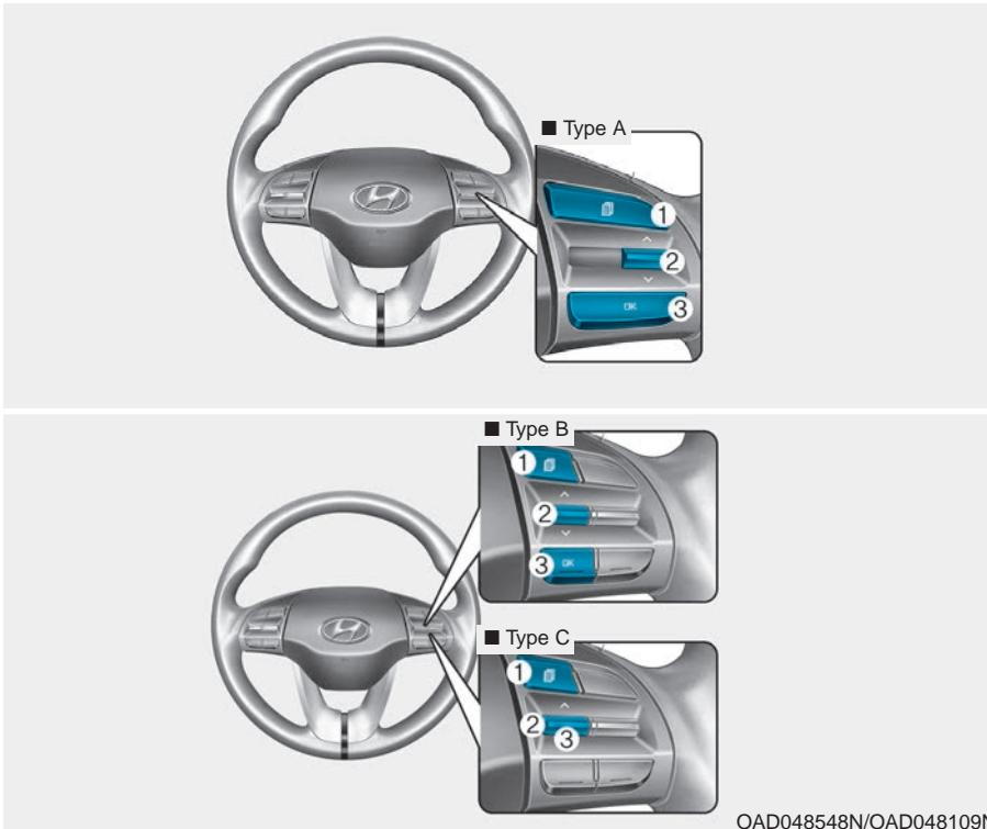
The LCD display modes can be changed by using the control buttons on the steering wheel.
