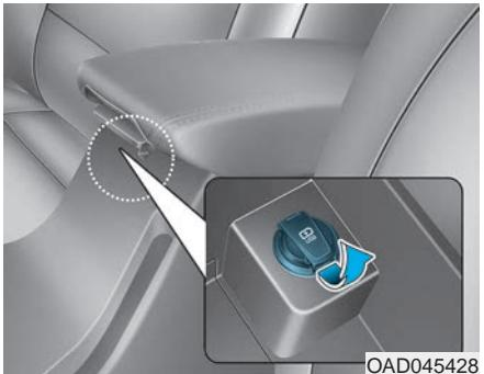
The USB charger is located inside the console box between the driver's seat and the front passenger's seat.
