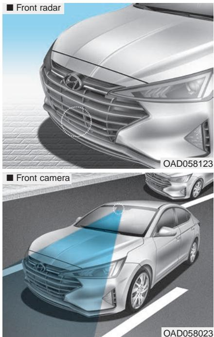
In order for the FCA system to operate properly, always make sure the sensor cover or sensor is clean and free of dirt, snow, and debris.
