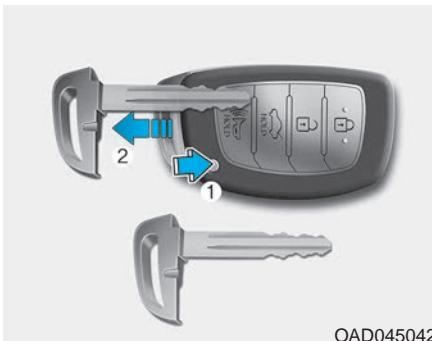
Press and hold the release button (1) and remove the mechanical key (2). Insert the mechanical key into the key hole on the door.
