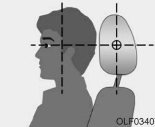
Adjust the head restraints so the middle of the head restraints is at the same height as the height of the top of the eyes.
