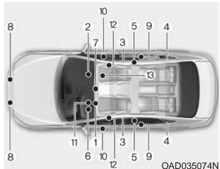
The SRS consists of the following components:
