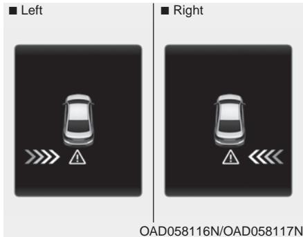
If the vehicle detected by the sensors approaches from the rear left/right side of your vehicle, the warning chime will sound, the warning light on the outside rearview mirror will blink and a warning will appear on the LCD display. If the rear view monitor system is in activation, a warning will also appear on the audio or AVN screen.
