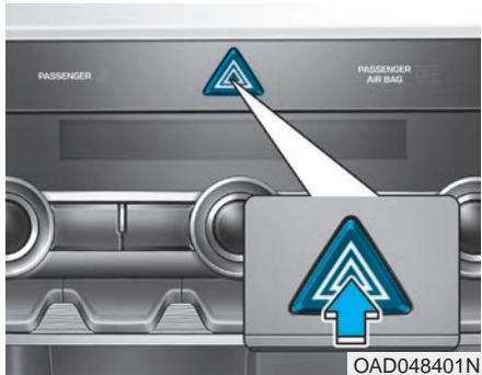
To turn the hazard warning flasher on or off, press the hazard warning flasher button. The button is located in the center fascia panel. Both the left and right turn signal lights will flash simultaneously.
