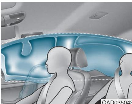
Curtain air bags are located along both sides of the roof rails above the front and rear doors.
