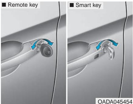
If you lock the driver's door with a mechanical key, all vehicle doors will lock. If you unlock the driver's door with a mechanical key, the driver's door will unlock and the passenger doors will unlock according to the current two press unlock setting.
