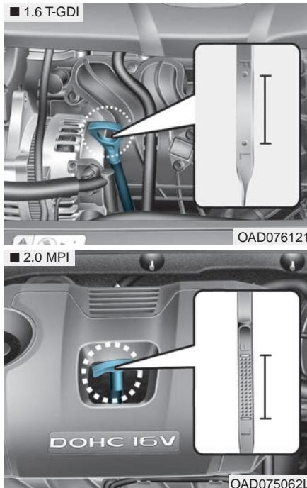
6. Pull the dipstick out again and check the level. The level should be between F and L.
