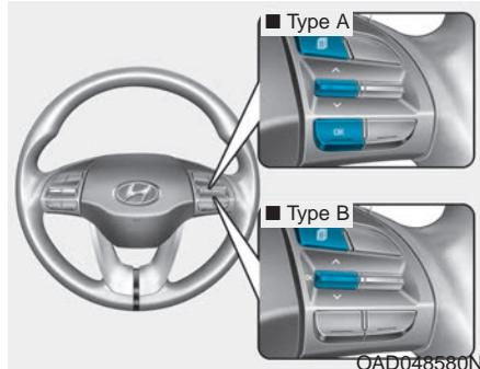
To change the trip mode, toggle the UP/DOWN arrow switch "▲, ▽" on the steering wheel.
