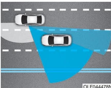
The Blind Spot Mirror (BSM) is a supplemental mirror that reduces the driver's blind spot by showing the rear side area of the vehicle. The blind spot mirror is equipped on the left-hand side view mirror.
