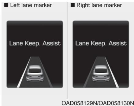
1. A visual warning appears on the cluster LCD display. Either the left lane marker or the right lane marker in the cluster LCD display will blink depending on which direction the vehicle is veering. Also, a warning sound will be heard.
