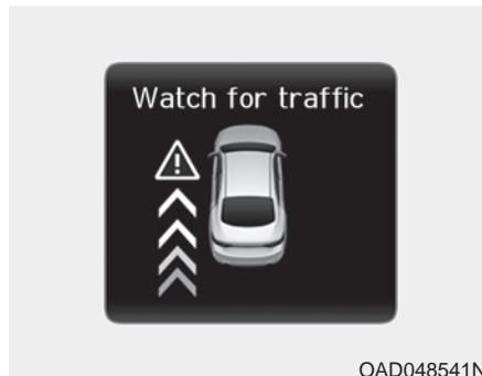
Once the system decides it is dangerous for a passenger to open a car door by sensing the approaching of a car from behind when the person is opening the door, the warning message "Watch for traffic" appears and the alarming sound will continue for five seconds.
