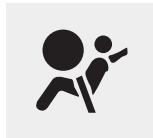
The SRS (Supplemental Restraint System) air bag warning light on the instrument panel displays the air bag symbol depicted in the illustration. The system checks the air bag electrical system for malfunctions. The light indicates that there is a potential malfunction with your air bag system, which could include your side and curtain air bags used for rollover protection.
