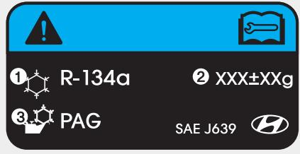
The actual Air Conditioning refrigerant label in the vehicle may differ from the illustration.
