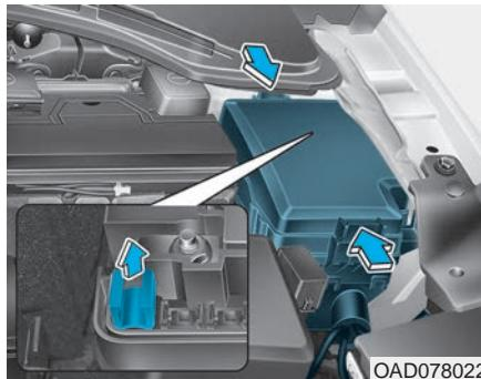
5. Pull the suspected fuse straight out. Use the removal tool provided in the engine compartment fuse panel.
