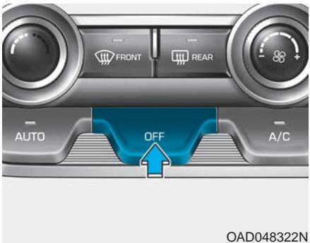
Push the OFF button of the front to turn off the air climate control system. You can still operate the mode and air intake buttons as long as the ignition switch is in the ON position.
