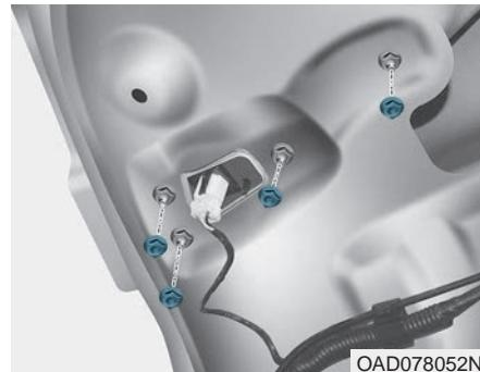
3. Disconnect the connector and then remove the nuts by turning the nuts counter clockwise.
