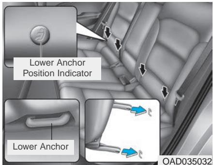
The lower anchor position indicator symbols are located on the left and right rear seat backs to identify the position of the lower anchors in your vehicle (see arrows in illustration).
