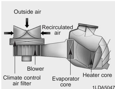
This filter is installed behind the glove box. It filters the dust or other pollutants that enter the vehicle through the heating and air conditioning system.
