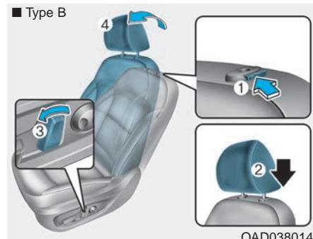
1. Put the head restraint poles (2) into the holes while pressing the release button (1).
