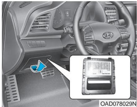
Inside the fuse/relay box cover, you can find the fuse/relay label describing fuse/relay name and capacity.
