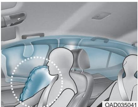
Your vehicle is equipped with a side air bag in each front seat.
