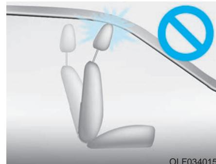
If you recline the seatback towards the front with the head restraint and seat cushion raised, the head restraint may come in contact with the sunvisor or other parts of the vehicle.
