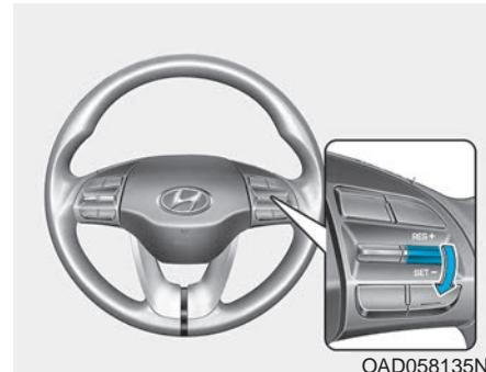
3. Push the toggle switch down (SET-), and release it. The SET indicator or set speed on the LCD display will illuminate.
