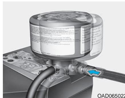
4. Insert the sealant bottle into the housing (4) of the compressor so that the bottle is upright.
