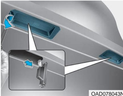
1. Remove the cover by pressing it as direction of the arrows.
