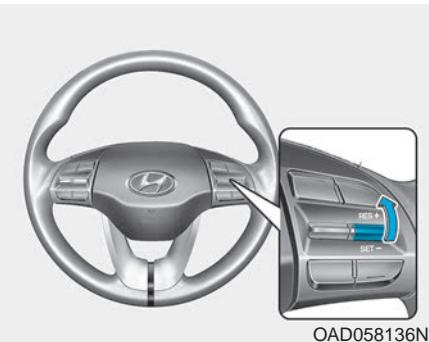
Push the toggle switch up (RES+). If the vehicle speed is over 20 mph (30 km/h), the vehicle will resume the preset speed.
