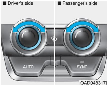
Turn the knob to the right to increase the fan speed temperature and airflow. Turn the knob to the left to decrease fan temperature.
