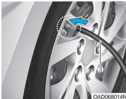
3. Connect the other end of the filling hose (3) directly into the valve.
