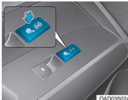
Each time you push the switch, the temperature setting of the seat is changed as follows :
