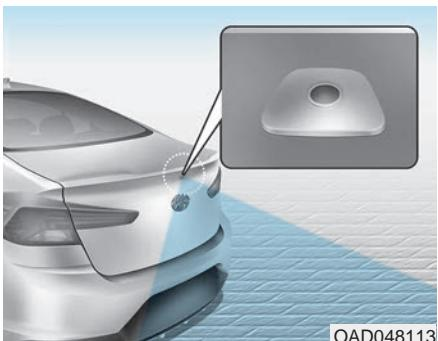
The Rear View Monitor will activate when the engine is running and the shift lever is in the R (Reverse) position.
