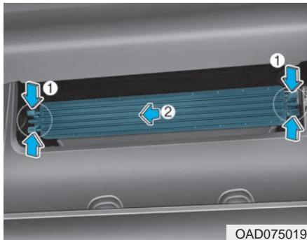
3. Press and hold the lock (1) on both sides of the cover.
