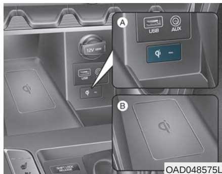
[A]: Indicator light, [B]: Charging pad
