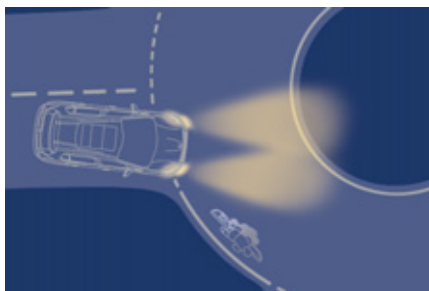
without cornering lighting
