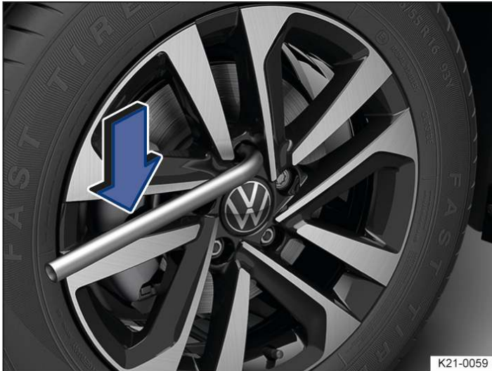
Fig. 1 Loosening wheel bolts.
