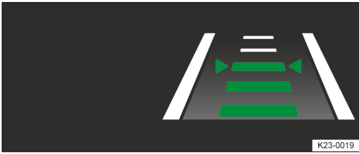
Fig. 1 In the head-up display: set distance for control (illustration).
