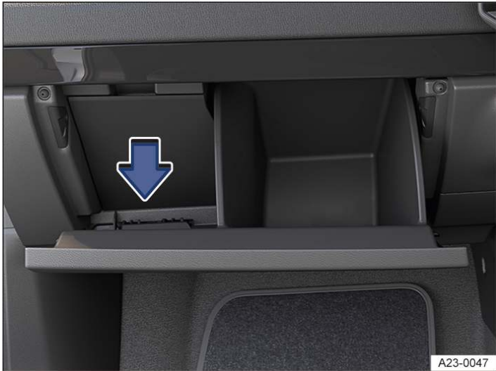
Fig. 2 On the front passenger side: fuse box cover in the dash panel (right-hand drive vehicle)
