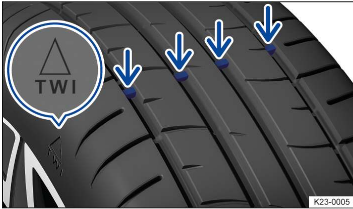
Fig. 1 In the tread grooves: tread wear indicator.
