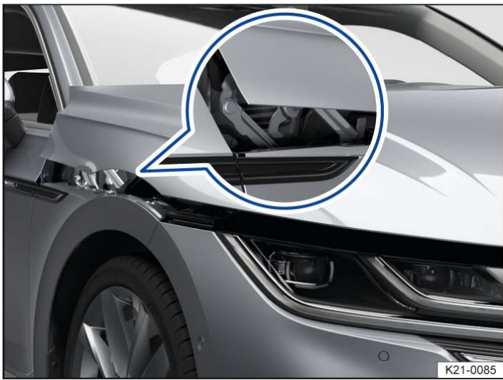
Fig. 1 Triggered re-active bonnet (illustration).
