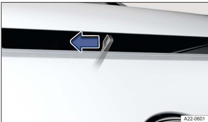
Fig. 2 On the bonnet: control lever. (illustration)
