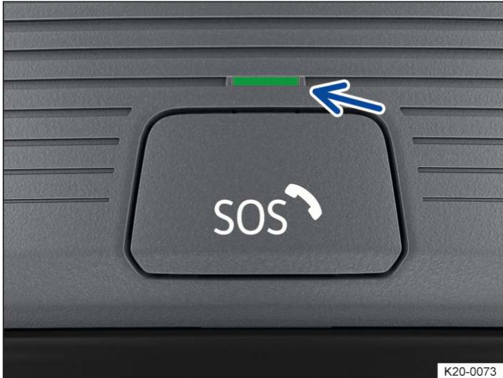
Fig. 1 In the roof console: button for legally required eCall Emergency System (behind button cover) and indicator lamp.
