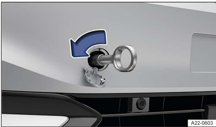
Fig. 2 In the front bumper on the right: screwing in the towing eye.
