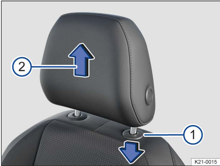
Fig. 1 Removing a front head restraint (illustration).
