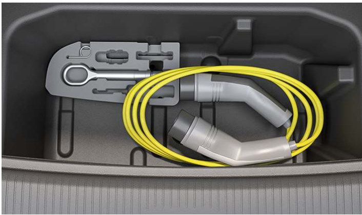
Fig. 2 Under the luggage compartment floor: stowage compartment with stowage space for the charging cable.
