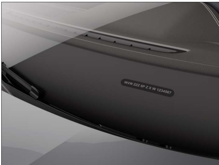
Fig. 1 In the windscreen: vehicle identification number.
