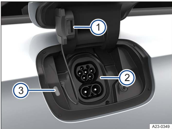
Fig. 2 Behind the charging socket flap at the rear right: charging socket.
