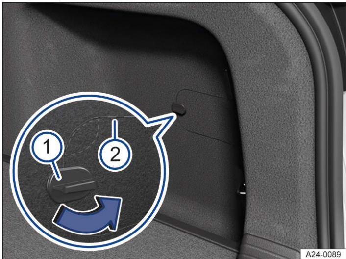
Fig. 1 In the lower right-hand side of the luggage compartment trim: flap with the coupling points.
