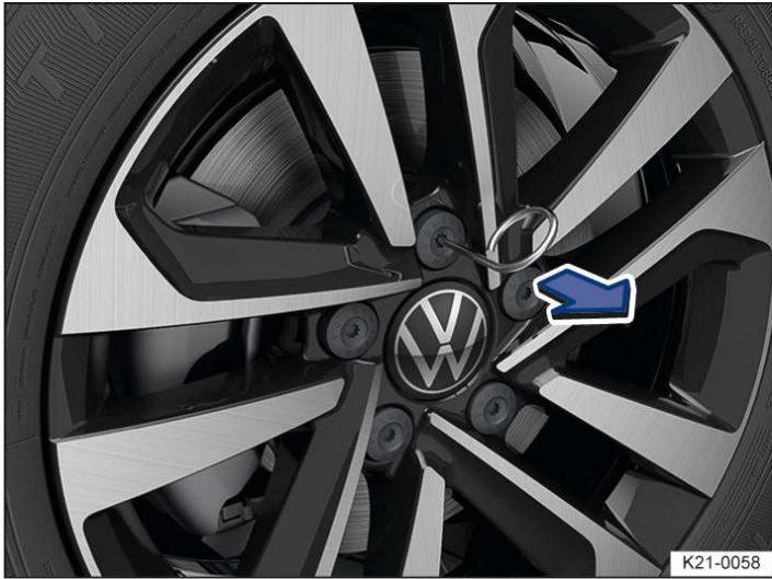
Fig. 1 Removing the wheel bolt caps.
