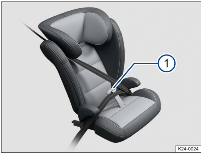
Fig. 2 Child seat with additional belt guide (illustration).
