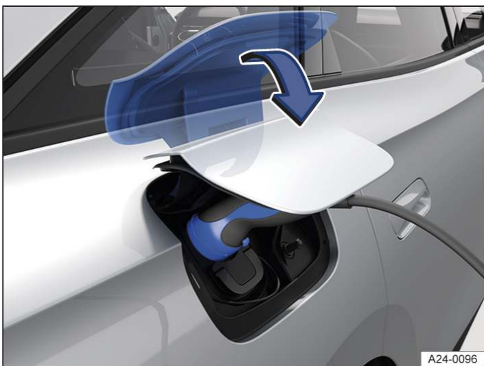
Fig. 4 On the rear right of the vehicle: charging socket flap in the weather protection position.
