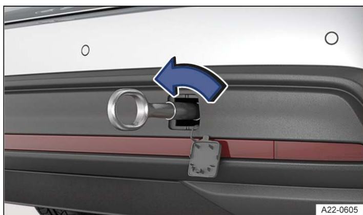
Fig. 3 In the rear bumper on the right: screwing in the towing eye, variant 1.
