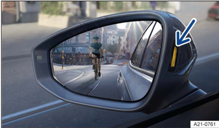
Fig. 1 In the exterior mirror housings: display of the exit warning system (illustration).
