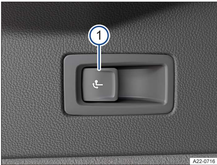
Fig. 1 On the left of the luggage compartment: button for releasing the ball coupling.
