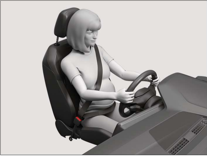
Fig. 2 Correct seat belt routing during pregnancy (illustration).
