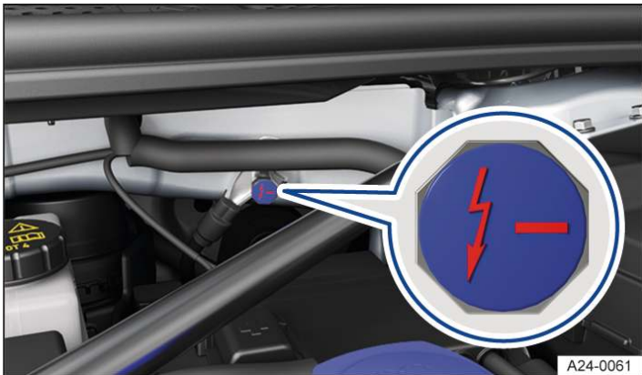
Fig. 2 In the bonnet space: jump-start connection point (earth).
