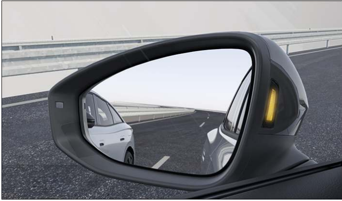
Fig. 1 In the housings of the exterior mirrors: Side Assist displays.
