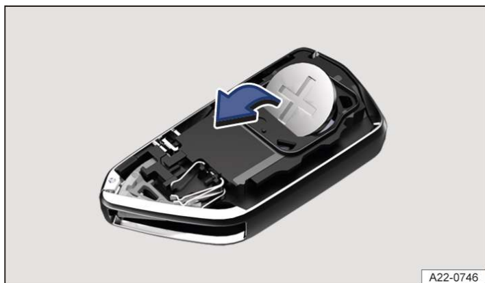
Fig. 2 Vehicle key: replacing the button cell.
