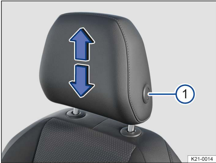
Fig. 1 Adjusting a front head restraint (illustration).
