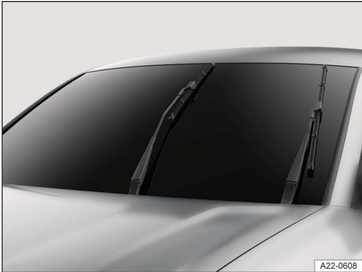
Fig. 1 Wipers in service position (illustration).
