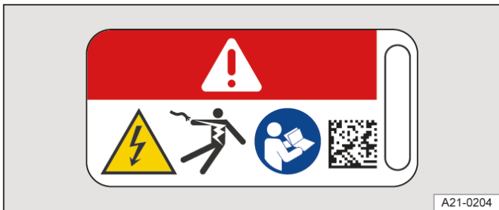
Fig. 2 Warning sign on high-voltage components.
