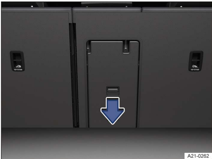
Fig. 2 In the luggage compartment: rear side of the load-through hatch (illustration).
