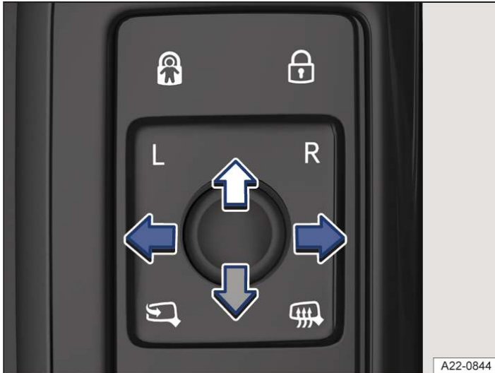
Fig. 1 In the driver door: rotary knob for the exterior mirrors.
