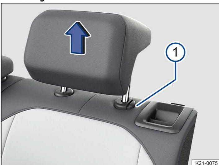
Fig. 2 Removing a rear head restraint (illustration).
