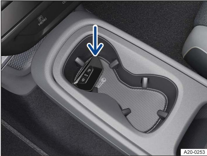
**Fig. 1** In the centre console: emergency start function.
