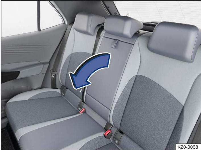
**Fig. 1** In the backrest of the middle seat: fold-out rear centre armrest.
