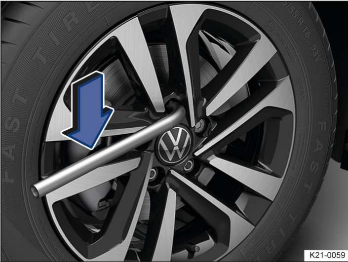
Fig. 1 Loosening wheel bolts.
