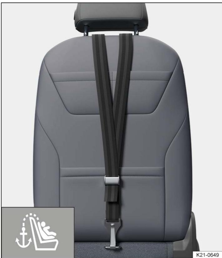
Fig. 2 On the rear of front passenger seat (country-dependent): attached top tether.
