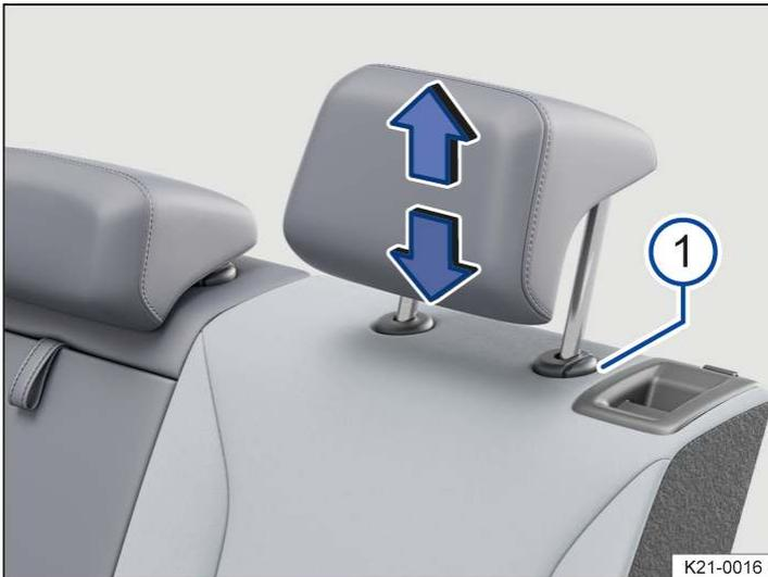
Fig. 2 Adjusting a rear head restraint (illustration).
