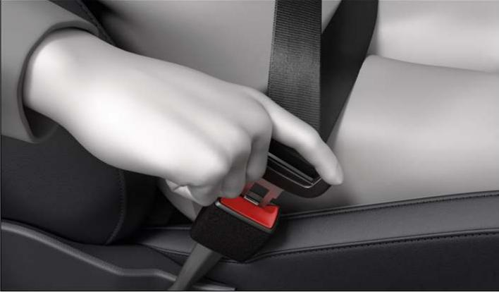
Fig. 1 Inserting the seat belt latch plate into the buckle (illustration).
