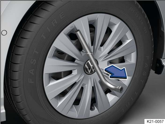
Fig. 1 Removing the wheel cover.
