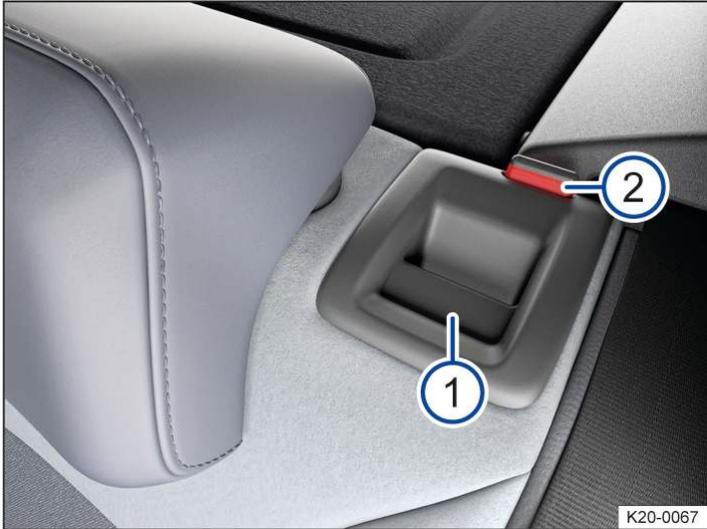
Fig. 1 In the rear seat backrest: release button.
