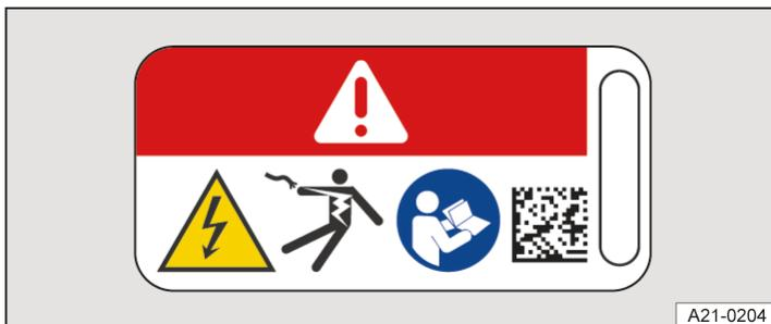
Fig. 2 Warning sign on high-voltage components.
