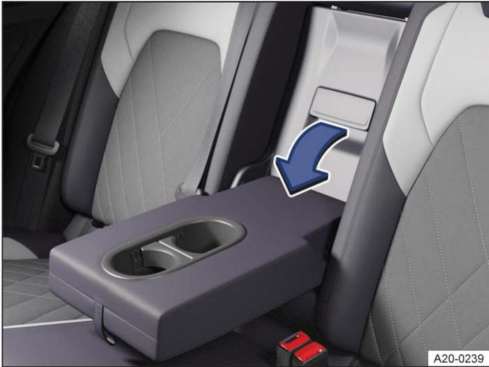
Fig. 1 In the rear seat backrest: load-through hatch (illustration)
