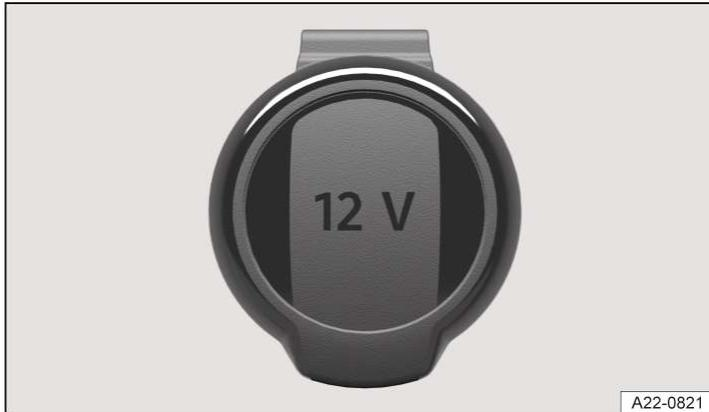
**Fig. 1** In the luggage compartment on the right-hand side: fold-open 12-volt socket (illustration).
