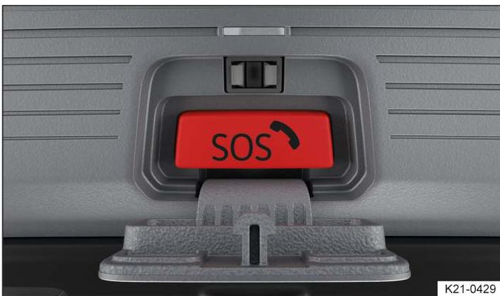
Fig. 2 In the roof console: button for Emergency Call Service.
