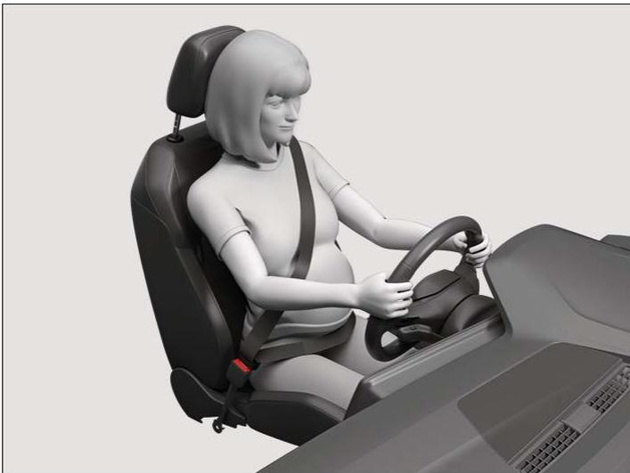
**Fig. 2** Correct seat belt routing during pregnancy (illustration).
