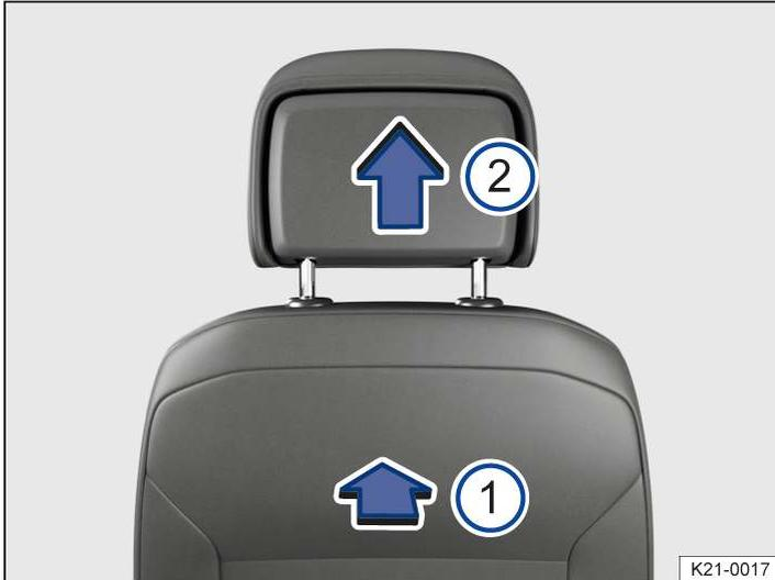
Fig. 1 Removing a front head restraint (illustration).
