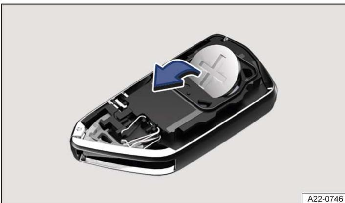
Fig. 2 Vehicle key: replacing the button cell.
