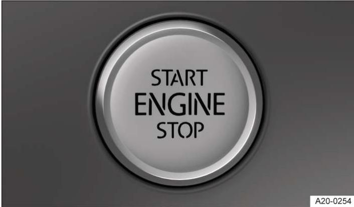
Fig. 1 On the right of the steering column: starter button.
