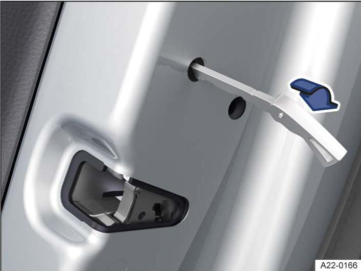
**Fig. 1** In the front edge of the rear door: locking the vehicle manually with the manual key (variant 1).
