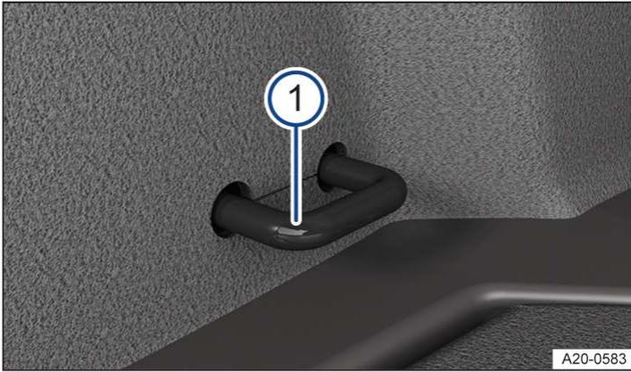
Fig. 1 In the luggage compartment: fastening ring (illustration).
