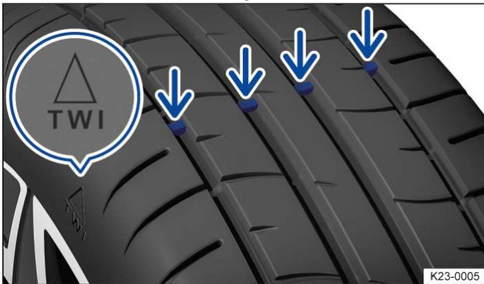
Fig. 1 In the tread grooves: tread wear indicator.
