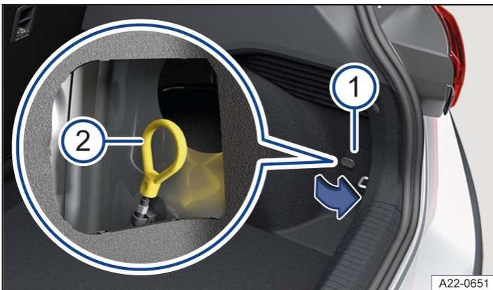
Fig. 2 In the lower right-hand side of the luggage compartment trim: manual release of the charging connector.
