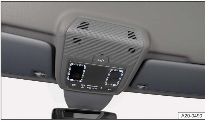
Fig. 1 In the roof console: touch-sensitive reading lights.
