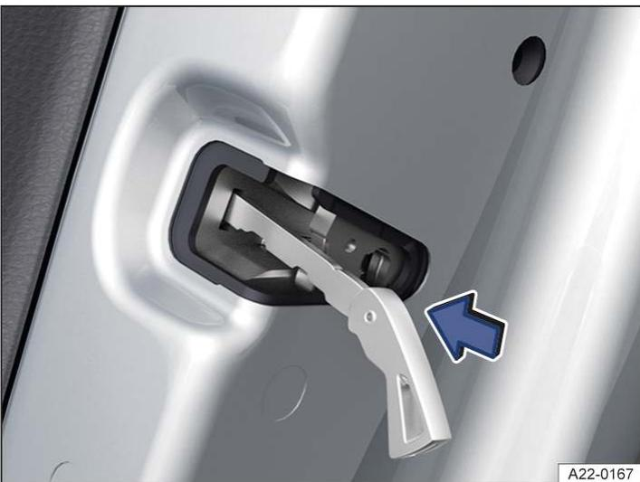
**Fig. 2** In the front edge of the rear door: locking the vehicle manually with the manual key (variant 2).
