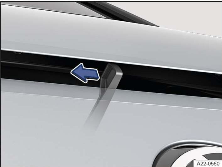
Fig. 2 On the bonnet: control lever. (illustration)
