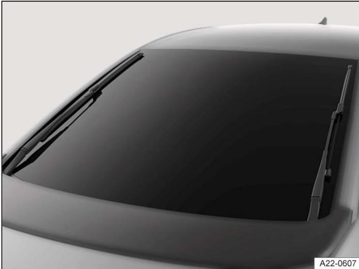
Fig. 1 Wipers in service position (illustration).
