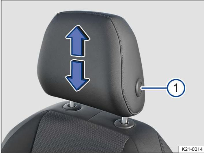
Fig. 1 Adjusting a front head restraint (illustration).
