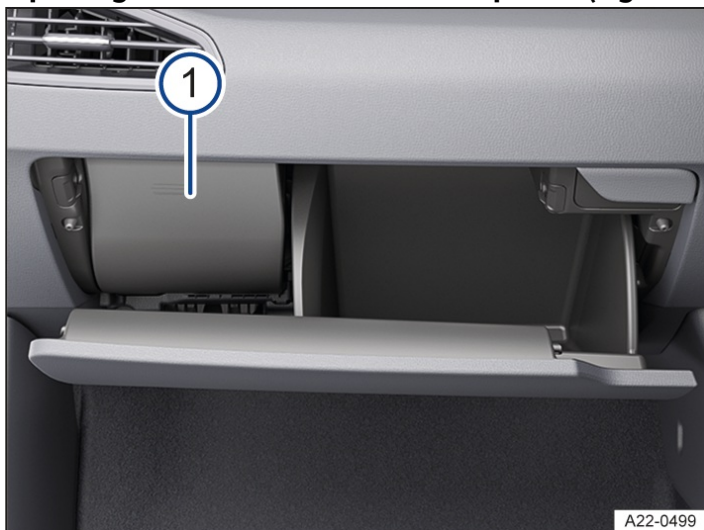
Fig. 2 In the dash panel on the front passenger side: fuse box (right-hand drive vehicle).
