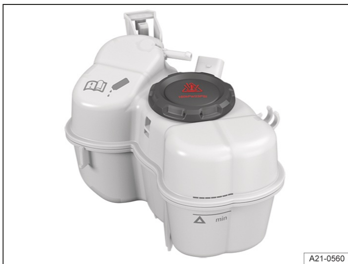
Fig. 2 In the bonnet space: markings on the coolant expansion tank (illustration).
