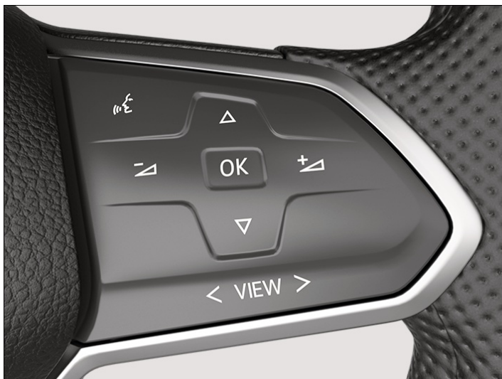
Fig. 1 Right-hand side of the multifunction steering wheel: controls for using the menus and information displays in the digital instrument cluster.
