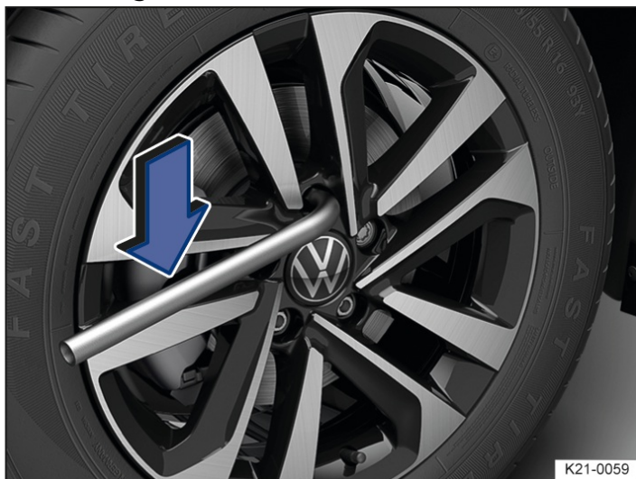
Fig. 1 Changing a wheel: loosening the wheel bolts.
