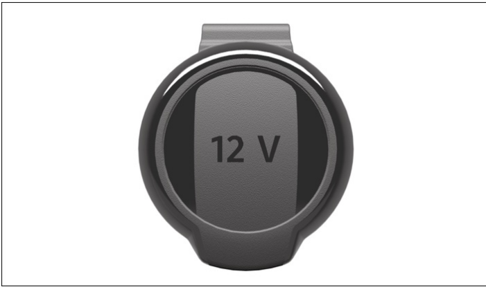
Fig. 1 In the luggage compartment on the right-hand side: fold-open 12-volt socket (illustration).
