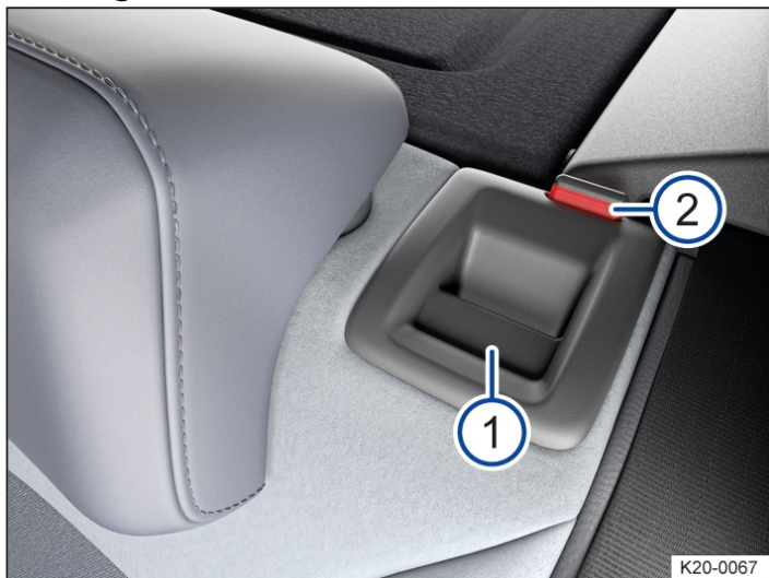
Fig. 1 In the rear seat backrest: release button.
