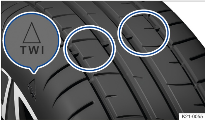
Fig. 1 Tyre tread: tread wear indicators.
