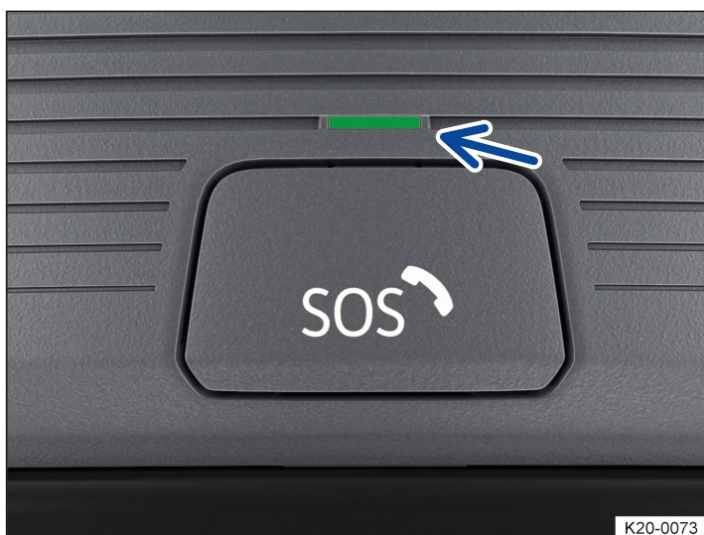
Fig. 1 In the roof console: control for legally required eCall Emergency System (behind button cover) and indicator lamp.
