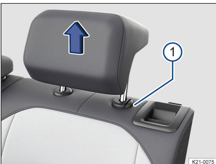
Fig. 2 Rear head restraint: removing(illustration).
