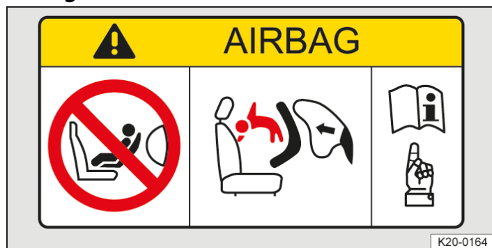
Fig. 1 Illustration: airbag label on the sun visor.
