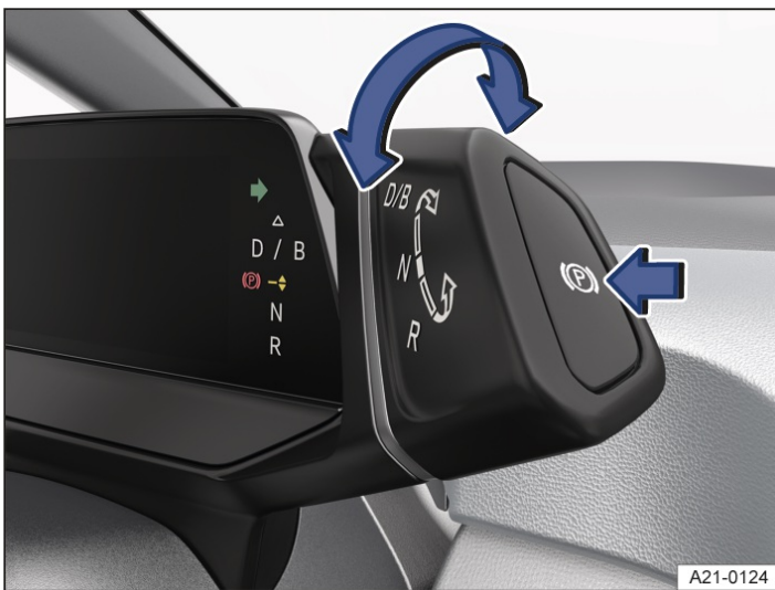
Fig. 1 Position switch with button for the electronic parking brake (arrow).
