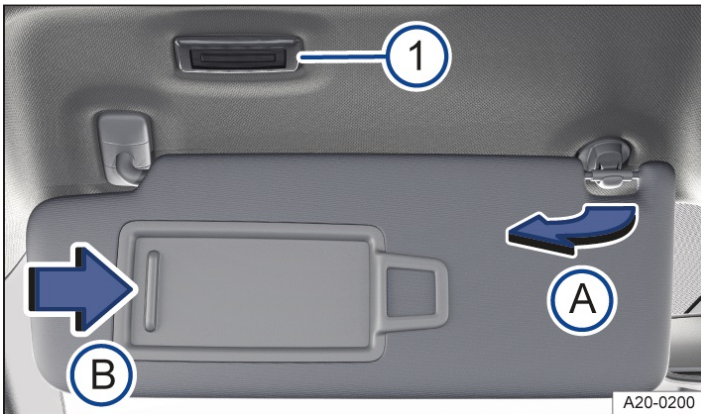
Fig. 1 In the front headliner: sun visor.
