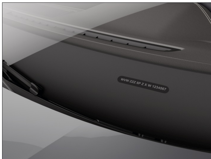
Fig. 1 In the windscreen: vehicle identification number.
