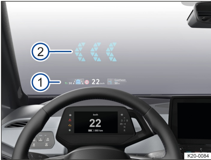
Fig. 1 In the driver's field of vision: head-up display close range (1) and AR head-up display (2).
