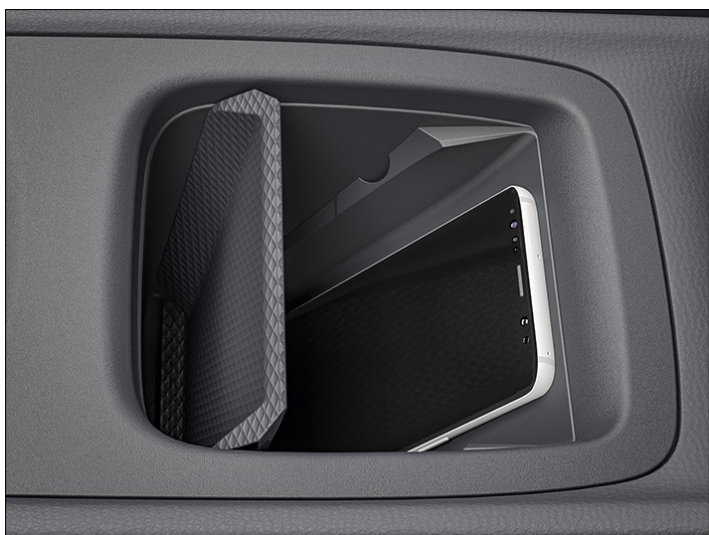
Fig. 2 Illustration: stowage compartment cover (open).
