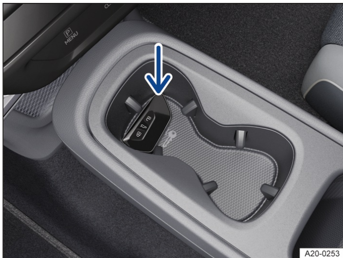
Fig. 1 In the centre console: emergency start function.
