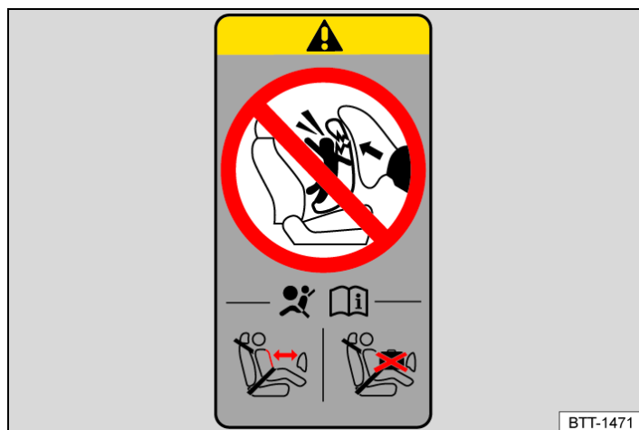
Fig. 2 Illustration: airbag label on the B-pillar.
