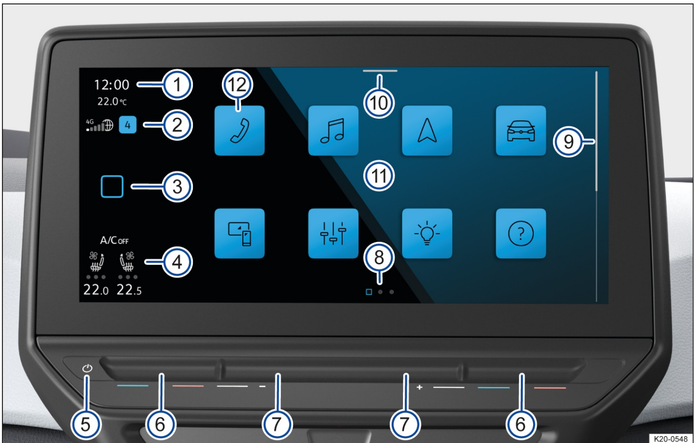
Fig. 1 Overview: display and operating unit of the 10-inch version(10").
