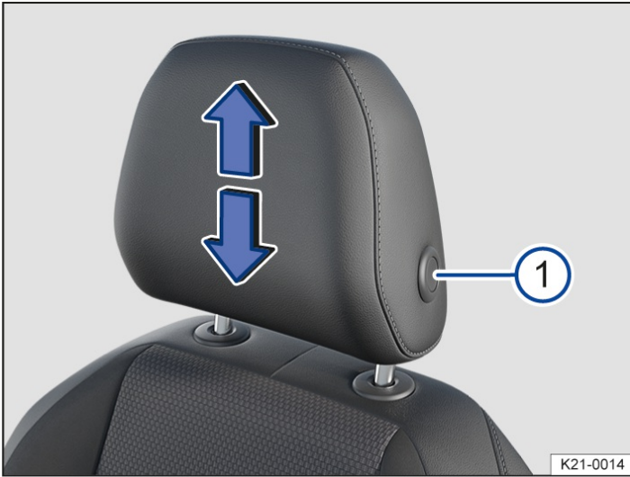
Fig. 1 Front head restraint: adjusting (illustration).
