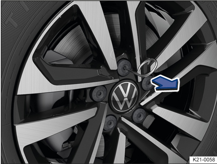
Fig. 1 Removing the wheel bolt caps.
