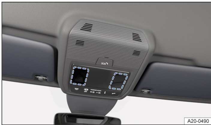
Fig. 1 In the roof console: touch-sensitive reading lights.
