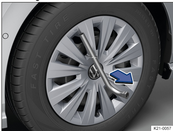
Fig. 1 Removing the wheel cover.
