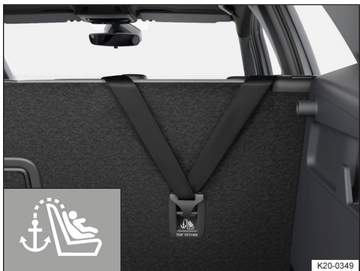
Fig. 1 In the luggage compartment: attached top tether.
