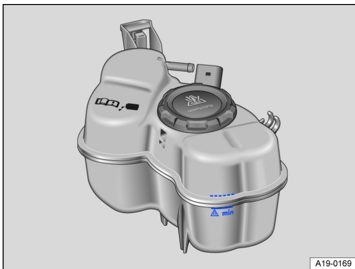
Fig. 2 In the bonnet space: markings on the coolant expansion tank.
