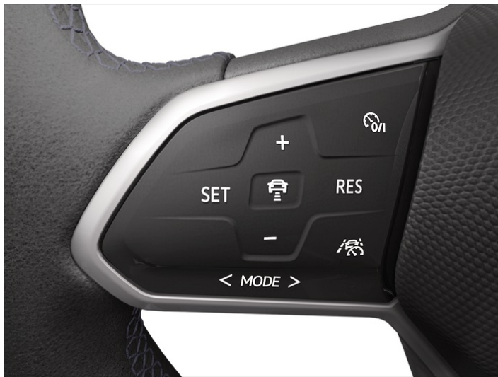
Fig. 1 Lefthand side of the multifunction steering wheel.
