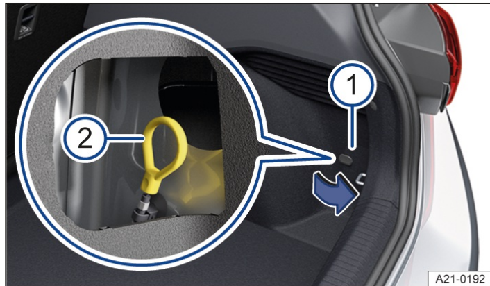
Fig. 1 Behind the flap in the right-hand luggage compartment trim: manual release mechanism for the charging connector.
