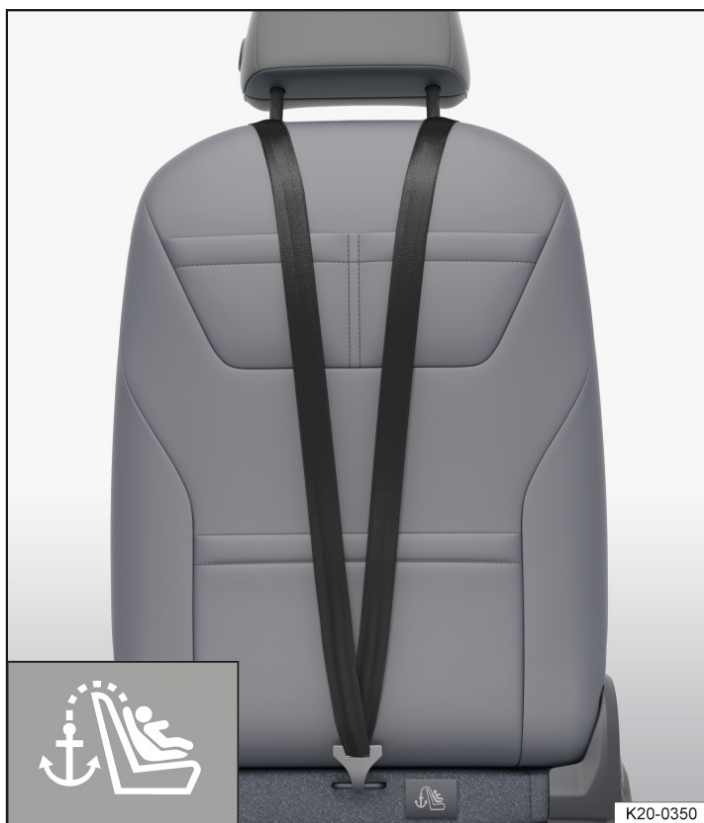
Fig. 2 On the rear of the front passenger seat(country-dependent): attached top tether.
