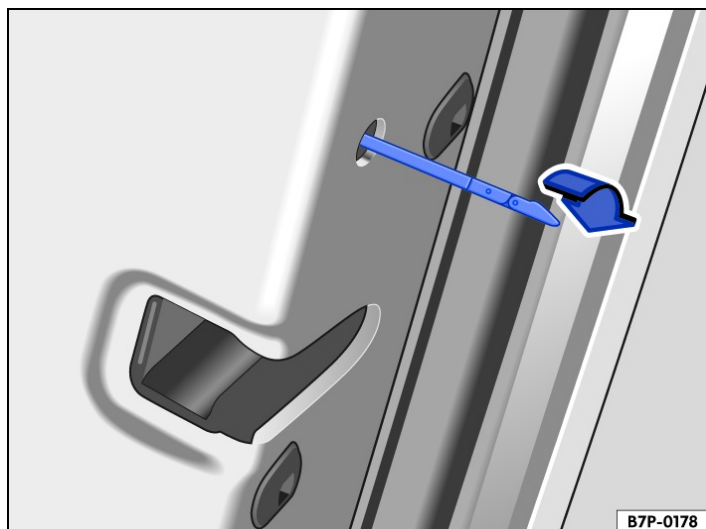
Fig. 1 In the front edge of the rear right-hand door: locking the vehicle manually with the spare key (variant 1).
