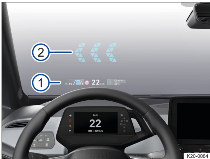
Fig. 1 In the driver's field of vision: head-up display close range
