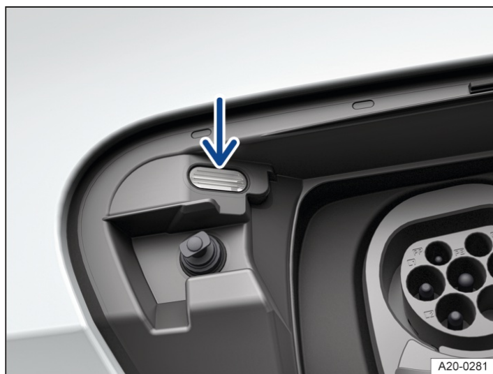
Fig. 1 Behind the charging socket flap: charging process indicator.
