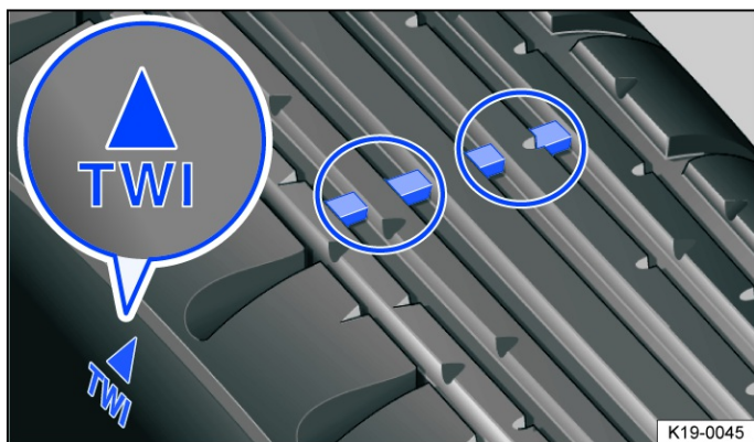
Fig. 1 Tyre tread: tread wear indicators.
