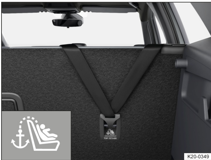
Fig. 1 In the luggage compartment: attached top tether.
