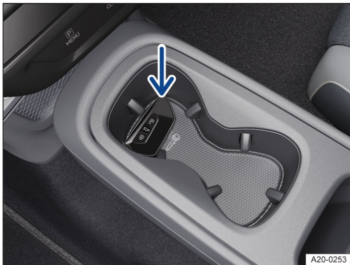
Fig. 1 In the centre console: emergency start function.
