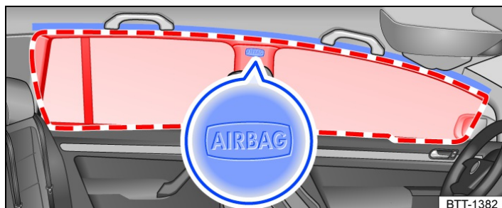
Fig. 1 On the left-hand side of the vehicle: location and deployment zone of the curtain airbag.
