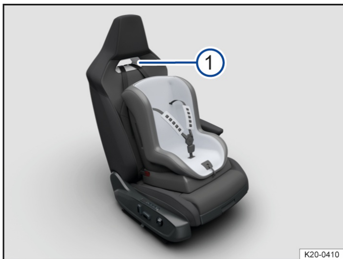
Fig. 3 In the backrest of the Top sports seat on the passenger side: opening for the top tether (schematic diagram).
