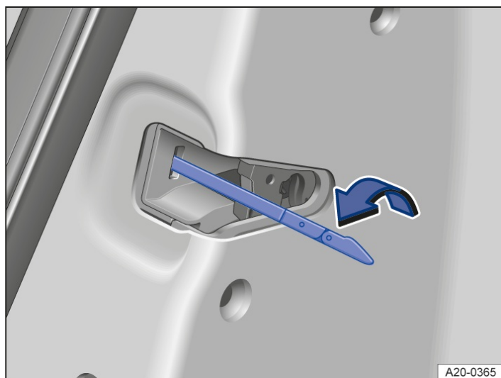
Fig. 2 In the front edge of the rear right-hand door: locking the vehicle manually with the spare key (variant 2).
