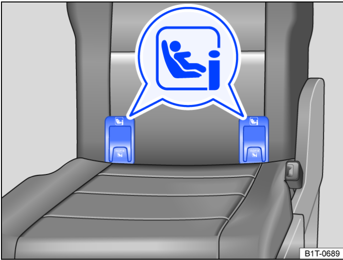
Fig. 2 Markings identifying the i-size anchorage points for child seats.
