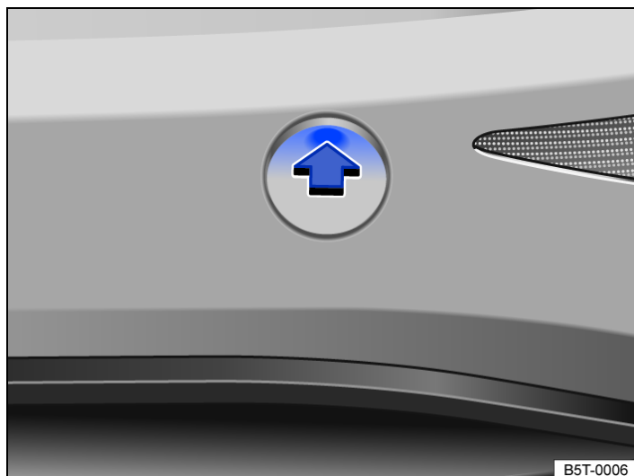
Fig. 1 In the rear bumper on the right: removing the cover.
