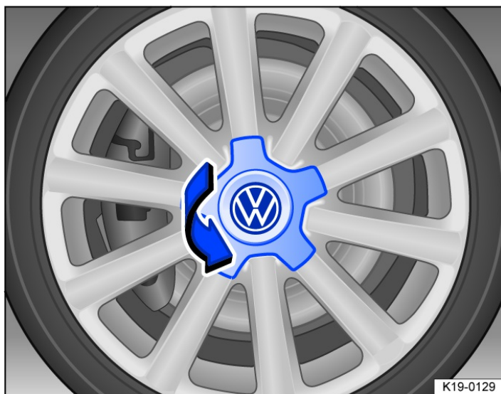
Fig. 2 Removing the centre wheel trim by turning.
