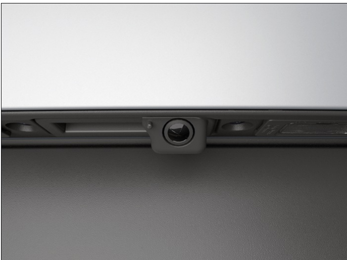
Fig. 3 At the rear of the vehicle: rear view camera system on the handle button (illustration).
