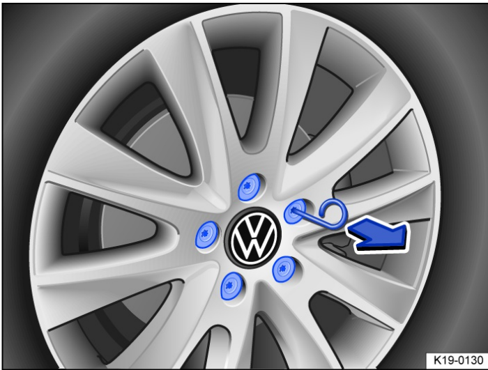
Fig. 1 Removing the wheel bolt caps.
