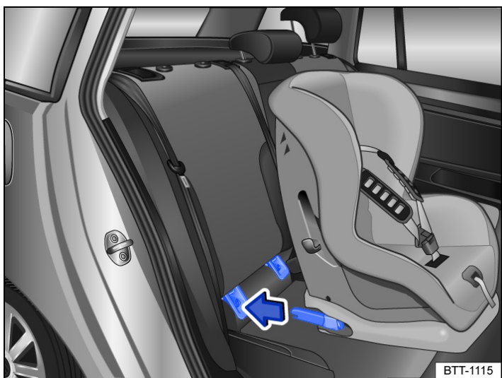
Fig. 3 Illustration: fitting a child seat with the attachment arms.
