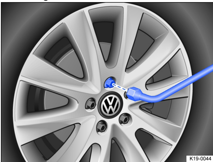
Fig. 1 Wheel change: Unscrew the wheel bolts with the wheel wrench.
