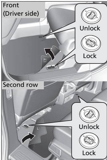
The front and second row floor mats hook over floor anchors, which keep them from sliding forward. To remove a mat for cleaning, turn the anchor knobs to the unlock position. When reinstalling the mat after cleaning, turn the knobs to the lock position.
