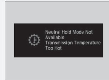
The transmission may not stay in **N** position while the following indicator is on:
