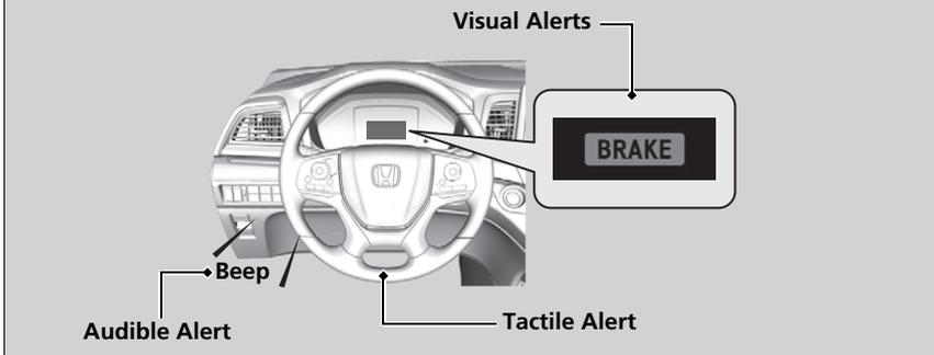
At system's earliest collision alert stage, you can change the distance (**Long/Normal/Short**) between vehicles at which alerts will come on through audio/information screen setting options.
