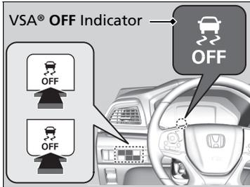
This button is on the driver side control panel. To partially disable VSA® functionality/features, press and hold it until you hear a beep.
