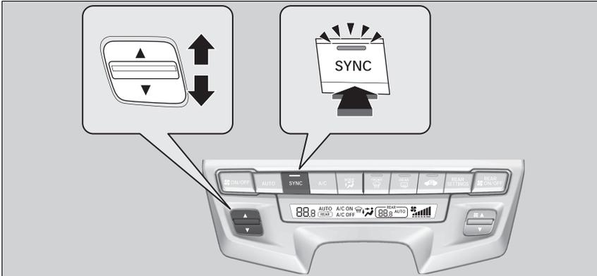
You can set the temperature synchronously for the front compartment and the rear passenger compartment in synchronization mode.
