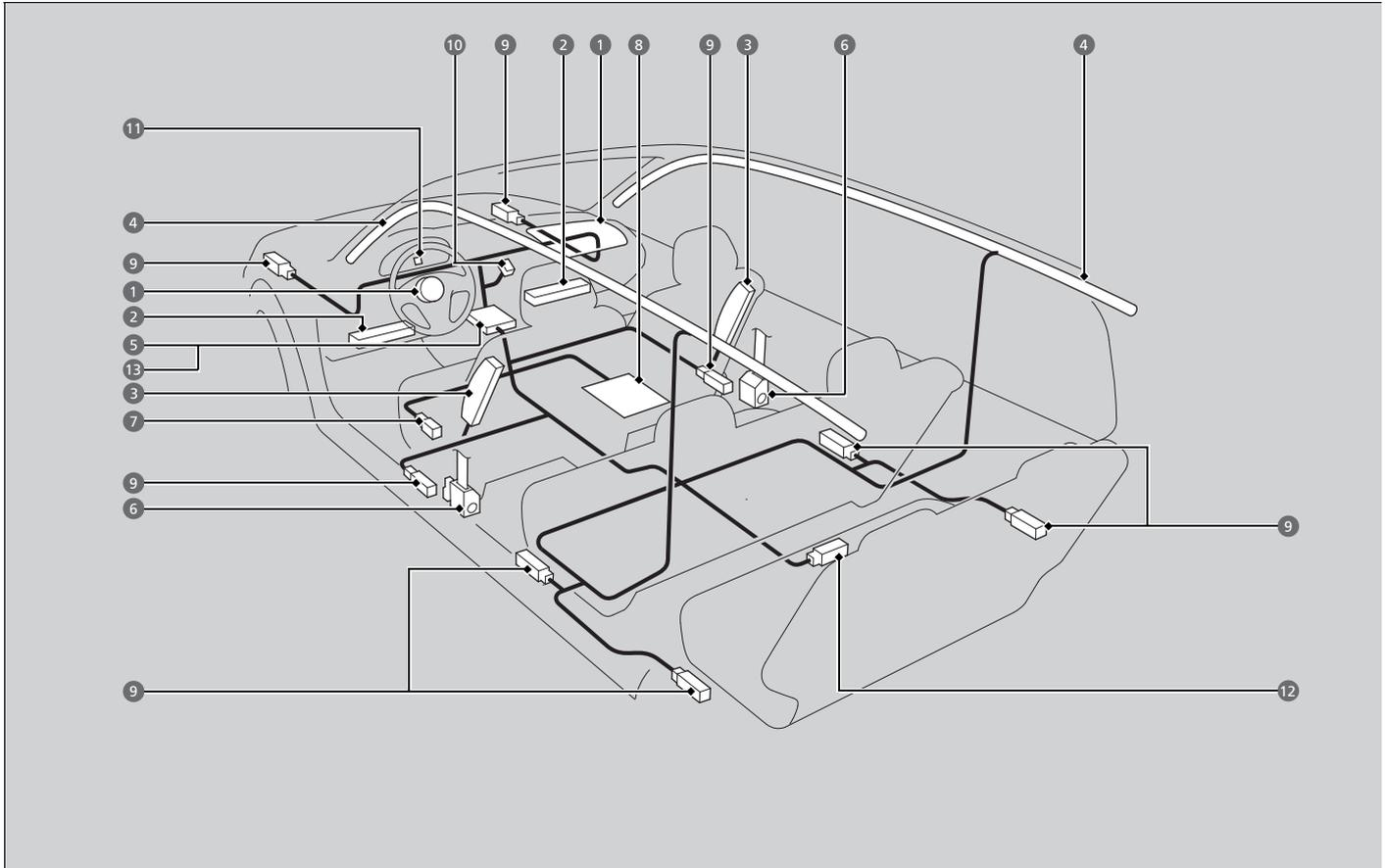
The front, driver's and passenger's knee, front side, and side curtain airbags are deployed according to the direction and severity of impact. Both side curtain airbags are deployed in a rollover. The airbag system includes:
