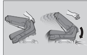
Install the head restraints, then raise the seat-back to an upright position, then rock the seat-back and forth to confirm both the inner and outer latches are securely locked into position.
