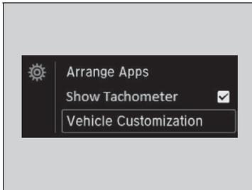
2. Press the
