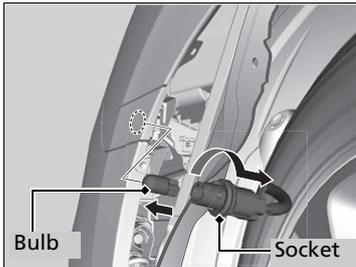
3. Rotate the socket counter-clockwise and remove it.
