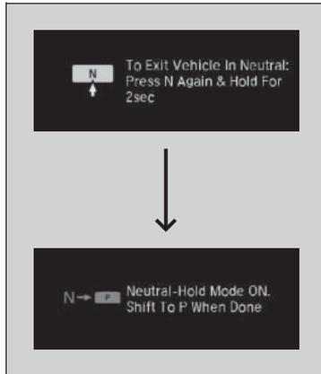
If the **ENGINE STOP/START** button is pressed after car wash mode has been activated, the power mode will change to ACCESSORY and a message will be displayed on the driver information interface.
