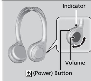
**To turn on the switch:** Press the
