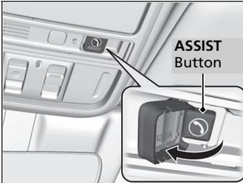
If you need to talk to the HondaLink® operator in a situation where no airbag has deployed, you can manually connect to them by pressing the **ASSIST** button with the power mode in ACCESSORY or ON.
