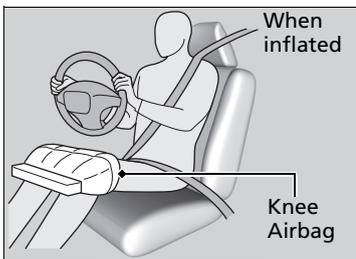
When the driver's front airbag inflates, the driver's knee airbag also inflates. When front passenger's airbag inflates, the front passenger's knee airbag also inflates.
