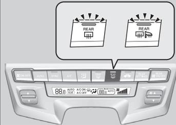
Press the rear defogger and heated door mirror\* button to defog the rear window and mirrors\* when the power mode is in ON.
