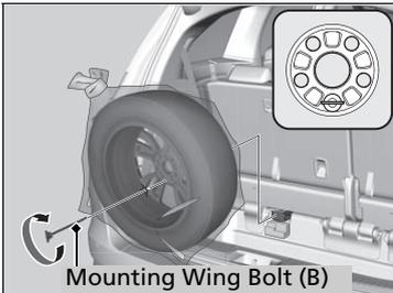
5. Install the flat tire on the bracket with the inside of the wheel facing toward you.
