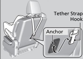
2. Put the head restraint to its upper-most position, then route the tether strap outside/through the head restraint legs. Make sure the strap is not twisted.
