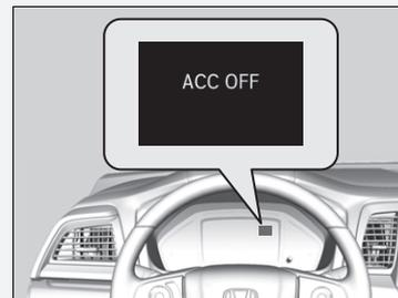
Even though ACC has been automatically canceled, you can still resume the prior set speed. Wait until the condition that caused ACC to cancel improves, then press the **RES/+** button.
