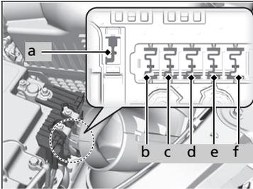
1. Remove the engine compartment cover and the air intake duct.
