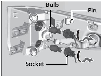
5. Turn the socket counter-clockwise and remove it. Remove the old bulb.
