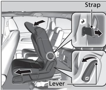
1. Pulling forward on the walk-in lever or pulling the release strap tilts the second row outer seat's seat-back forward.
