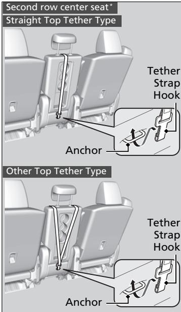
3. Secure the tether strap hook to the anchor.
