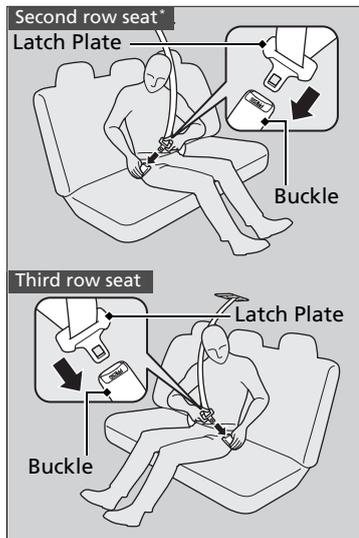
3. Insert the latch plate into the buckle. Properly fasten the seat belt the same way you fasten the lap/shoulder seat belt.
