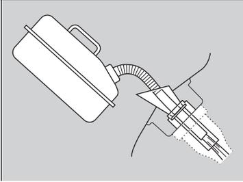
6. Fill the tank with fuel from the portable fuel container.
