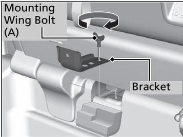
4. Install the bracket and the mounting wing bolt (A) on the attachment point, and tighten the bolt.
