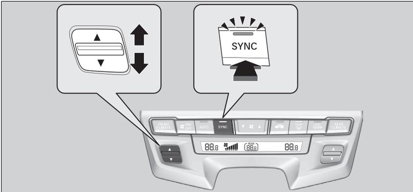
You can set the temperature synchronously for the driver side, the passenger side and the rear passenger compartment in synchronization mode.
