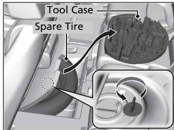
4. Take the tool case out of the spare tire well. Take the jack and wheel nut wrench out of the tool case.
