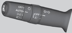
Automatic lighting control can be used when the power mode is in ON.
