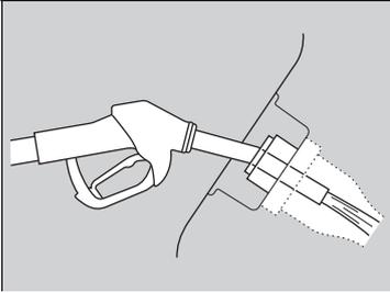
5. Place the end of the filler nozzle on the lower part of filler opening, then insert it slowly and fully.
