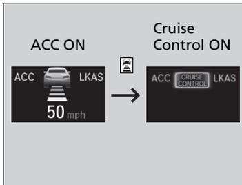
Press and hold the
