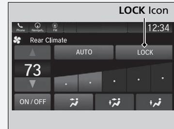
Select the **LOCK** icon to turn the rear lock mode on and off.
