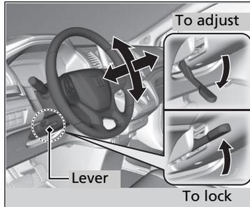
1. Push the steering wheel adjustment lever down.
