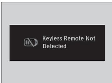
Warning buzzers may sound from inside and/or outside the vehicle to remind you that the remote is out of the vehicle. If the buzzer continues even after the remote is put back inside, place it to be within its operational range.
