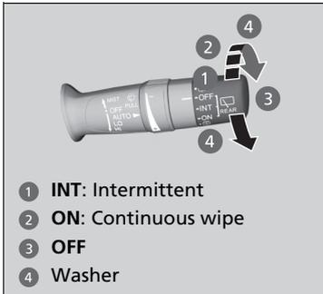
The rear wiper and washer can be used when the power mode is in ON.
