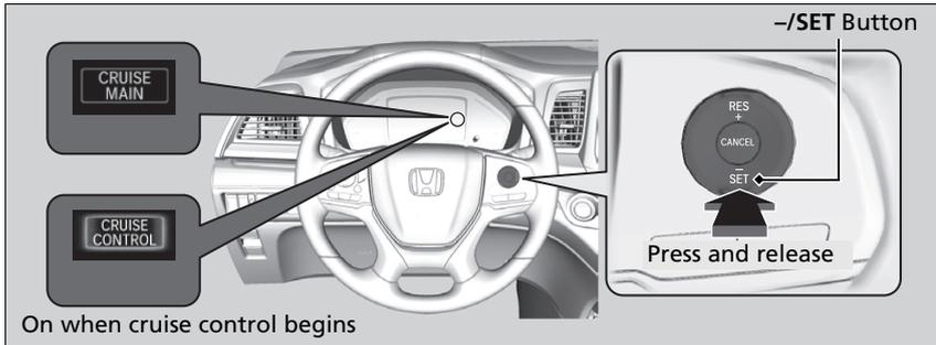
Take your foot off the pedal and press the **-/SET** button when you reach the desired speed. The moment you release the **-/SET** button, the set speed is fixed, and cruise control begins. The **CRUISE CONTROL** appears on the driver information interface.
