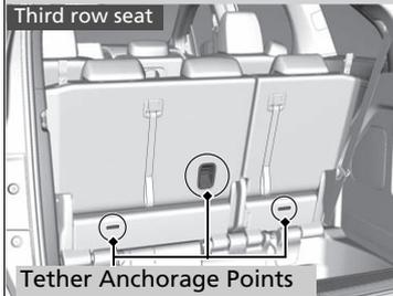
A tether anchorage point is provided behind each second and third row seating position. If you have a child restraint system that comes with a tether but can be installed with a seat belt, the tether may be used for additional security.
