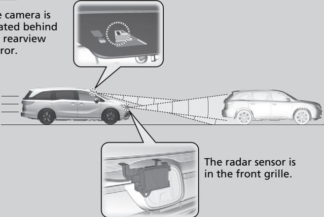
The radar sensor is in the front grille.
