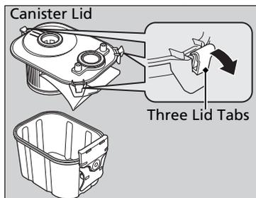
4. Push the three lid tabs outward and remove the canister lid.
