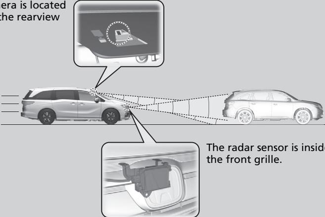
The radar sensor is inside the front grille.
