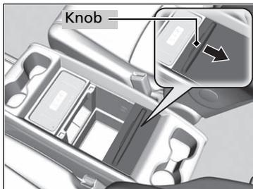
To open the console compartment, press the knob to unlock the lid, and then slide it rearward.
