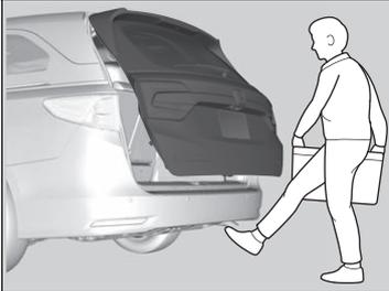
Use a forward and back kicking motion under the center of the rear bumper to open or close the power tailgate while carrying the smart entry remote.
