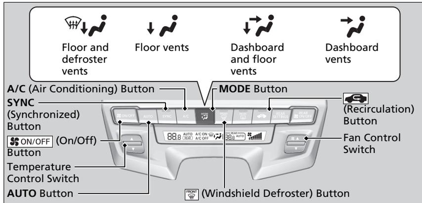
Use the system when the engine is running.
