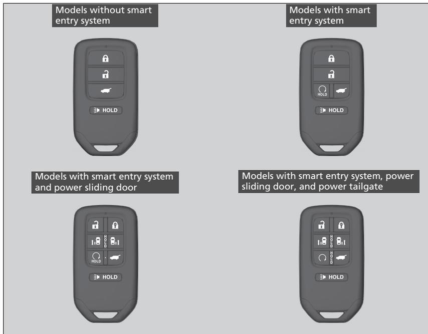
Use the keys to start and stop the engine, and to lock and unlock all the doors, tailgate, and fuel fill door. You can also use the remote transmitter or smart entry system\* to lock and unlock all the doors, tailgate, and fuel fill door.
