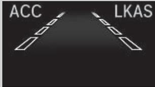
When the LKAS is suspended, the lane lines on the driver information interface change to contour lines, and the beeper sounds (if activated).
