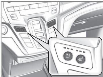
Press the seat heater or the seat ventilation button:
