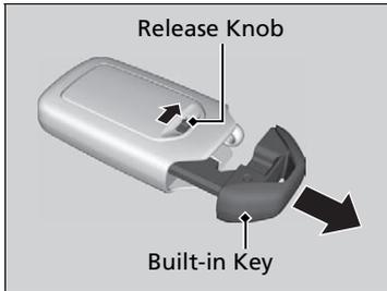
The built-in key can be used to lock/unlock the doors and tailgate when the remote battery becomes weak and the power door lock/unlock operation is disabled.
