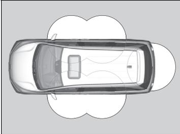
When you carry the remote, you can lock/unlock the doors, fuel fill door, and open the tailgate.
