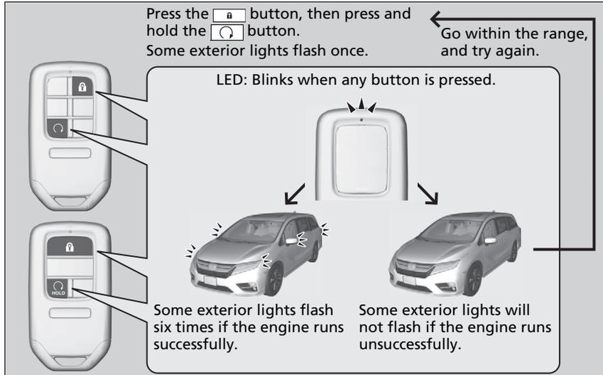
When started remotely, the engine automatically shuts off after 10 minutes of idling and/or the brake pedal and **ENGINE START/STOP** button have not been pressed simultaneously.
