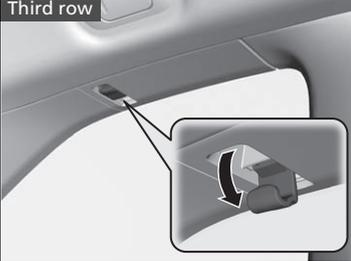
There are coat hooks under the grab handles in the second row, and under the window frames in the third row. Pull it down to use it.
