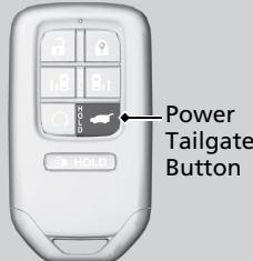
Press the power tailgate button for more than one second to operate the power tailgate when the power mode is in VEHICLE OFF.
