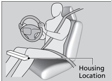
The driver's knee airbag is housed under the steering column. The front passenger's knee airbag is stored under the glove box.
