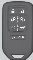
Use the keys to start and stop the engine, and to lock and unlock all the doors, tailgate, and fuel fill door. You can also use the remote transmitter or smart entry system\* to lock and unlock all the doors, tailgate, and fuel fill door.
