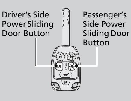
Press the power sliding door button for more than one second to operate.
