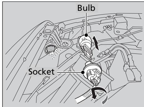
1. Turn the socket to the left and remove it.
