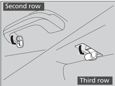
There are coat hooks on the both side of the grab handle and the window frame. Pull it down to use it.
