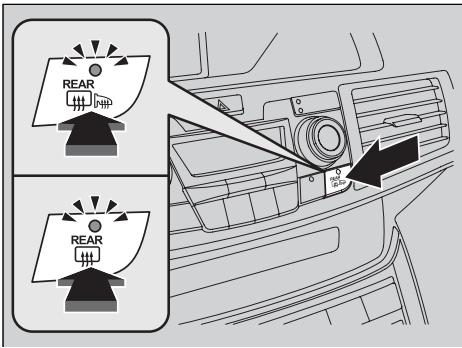
Press the rear defogger and heated door mirror button to defog the rear window and mirrors when the ignition switch is in ON **II**.
