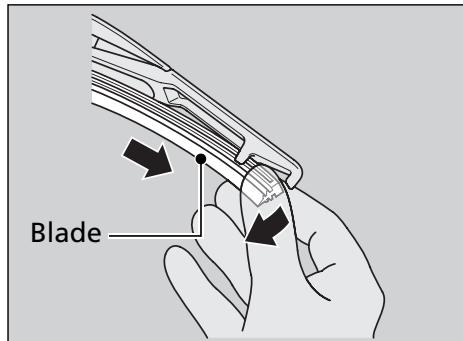
3. Slide the blade out of the wiper.
