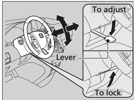
1. Push the steering wheel adjustment lever down.
