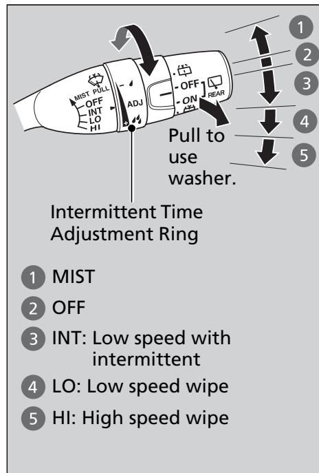
The windshield wipers and washers can be used when the ignition switch is in ON **II**.
