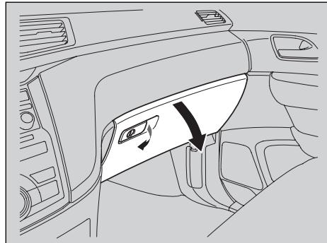
Pull the handle to open the glove box. You can lock the glove box with the master key.
