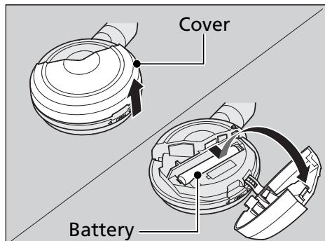
2. Make sure to replace the battery with the correct polarity.
