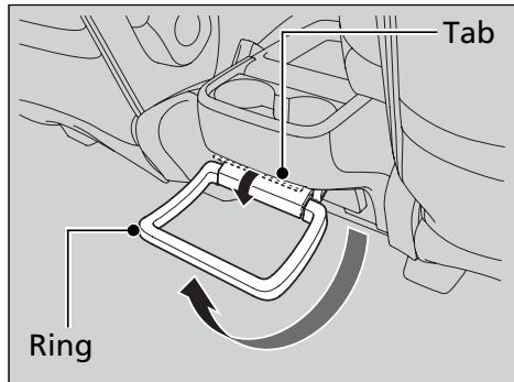
Pull up the ring until it clicks, and lift the tab. Put a plastic bag in the ring. Push the tab down to hold the bag.
