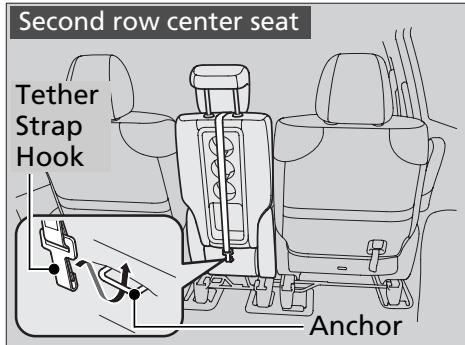
3. Raise the head restraint to its highest position, then route the tether strap between the head restraint legs, and secure the tether strap hook onto the anchor.
