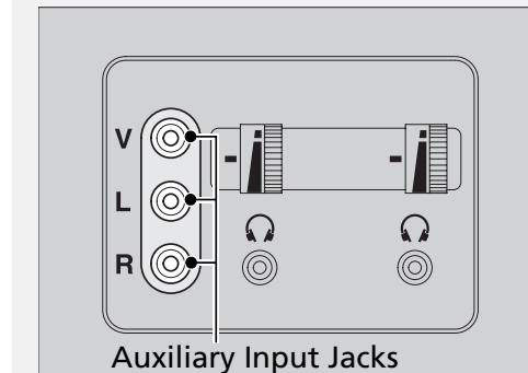
The system also allows for auxiliary inputs from standard video games. The jacks are above the third row seat armrest on the driver's side.
