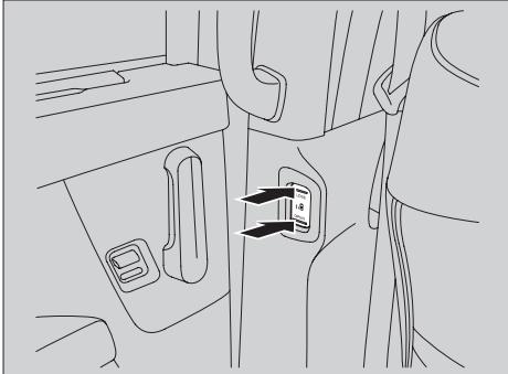
The power sliding door opens when you press the OPEN side of the / switch, and closes when you press the CLOSE side of the / switch.
