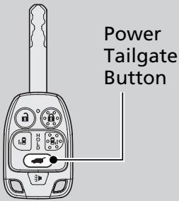
Press the power tailgate button for more than one second to operate.
