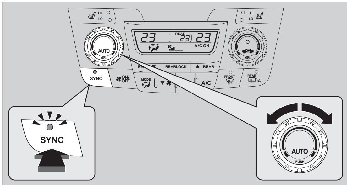
You can set the temperature synchronously for the driver side, the passenger side and the rear passenger compartment in synchronized mode.
