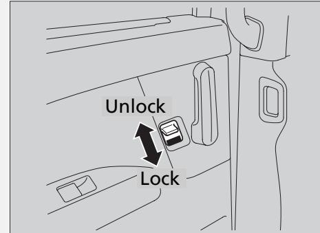
To open the door from the inside when the childproof door lock is on, put the lock tab in the unlock position, lower the rear window, put your hand out of the window, and pull the outside door handle.
