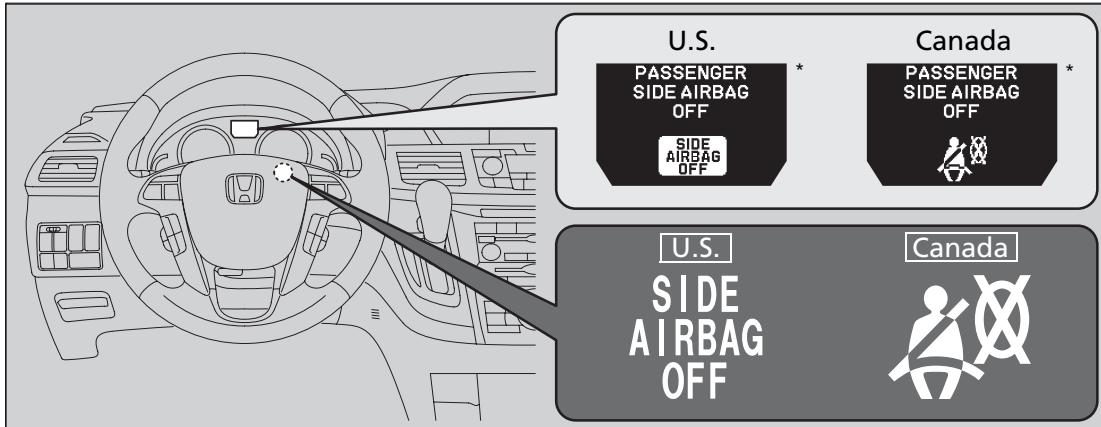
This indicator comes on if the passenger's side airbag has been turned off because the passenger is too small to be sitting in the front seat, is slouching or not sitting upright, or has leaned into the airbag's deployment path.
