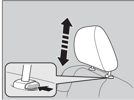
**To raise the head restraint:** Pull it upward.
