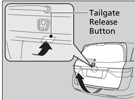
When all the doors are unlocked, the tailgate is unlocked. Push the tailgate release button and lift open the tailgate.
