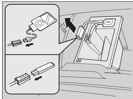
1. Unclip the USB connector and loosen the adapter cable.
