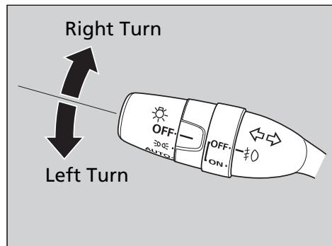
The turn signals can be used when the ignition switch is in ON **II**.
