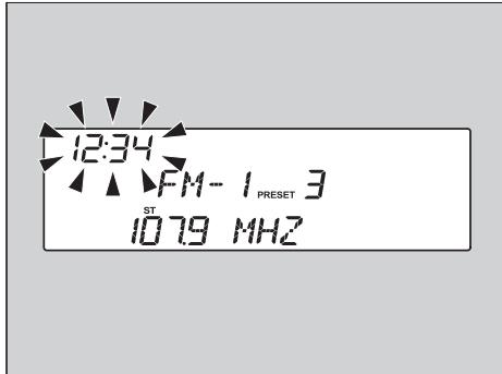
1. Press the CLOCK button until the displayed time begins flashing.
