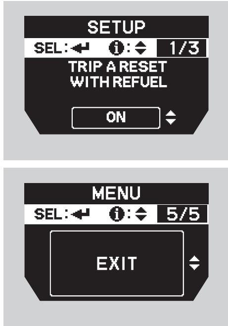
6. Press the  $\blacktriangle$  /  $\blacktriangledown$  button and select **ON**, then press the SEL/RESET button.
