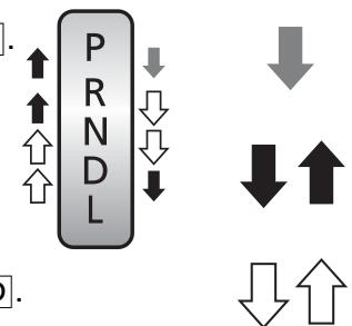
Depress the brake pedal and press the release button to move out of **P**.
