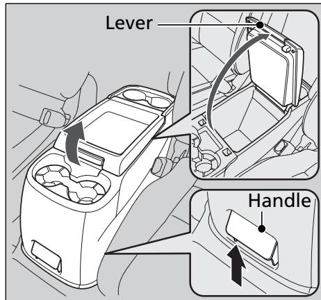
Pull up on the lever to open the console compartment.
