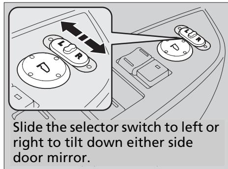
If activated, either side door mirror automatically tilts downward when you put the shift lever in **[R]**; this improves close-in visibility on the selected side of the vehicle when backing up. The mirror automatically returns to its original position when you shift out of **[R]**.
