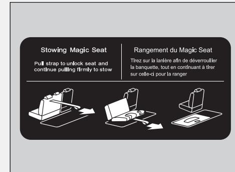
When you tuck away one side of the third row seats and use the non-recessed part of the cargo area, make sure to secure the cargo. Loose items can fly forward and cause injury if you have to brake hard.
