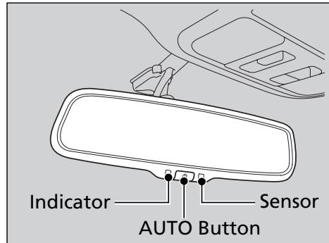
When driving after dark, the automatic dimming rearview mirror reduces the glare from headlights behind you. Press the AUTO button to turn this function on and off. When activated, the AUTO indicator comes on.
