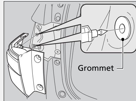
To reinstall, insert the fasteners into the grommets and push the assembly back into place.
