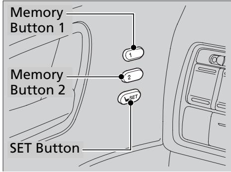
1. Adjust the driver's seat and the outside mirrors to the desired position, and turn the ignition switch to ON **II**.
