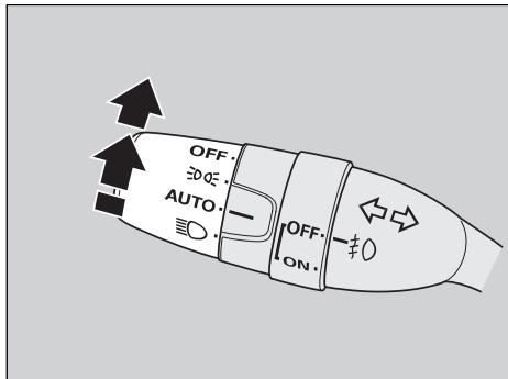
Automatic lighting control can be used when the ignition switch is in ON **[II]**.
