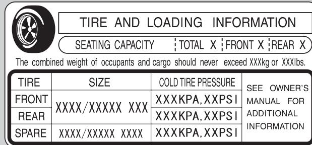
This figure includes the total weight of all occupants, cargo, and accessories, and the tongue load if you are towing a trailer.
