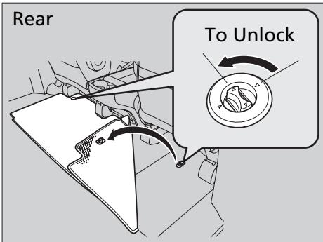
The front and second row passenger's floor mats hook over the floor anchors, which keep the mats from sliding forward. To remove a mat for cleaning, turn the anchor knobs to the unlock position. When reinstalling the mat after cleaning, turn the knobs to the lock position.
