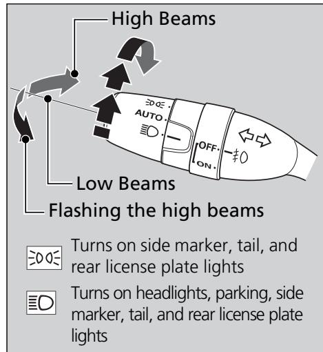
Rotating the light switch turns the lights on and off, regardless of the position of the ignition switch.
