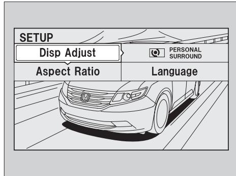
Press the SETUP button while the DVD is playing to see the available options. Use the  $\blacktriangle$ ,  $\blacktriangledown$ ,  $\blacktriangleright$ , and  $\blacktriangleleft$  buttons to highlight the option and then press the ENTER button.
