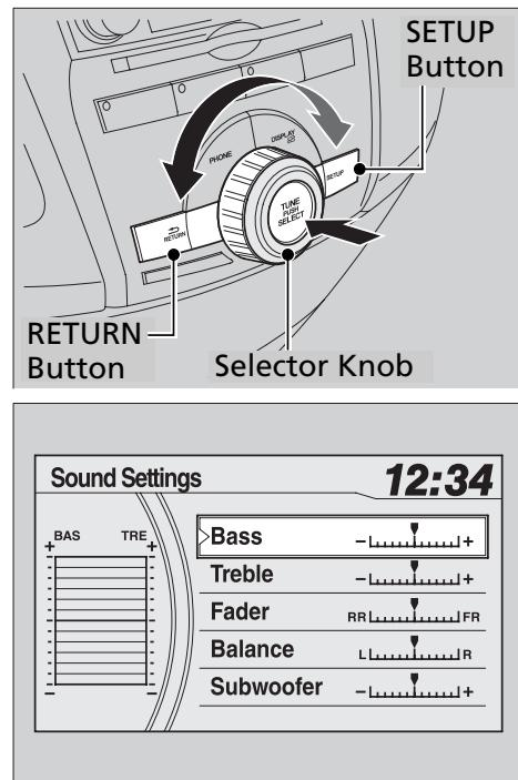
Press the SETUP button, and rotate to adjust the setting. Rotate to scroll through the following choices:
