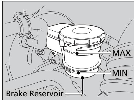
The fluid level should be between the MIN and MAX marks on the side of the reservoir.
