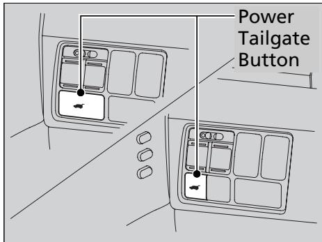
To open or close the power tailgate, press the tailgate button on the dashboard for about one second. The beeper sounds and some exterior lights flash.
