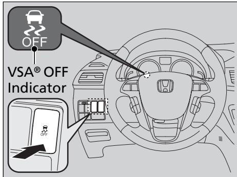
This button is on the driver side control panel. To turn the VSA® system on and off, press and hold it until you hear a beep.
