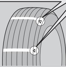
The groove where the wear indicator is located is 1/16 inch (1.6 mm) shallower than elsewhere on the tire. If the tread has worn so that the indicator is exposed, replace the tire. **Worn out tires have poor traction on wet roads.**
