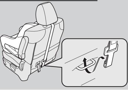
A tether anchorage point is provided behind each second and third row seating position. A child seat that is installed with a seat belt and comes with a tether can use the tether for additional security.
