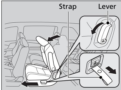
Pulling up on the seat-back angle adjustment lever, or pulling the release strap tilts the second row outer seat's seat-back forward.
