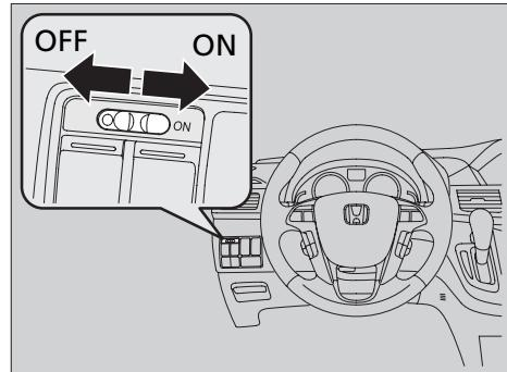
**Automatic operation:** Select the ON position of the sliding door main switch.
