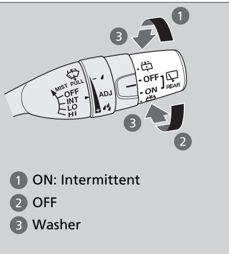
The rear wiper and washer can be used when the ignition switch is in ON **II**.
