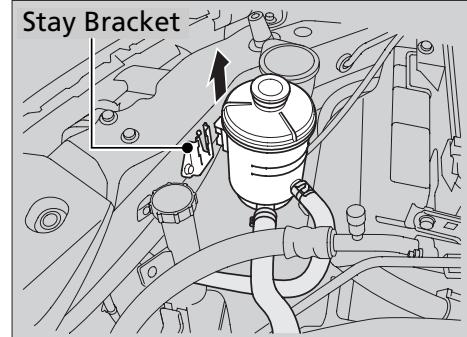
Remove the power steering reservoir from the stay bracket.
