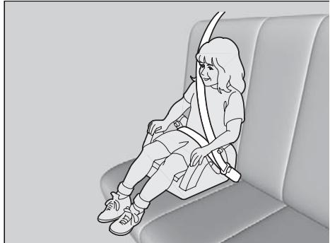
If a lap/shoulder seat belt cannot be used properly, position the child in a booster seat in a rear seating position. For the child's safety, check that the child meets the booster seat manufacturer's recommendations.
