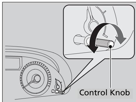
When the ignition switch is in ON **II**, you can use the brightness control knob to adjust instrument panel brightness.
