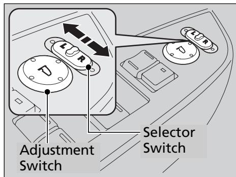
You can adjust the door mirrors when the ignition switch is in ON **[II]**.
