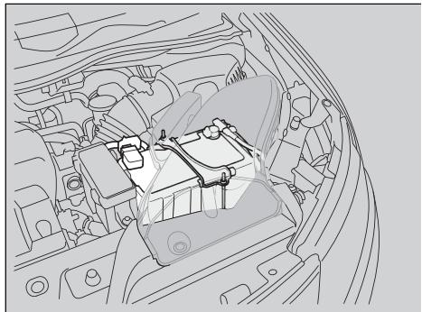
The battery condition is being monitored by the sensor on the negative terminal. If there is a problem with the sensor, the warning message on information display\*/multi-information display\* will let you know. Have your vehicle checked by a dealer.
