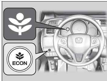
The **ECON** button turns the ECON mode on and off. The ECON mode helps you improve your fuel economy by adjusting the performance of the engine, transmission, climate control system\*, and cruise control\*.
