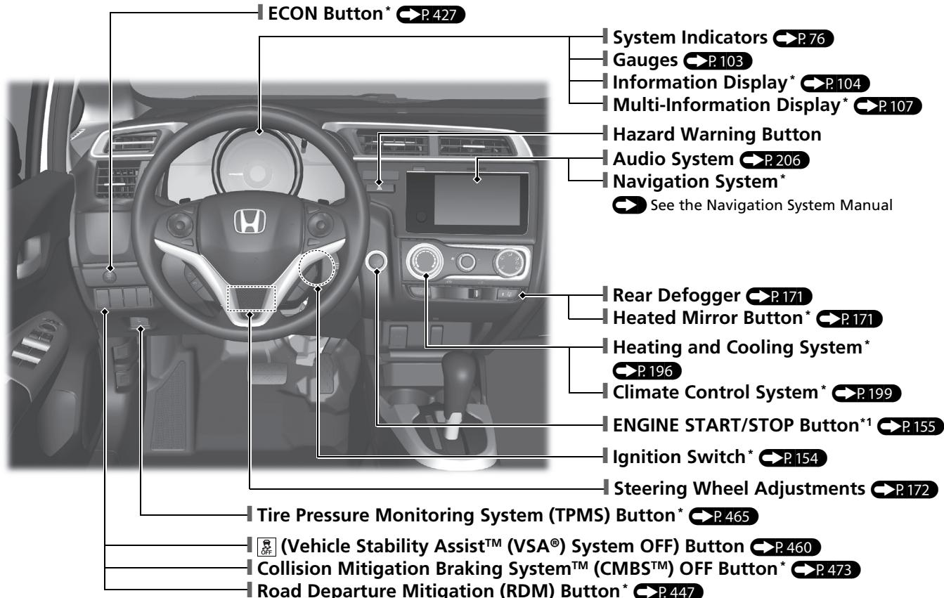
\*1: Models with the smart entry system have an ENGINE START/STOP button instead of an ignition switch.
