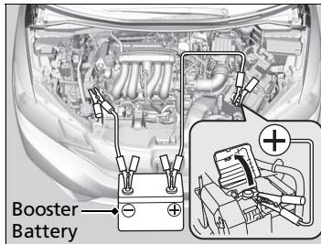
1. Connect the first jumper cable to your vehicle's battery  $\oplus$  terminal.
