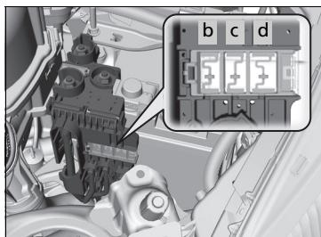
Pull up the cover on the  $\oplus$  terminal, then remove it while pulling out the tab as shown.
