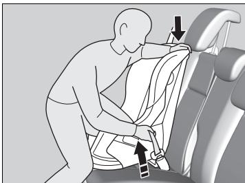
6. Grab the shoulder part of the seat belt near the buckle, and pull up to remove any slack from the lap part of the belt.
