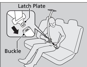
3. Insert the latch plate into the buckle.
