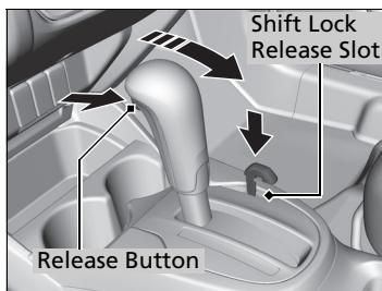
4. Insert the key into the shift lock release slot.
