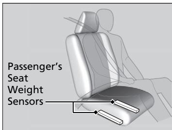
The front passenger's advanced airbag system has weight sensors.
