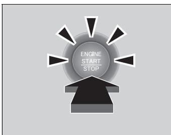
2. Depress the brake pedal (continuously variable transmission) or clutch pedal (manual transmission) and press the **ENGINE START/STOP** button within 10 seconds after the beeper sounds and the **ENGINE START/STOP** button changes from flashing to on.
