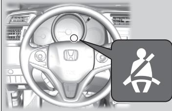
The seat belt system includes an indicator on the instrument panel to remind the driver or a front passenger or both to fasten their seat belts.
