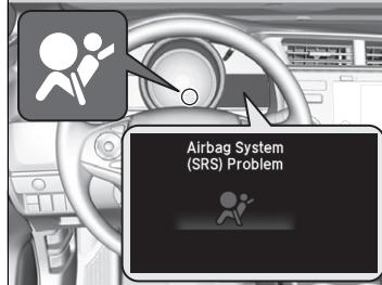
If the indicator comes on at any other time, or does not come on at all, have the system checked by a dealer as soon as possible. If you don't, your airbags and seat belt tensioners may not work properly when they are needed.
