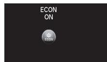
The message is displayed for a few seconds when the ECON button is pressed.
