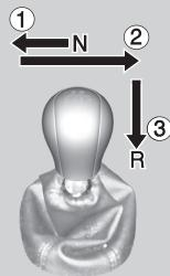
1. Depress the clutch pedal, move the shift lever all the way to the left, and shift to **R**.
